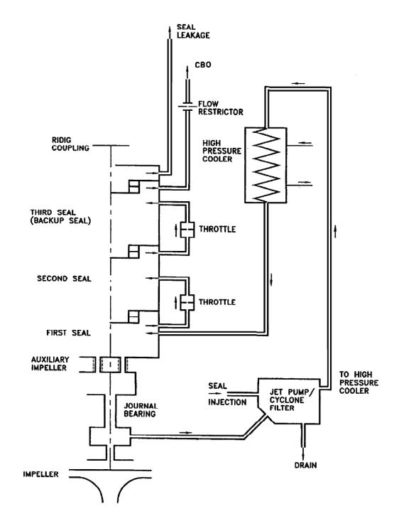
Figure 5.4.1-2 Flow Diagram for Reactor Coolant Pump Shaft Seal System
