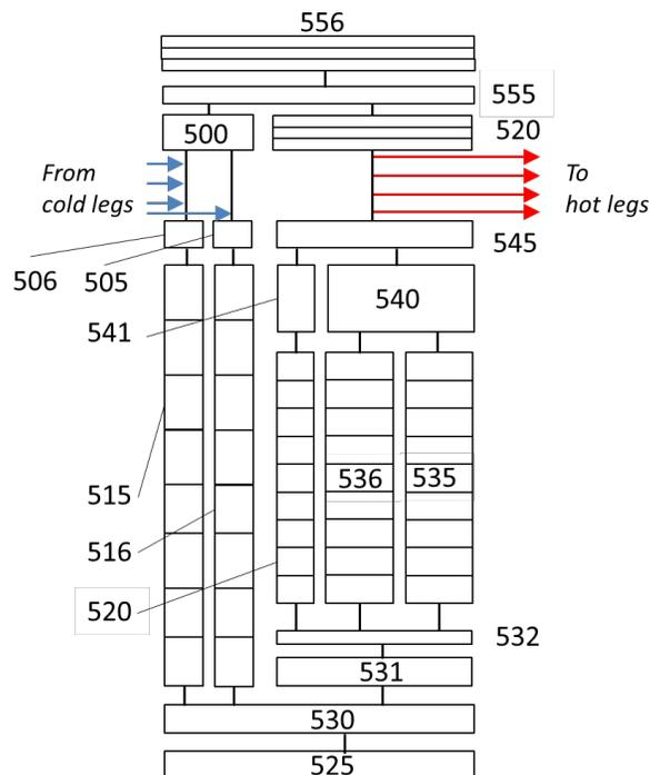
Figure 1 RPV Nodalization Scheme.
