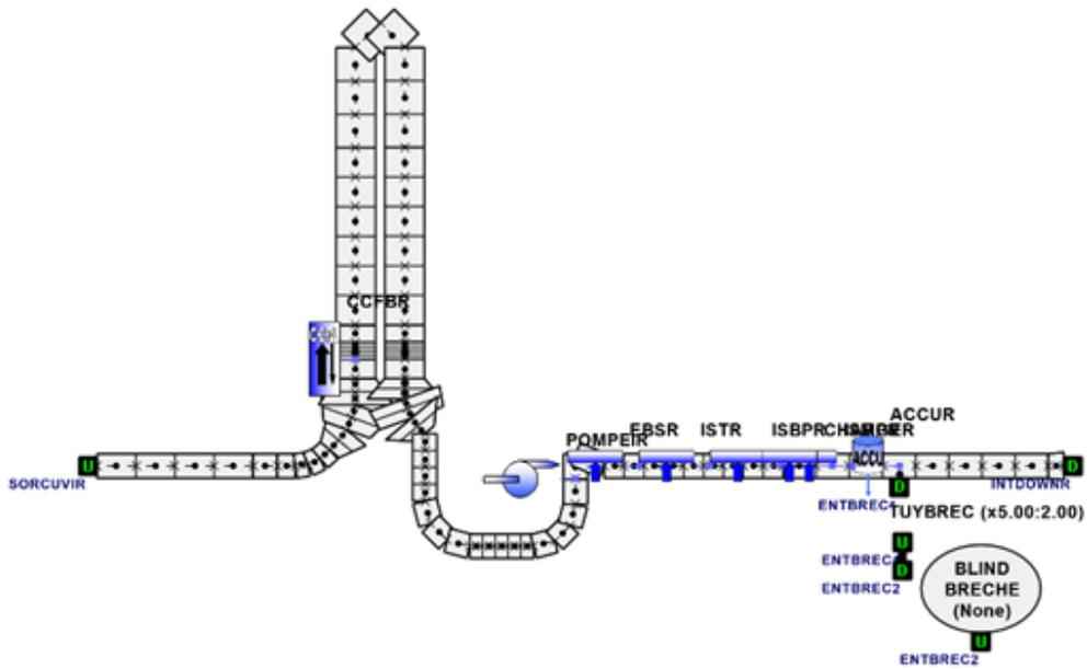
Figure 9 Primary Loop Nodalization Scheme.
