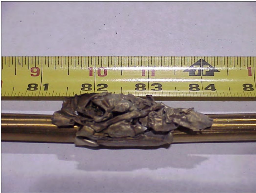
Figure 25. M9-BT-29 Burst Location
