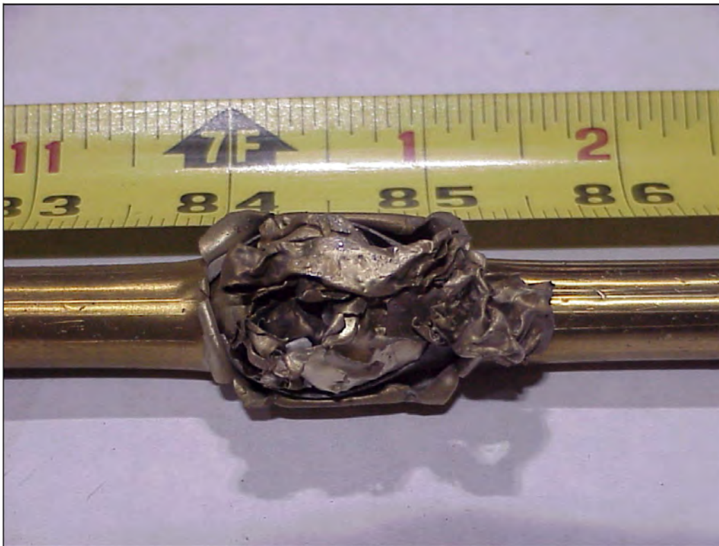
Figure 28. M9-BT-30 Burst Location
