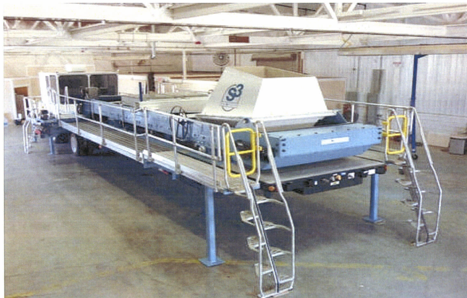
Figure 6-1 Trailer-Mounted S3 Soil Sorting System
