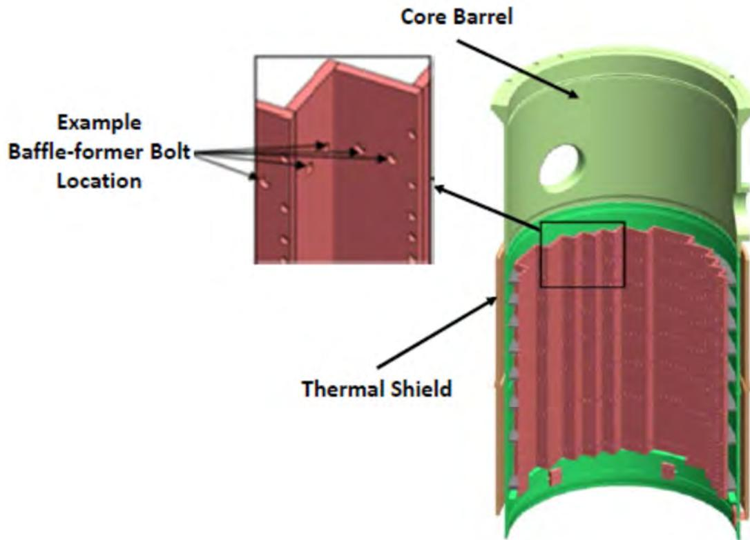
**Figure 2** – Three-dimensional view of a portion of the baffle-former assembly in Westinghouse-design RVI, showing baffle-former bolt locations (reproduced from updated Westinghouse Figures Presented at Public Meeting on MRP-227, Rev. 1, March 31, 2015, ADAMS Accession No. ML15091A136, Ex. NRC000211)
