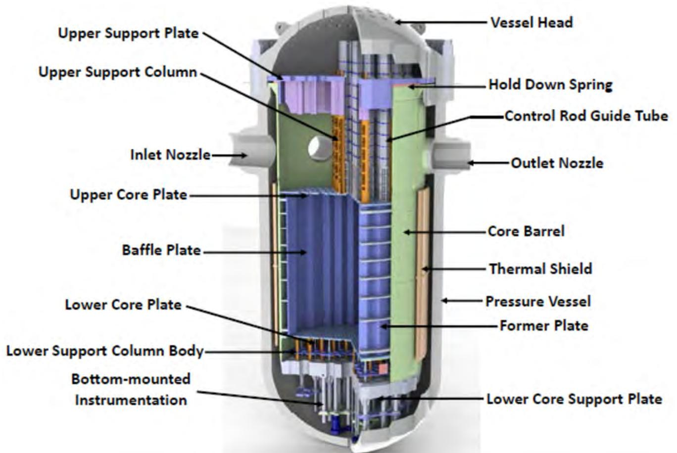
**Figure 1** – Overview of Typical Westinghouse-design Reactor Vessel Internals (reproduced from update Westinghouse Figures Presented at Public Meeting on MRP-227, Rev. 1, March 31, 2015, ADAMS Accession No. ML15091A136 Ex. NRC000211)
