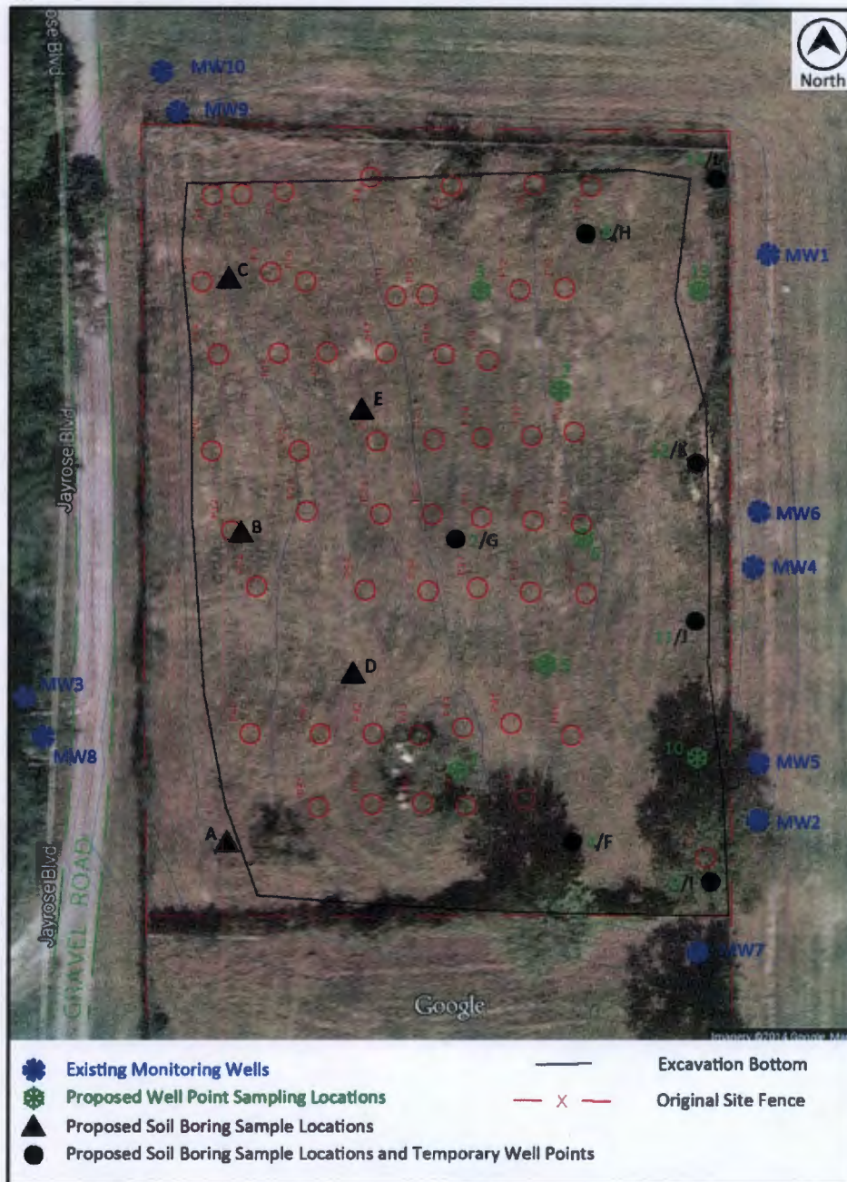
Figure 2 Excavation Sample Locations with Satellite Background Image
