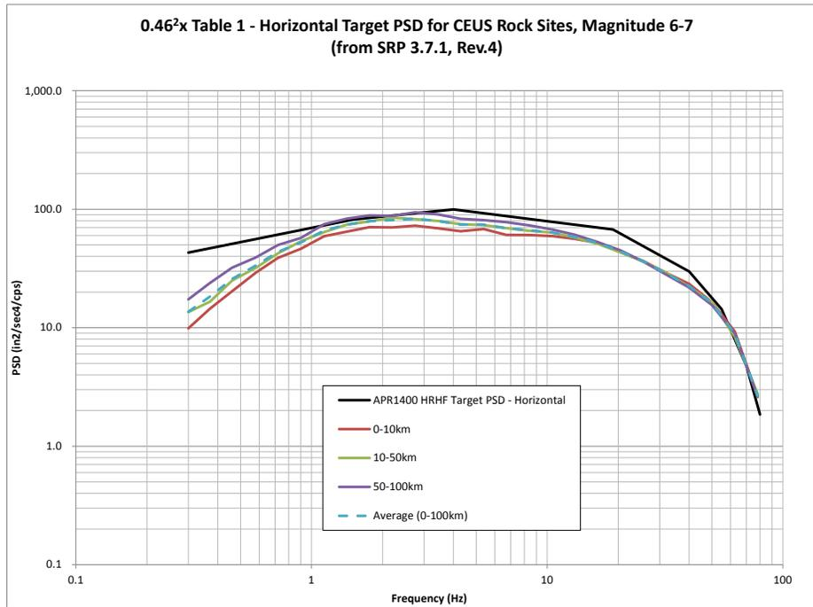
Figure 1 Comparison of the Horizontal Target PSD Compatible with APR1400 HRHF Horizontal Response Spectra with the SRP 3.7.1 PSDs for CEUS Rock Sites
