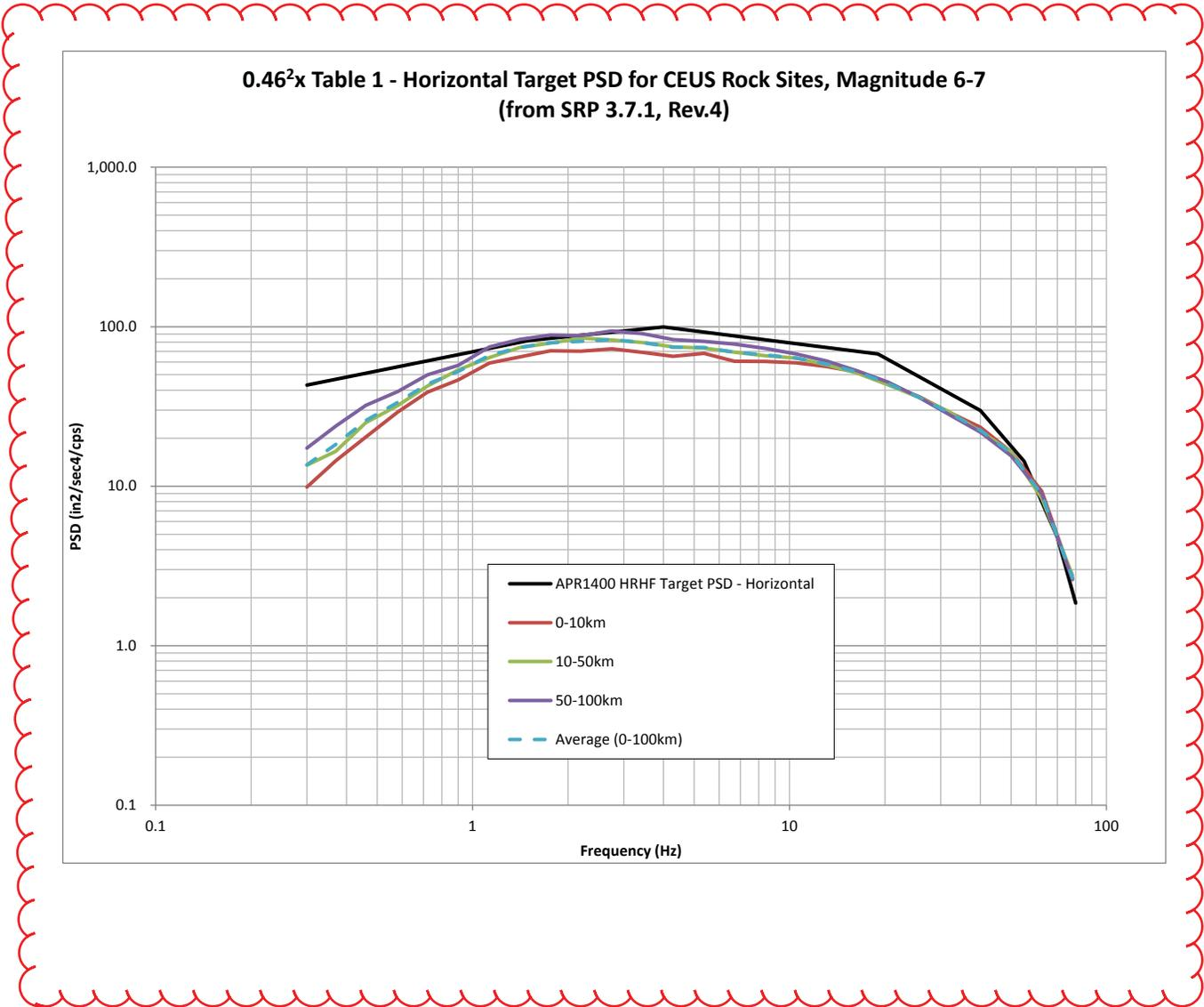
**Figure 3-24 Comparison of the Horizontal Target PSD Compatible with APR1400 HRHF Horizontal Response Spectra with the SRP 3.7.1 PSDs for CEUS Rock Sites**
