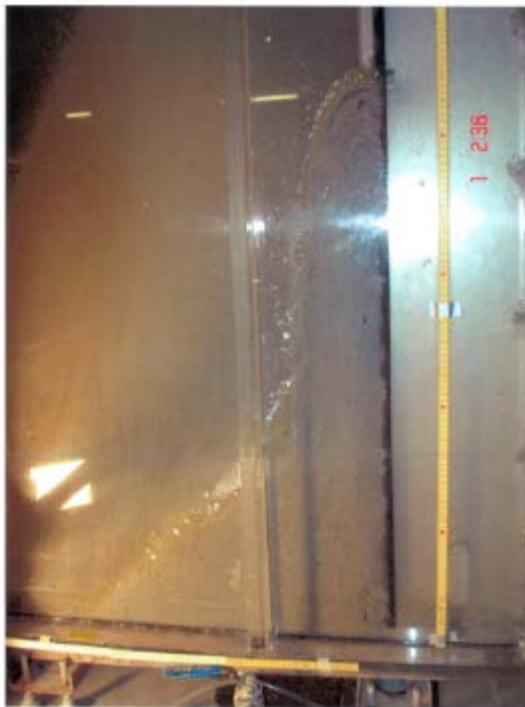
Picture 27: Debris layer without precipitate
