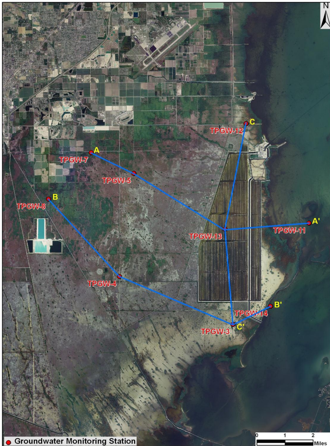
Figure 3.1-7. Locations of Aquifer Cross Sections for Groundwater Chloride Concentrations.
