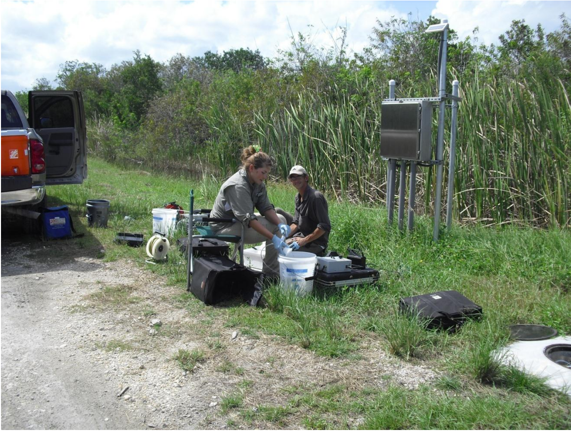
Figure 3.1-1. Typical Groundwater Field Sampling Setup.
