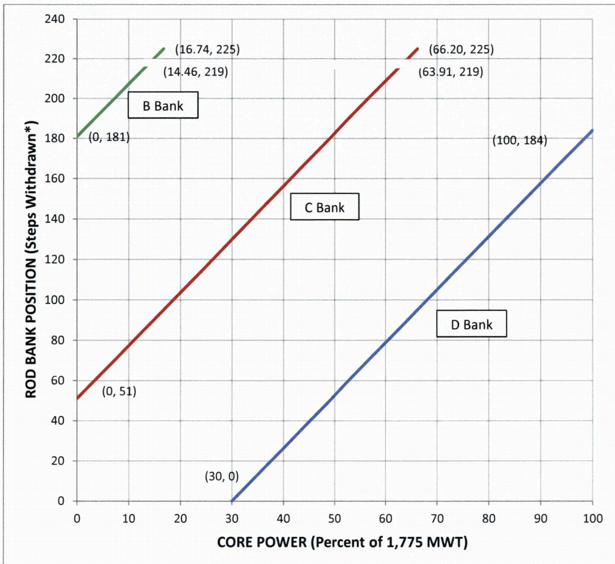
\*The top of the active fuel corresponds to 219. The ARO parking position may be any position above the corresponding top of active fuel for each respective bank. The control rod tip-to-tip distance is defined as 130 steps while rods are moving in overlap. The bank positions are given as follows:
