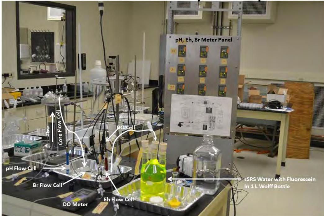
**Figure 3-1. Flow Loop Apparatus Used for Core 11, Middle Section Closed-Loop Aerated Test**
