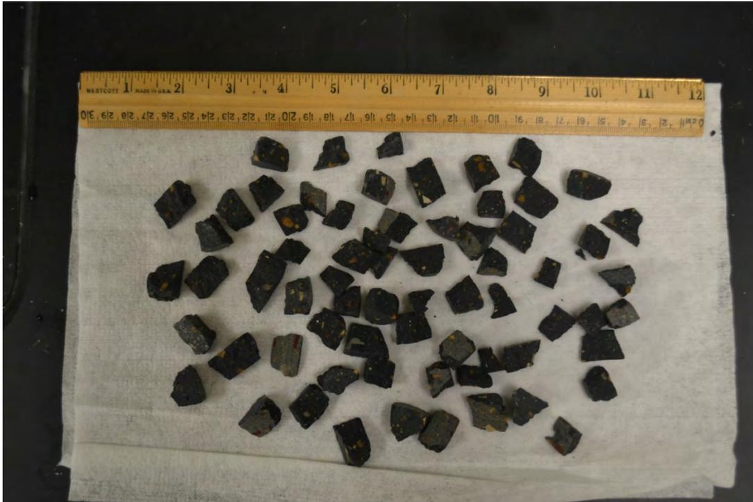
**Figure 4-5. Chips of Core 10 Used in July 30–August 3, 2015 Static Test**
