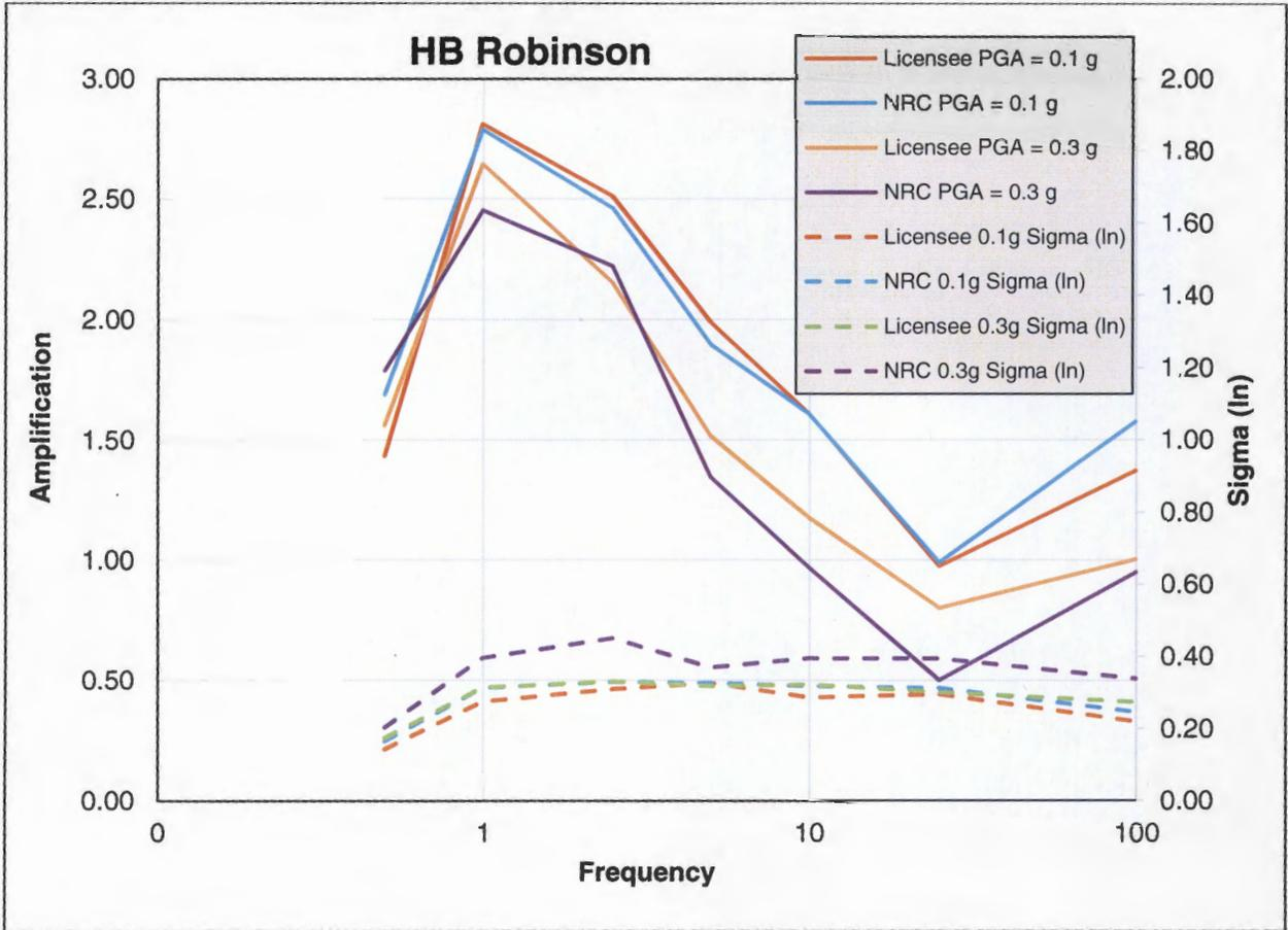
Figure 3.3-3 Plot Comparing the Staff's and the Licensee's Mean Control Point Hazard Curves at a Variety of Frequencies for the Robinson site.
