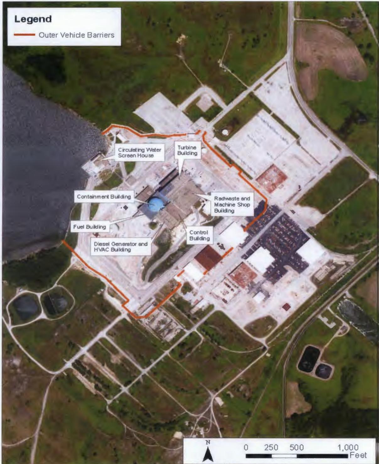
Figure 3.1-2 Clinton Power Station Site Layout (derived from Exelon, 2014)
