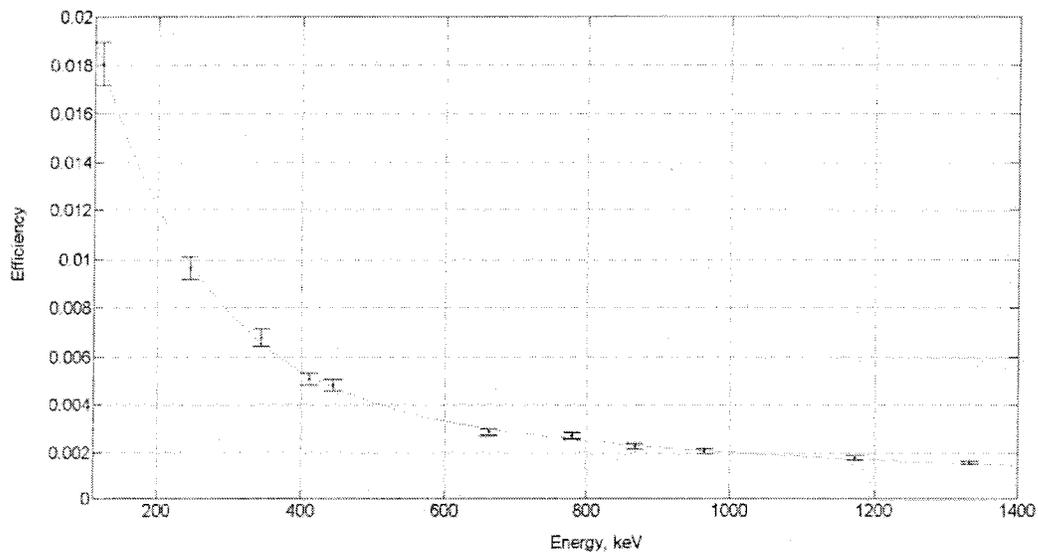
Figure 2. Efficiency curve for Niowave's HPGe detector.
