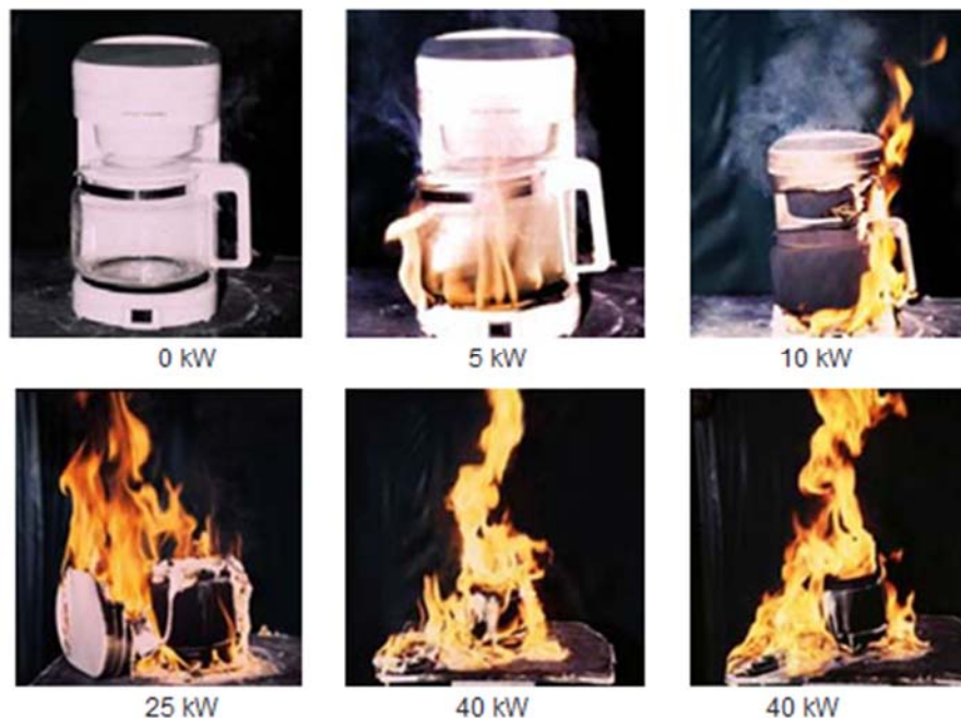
Figure 2-1 Fire Size/Intensity Calibration (0 to 40 kW)
