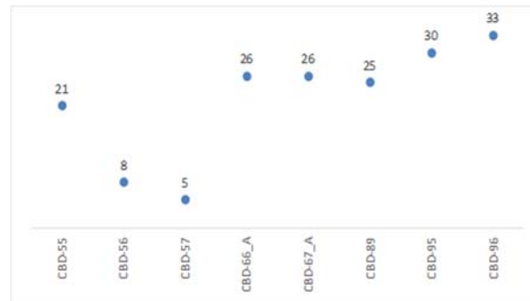
Figure D-15 Control Large Closed TP-Very Low. Values above round markers list the test heat release rate value in units of kW.
