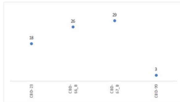
Figure D-20 Control Large Open TP-Low. Values above round markers list the test heat release rate value in units of kW.
