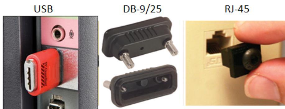
Figure 4.4 – Physical barrier (port-lock) devices used to block port access
