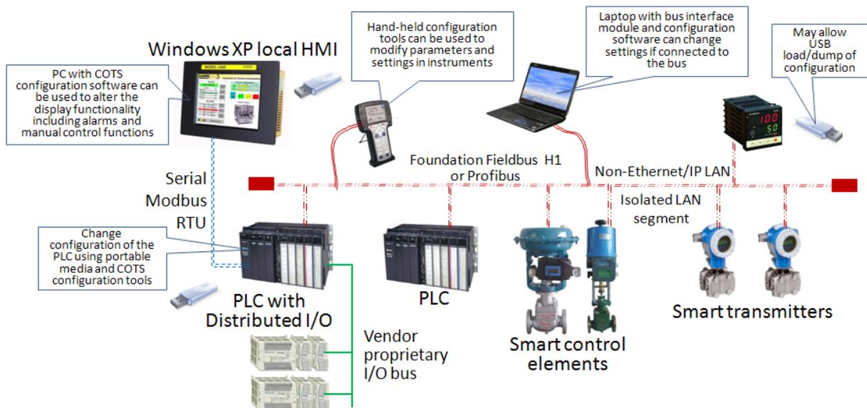
Figure 10.1 – An instrument bus can connect a range of smart devices
