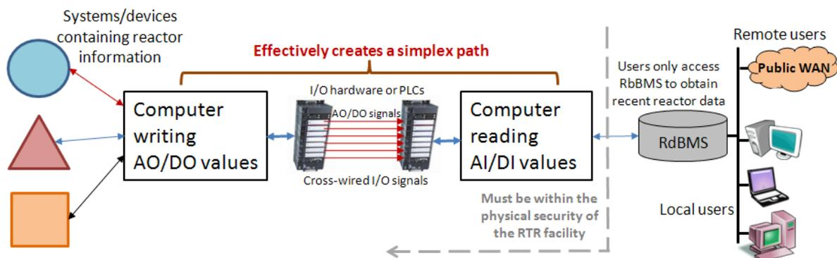
Figure 6.13 – Using analog and contact I/O for unidirectional data transfers
