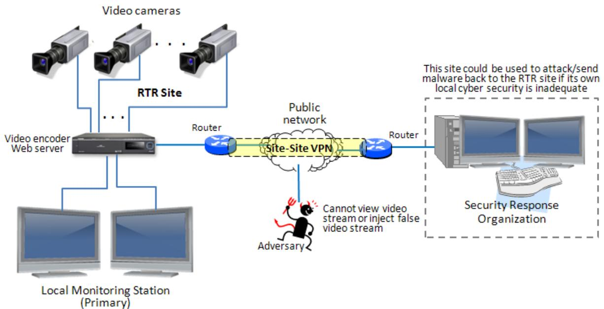
Figure 6.7 – Creating a site-to-site VPN using routers to encrypt video stream
