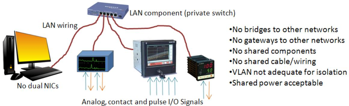
Figure 6.8 – Example of a small isolated LAN containing multiple CDAs
