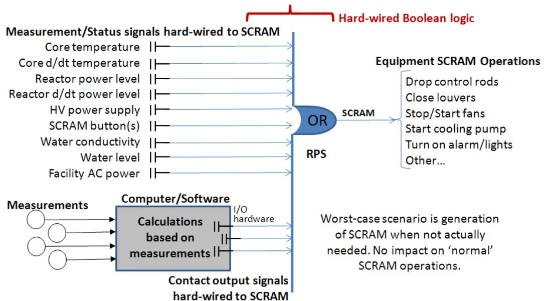
Figure 11.6 – Adding computed trip signals to the reactor SCRAM logic
