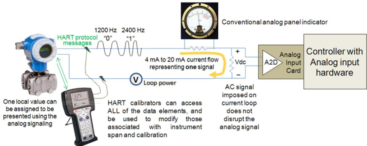
Figure 10.2 – A HART-compliant transmitter operating in analog mode
