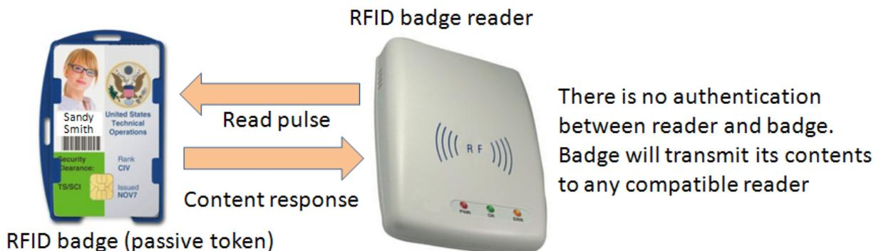
Figure 4.3 – RFID badge (passive token device) and compatible badge reader
