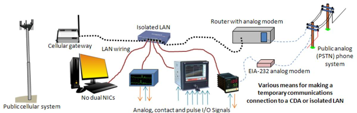
Figure 7.3 – Establishing direct remote access to CDAs and isolated LANs
