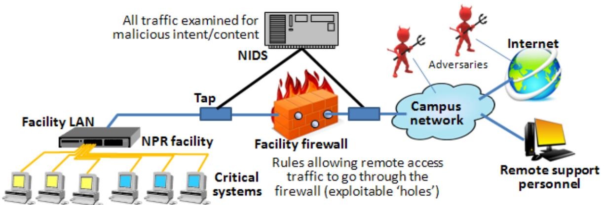
Figure 6.15 – Installing a NIDS to inspect all NPR facility message traffic
