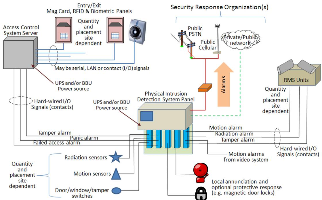
Figure 4.7 – Simplified block diagram of typical integrated (interconnected) access monitoring, control and alarm systems at licensee facilities
