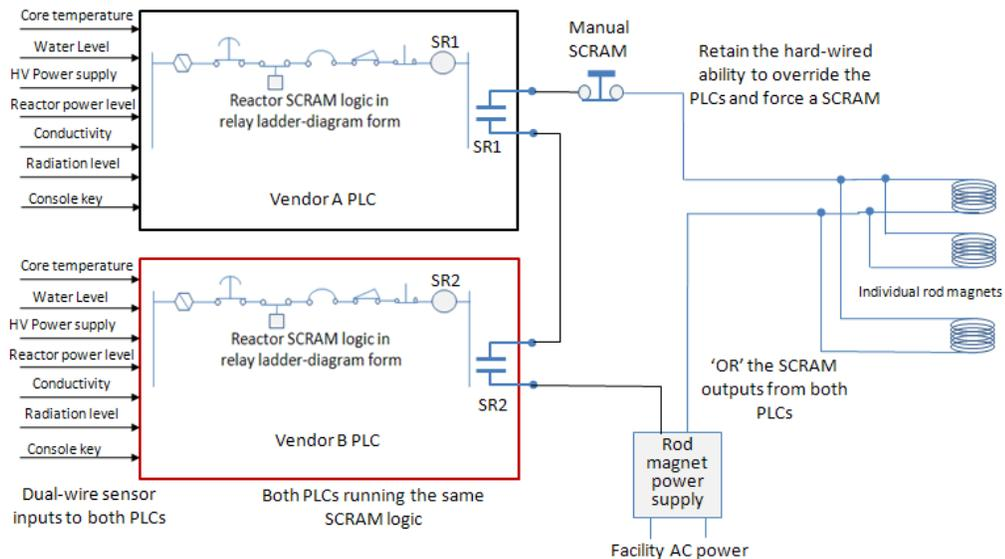
Figure 11.7 – Redundant PLCs used for a reactor safety system
