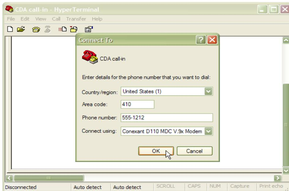
Figure 7.4 – Establishing a dial-up telephone connection via the PSTN
