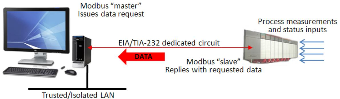
Figure 6.6 – Dedicated, low-speed, serial communications circuit using Modbus
