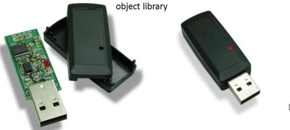
Figure 9.2 – Programmable USB “dongle” with integral microcontroller
