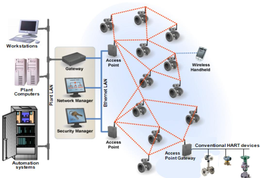
Figure 10.3 – A typical instrumentation WLAN based on WirelessHART
