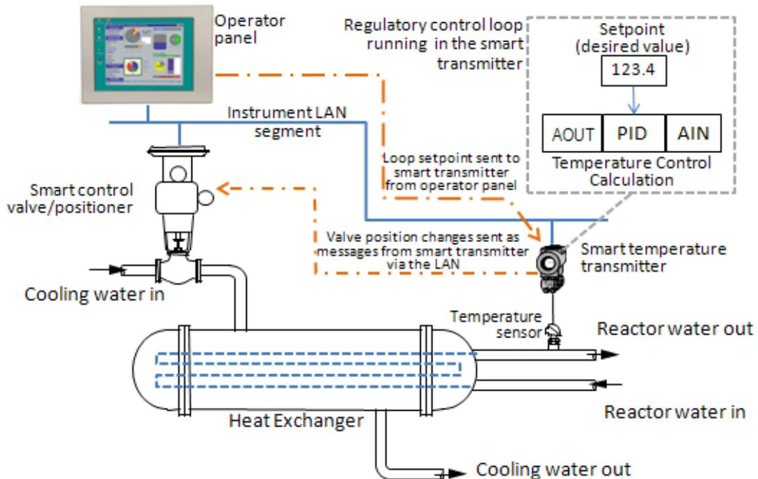
Figure 10.6 – Autonomous regulatory control using smart instruments
