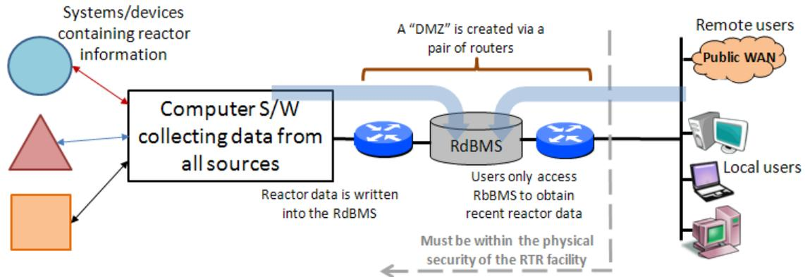
Figure 6.12 – Creating a DMZ and shared data server to isolate networks
