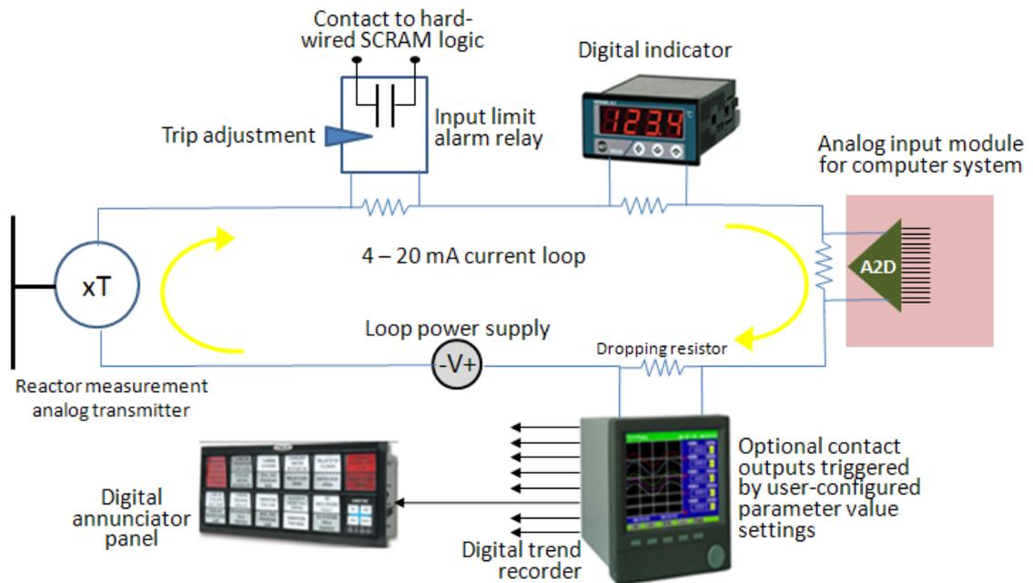
Figure 11.1 – Digital I&C devices integrated into ‘analog’ circuits
