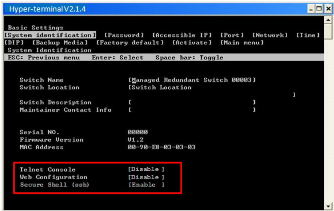
Figure 7.1 - Default network settings configured via the CDA's console port
