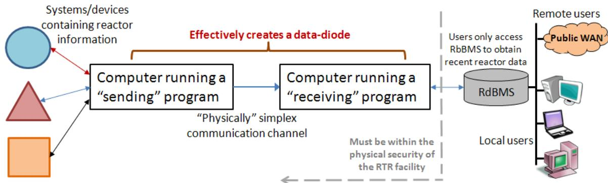
Figure 6.11 – Creating a one-way data flow using a data-diode
