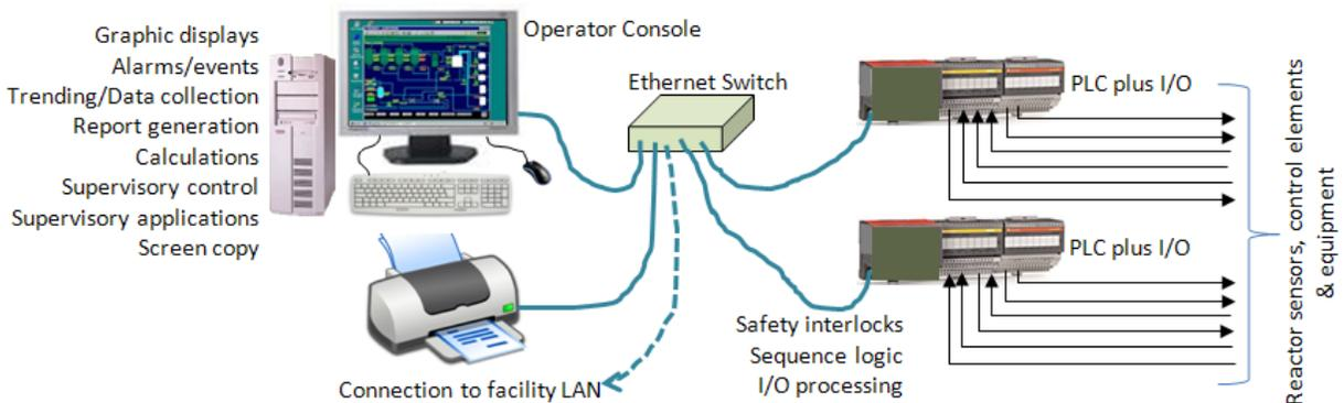
Figure 11.10 – Potential future digital reactor control system architecture
