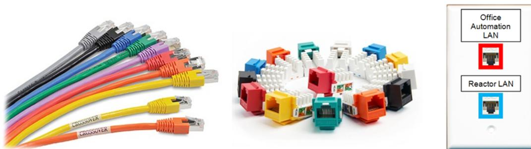
Figure 6.5 – Examples of the color variations available for Ethernet LANs
