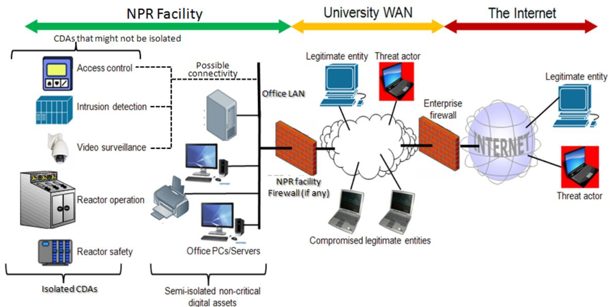
Figure 6.1 – General block diagram of a typical NPR facility network architecture
