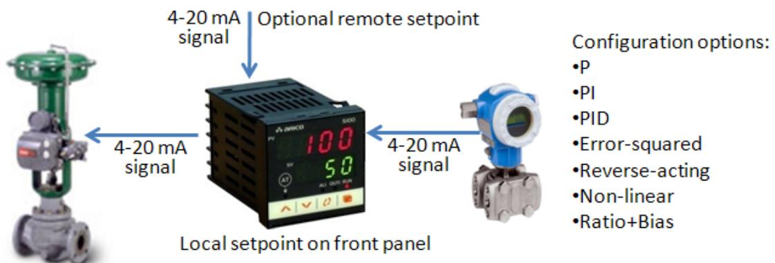
Figure 11.4 – A digital PID controller with a password-protected configuration
