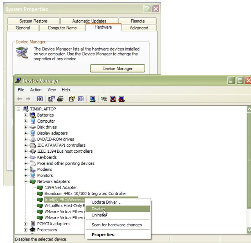
Figure 6.10 – Disabling/Enabling a wireless adapter under Windows XP®
