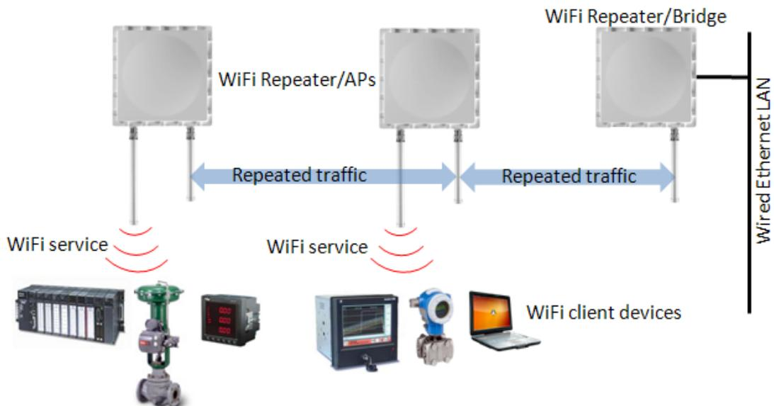
Figure 10.5 – Wireless Ethernet repeaters and access points
