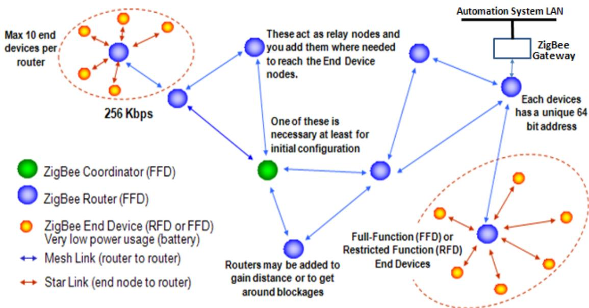
Figure 10.4 – The ZigBee wireless mesh architecture
