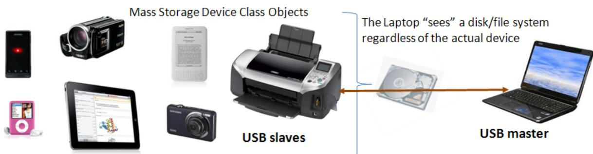
Figure 9.3 – Digital devices supporting USB accessible file systems
