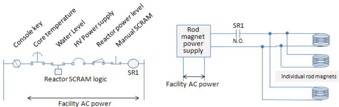
Figure 11.5 – Simplified reactor fail-safe SCRAM design concept
