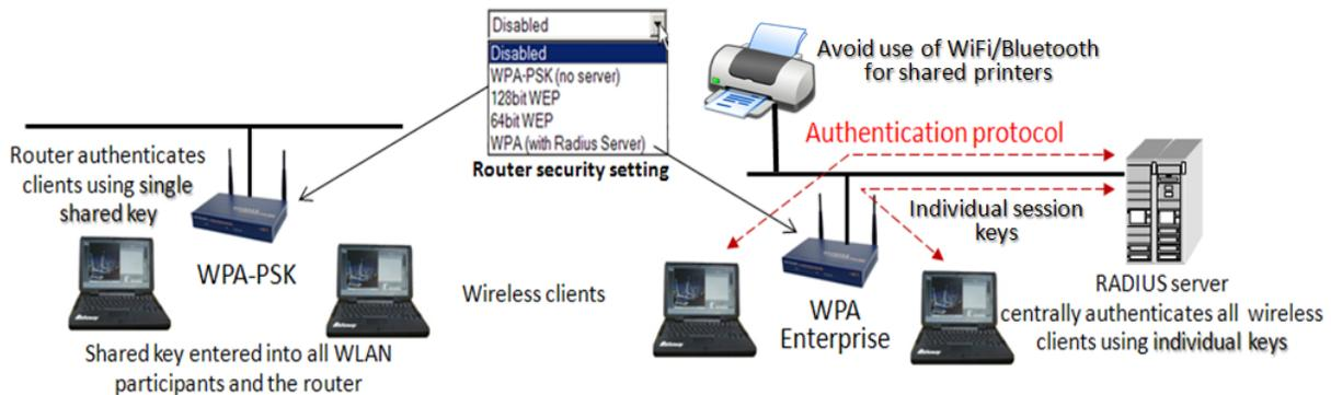
Figure 6.9 – Using WPA-PSK and WPA-Enterprise for wireless networking
