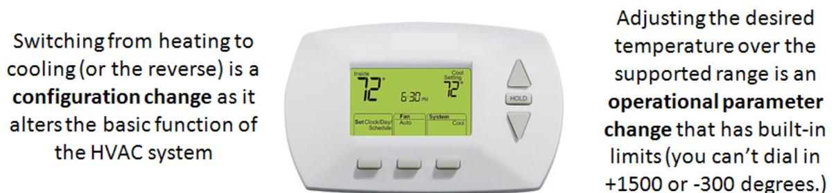
Figure 11.3 – The difference between configuration and operational settings
