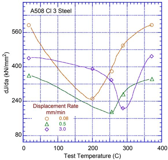
Figure 82. Dependence of crack growth resistance  $dJ/da$  on loading displacement rate and temperature for A508 Cl 3 pressure vessel steel (Ref. 165).
