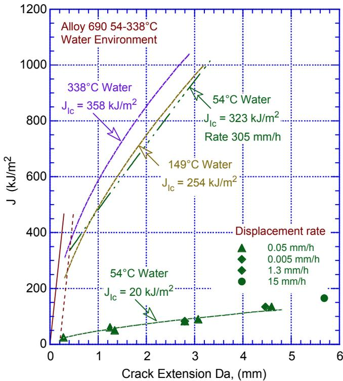
Figure 98. J-R curves for Alloy 690 in a water environment at a temperature of 54°C and displacement rates of 0.005 to 305 mm/h. The J-R curves at 149 and 338°C obtained under quasi-static conditions are shown for comparison (Ref. 241).
