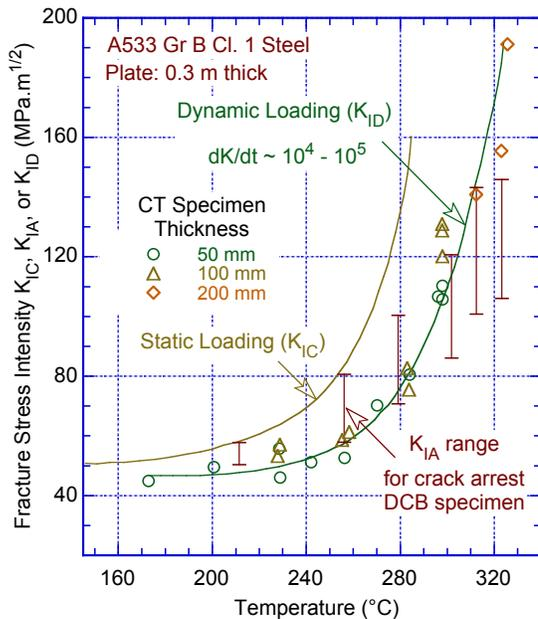
Figure 86. Temperature dependence of static  $K_{IC}$ , dynamic  $K_{ID}$ , and crack arrest  $K_{IA}$  fracture toughness measurements for A533 Gr B steel (Ref. 227 as adapted by 228).
