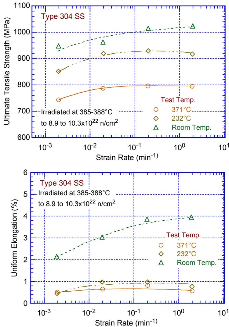
Figure 48. Effect of strain rate on the tensile properties of solution-annealed Type 304 stainless steel irradiated at 385-388°C in EBR-II to fluences of 8.8 to 10.3 x 10<sup>22</sup> n/cm<sup>2</sup> and tested at RT, 232, and 371°C (450 and 700°F) (Ref. 42).
