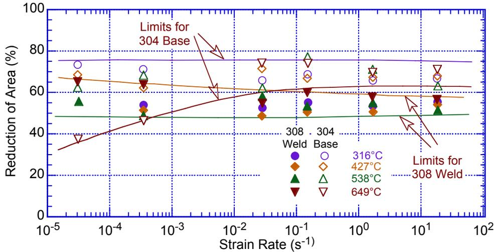
Figure 64. Effect of strain rate on the elevated-temperature reduction of area for Type 308 SS weld metal and Type 304 SS base metal (Ref. 177).
