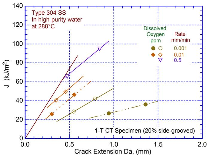
Figure 93. Crack resistance behavior of sensitized Type 304 SS at  $288^\circ\text{C}$  in simulated BWR coolant with two dissolved oxygen levels at three different displacement rates (Ref. 234).
