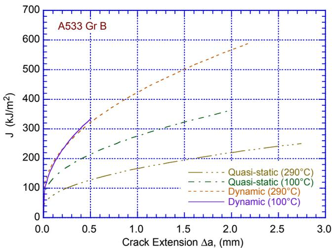
Figure 84. Crack resistance behavior for the JSPS special heat of A533 Gr B steel at 25 and 290°C under both quasi-static and dynamic loading conditions (Ref. 176).
