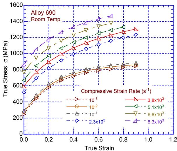
Figure 68. Room-temperature true stress-true strain curves for Alloy 690 obtained at various strain rates under compressive loading (Ref. 210).
