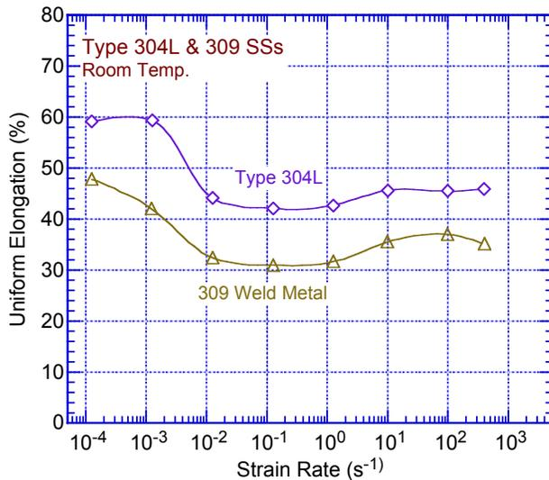
Figure 50. Variation of uniform elongation with strain rate for Types 304L and 309 SSs (Ref. 192).
