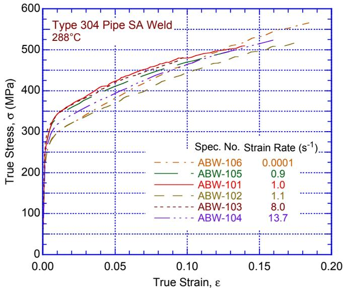
Figure 65. True stress-true strain curves at 288°C (550°F) for a SA weld in a Type 304 SS pipe at several different strain rates (Ref. 182).
