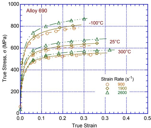
Figure 70. Shear stress-strain curves of Alloy 690 deformed at different strain rates and temperatures (Refs. 213,214).
