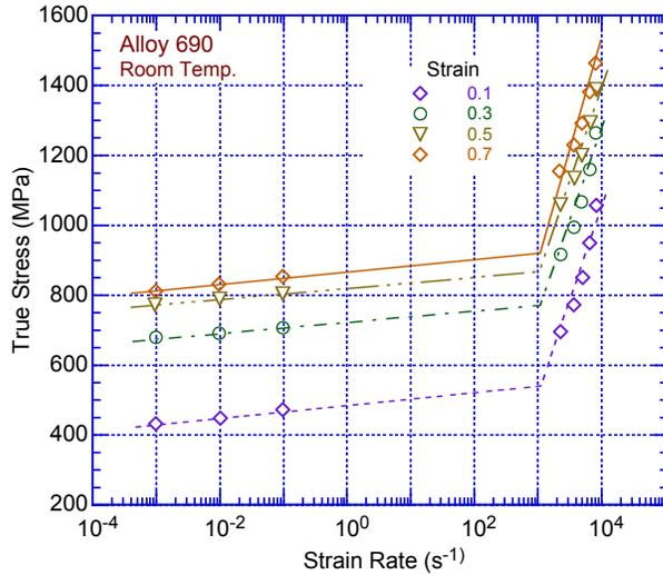
Figure 69. Room-temperature dependence of flow stress at various strains on strain rate for Alloy 690 under compressive loading (Ref. 211).
