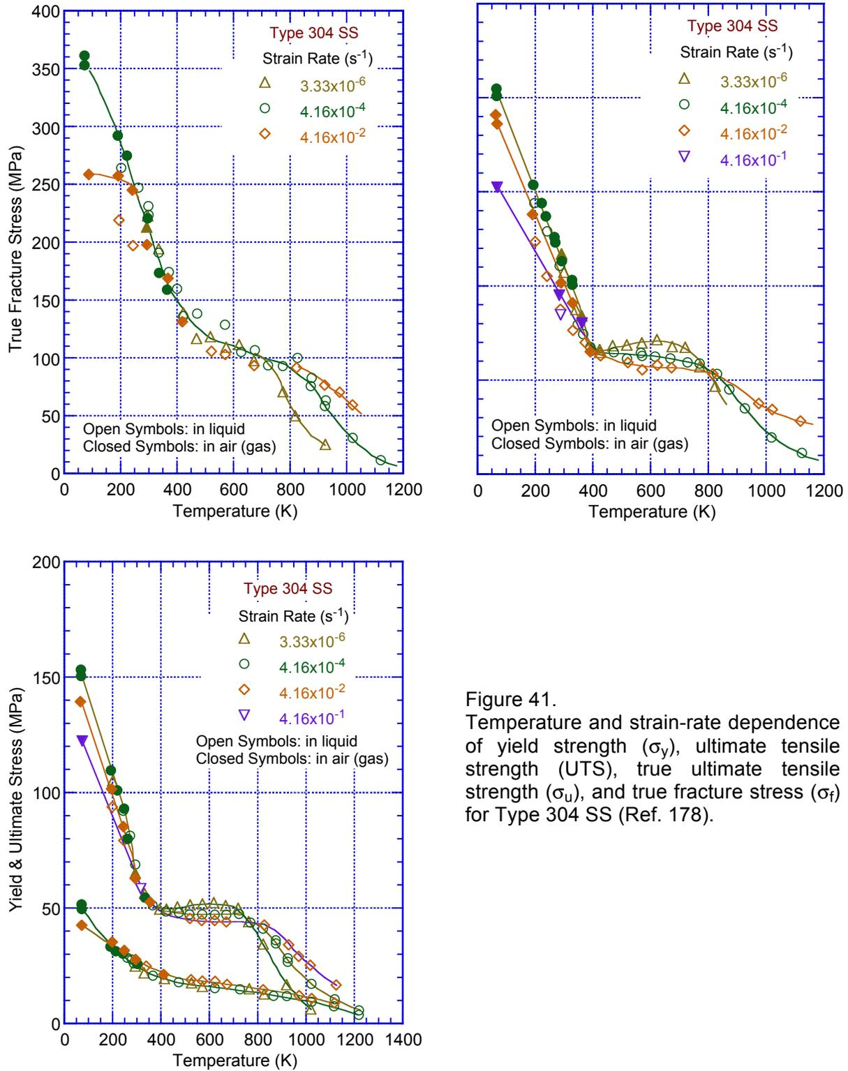
Figure 41. Temperature and strain-rate dependence of yield strength ( $\sigma_y$ ), ultimate tensile strength (UTS), true ultimate tensile strength ( $\sigma_u$ ), and true fracture stress ( $\sigma_f$ ) for Type 304 SS (Ref. 178).
