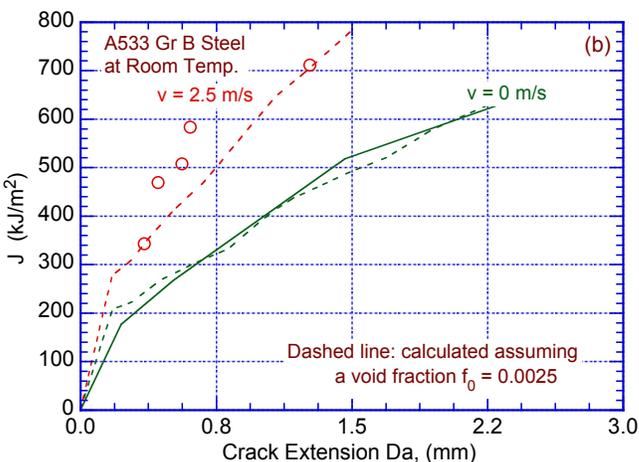
Figure 88. Crack resistance behavior for two different heats of A533 Gr B pressure vessel steel at room temperature under both quasi-static and dynamic loading conditions. (a) shows the data of Wallin et al. (Ref. 231), and (b) shows the data of Joyce (Ref. 232). The dashed curves are calculated assuming a given void volume fraction  $f_0$  in the material that leads to ductile fracture (Ref. 230).
