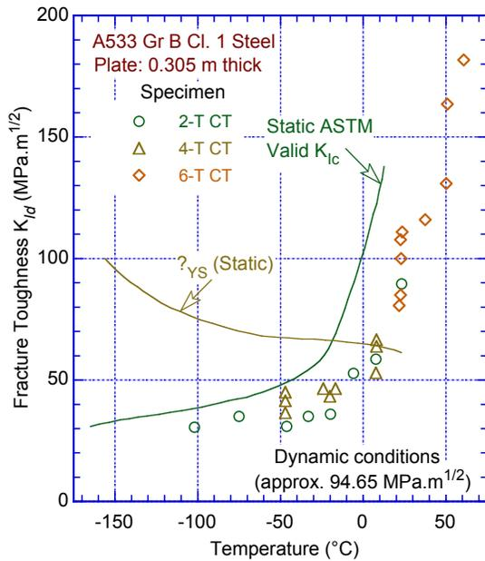
Figure 85. Fracture toughness versus temperature behavior for A533 Gr B steel under both static (solid line) and dynamic ( $dK/dt$  of approx.  $104 \text{ ksi}\cdot\text{in}^{1/2}$ ) conditions (data points) (Ref. 225, 226 as reproduced in 224).
