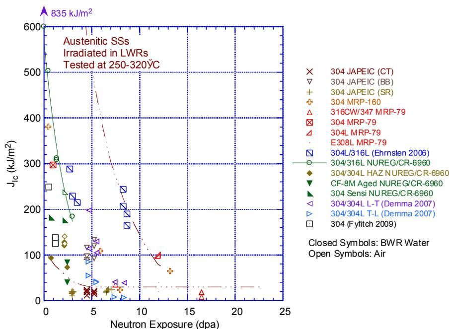
Figure 89. Change in fracture toughness,  $J_{Ic}$ , as a function of neutron exposure for irradiated austenitic SSs. Dashed lines represent the scatter band for the fast reactor data on austenitic SSs irradiated at 350–450°C (662–843°F) (Ref. 39,42–44,47-52).
