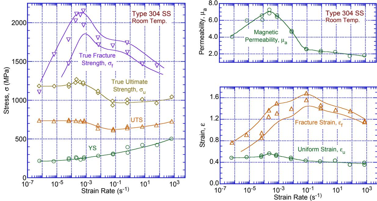
Figure 43. Variation of tensile and magnetic properties of Type 304 SS with strain rate at room temperature: (a) yield strength [ $\sigma_y$ ], ultimate tensile strength [UTS], true ultimate tensile strength [ $\sigma_u$ ], and true fracture strength [ $\sigma_f$ ]; (b) uniform strain [ $\epsilon_u$ ], true fracture strain [ $\epsilon_f$ ], and apparent magnetic permeability at  $\epsilon_u$  [ $\mu_a$ ] (Refs. 180,181).
