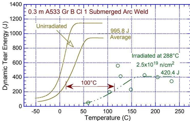
Figure 75. Charpy-V (Cv) and dynamic tear test data for a 0.3 m-thick A533 Gr B CI 1 SA weld deposit before and after 550°F (288°C) irradiation. Specimens were taken between the quarter- and half-thickness locations with their long dimension perpendicular to the welding direction. (Ref. 217).
