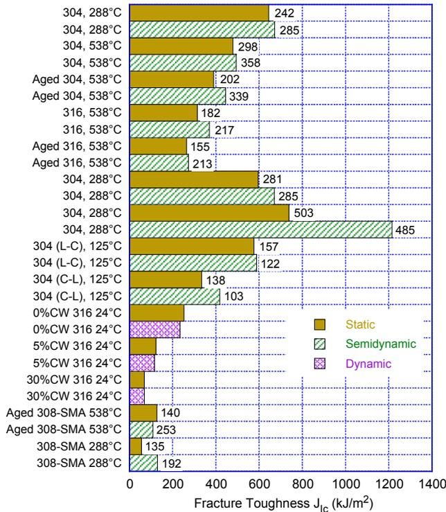
Figure 94. Effect of strain rate on  $J_{Ic}$  and  $dJ/da$  (values of the latter parameter are given next to each bar in MPa) for Types 304 and 316 SSs and Type 308 SS weld metal under various conditions (Ref. 41).
