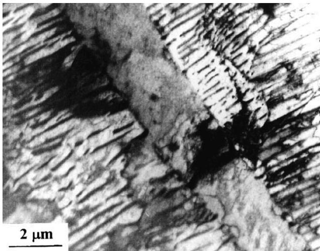
Figure 18. Typical microstructure in A106–Gr B specimen tested at an 0.4 %/s strain rate showing immature dislocation walls in three pearlite grains consisting of  $\text{Fe}_3\text{C}$  plates in the ferrite matrix (Ref. 124).
