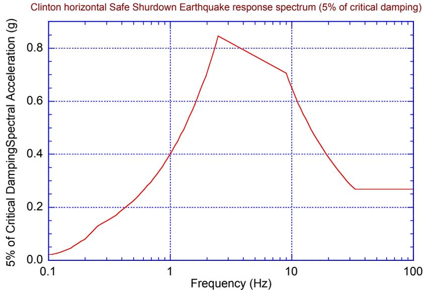
Figure 10. Horizontal SSE response spectrum with 5% critical damping.
