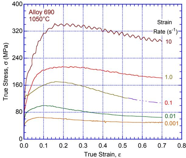
Figure 71. True stress-true strain curves for Alloy 690 obtained from hot compression tests at 1050°C (Ref. 215).
