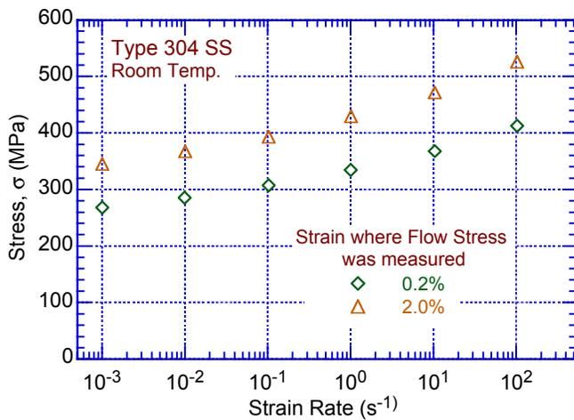
Figure 45. Variation of room-temperature tensile flow stress at 0.2 and 2.0% strain with strain rate for Type 304 SS (Ref. 183).
