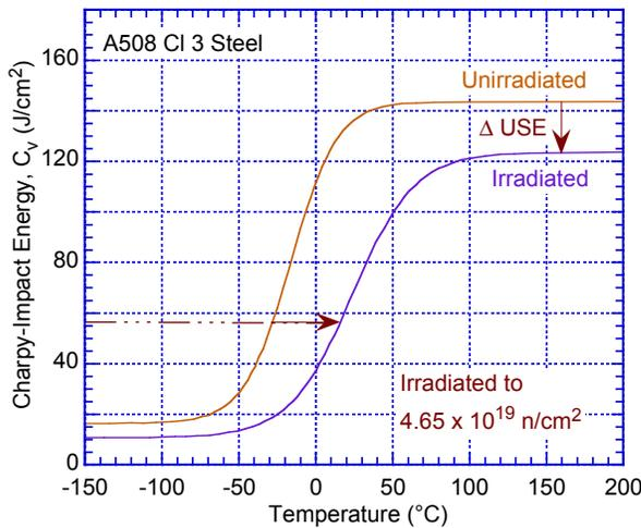
Figure 73. Charpy V-notch fracture toughness transition curves for A508 Cl 3 steel specimens in the unirradiated condition and after irradiation to a fluence of  $4.65 \times 10^{19} \text{ n/cm}^2$  (>1 MeV) (Ref. 216).
