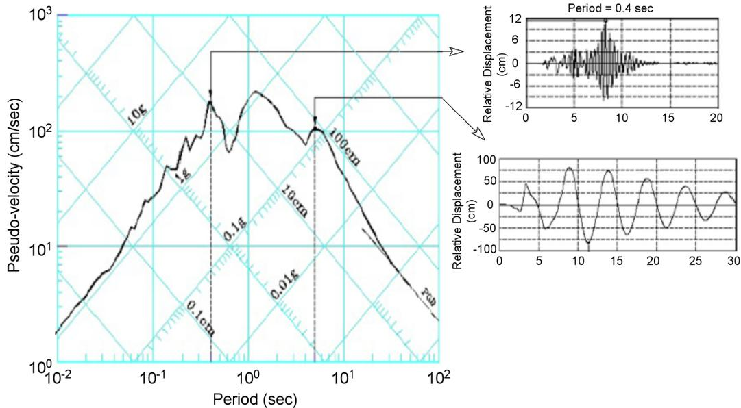
Figure 4. Site-specific ground motion response spectrum (Ref. 95).
