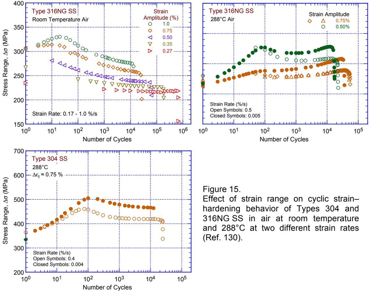
Figure 15. Effect of strain range on cyclic strain-hardening behavior of Types 304 and 316NG SS in air at room temperature and 288°C at two different strain rates (Ref. 130).
