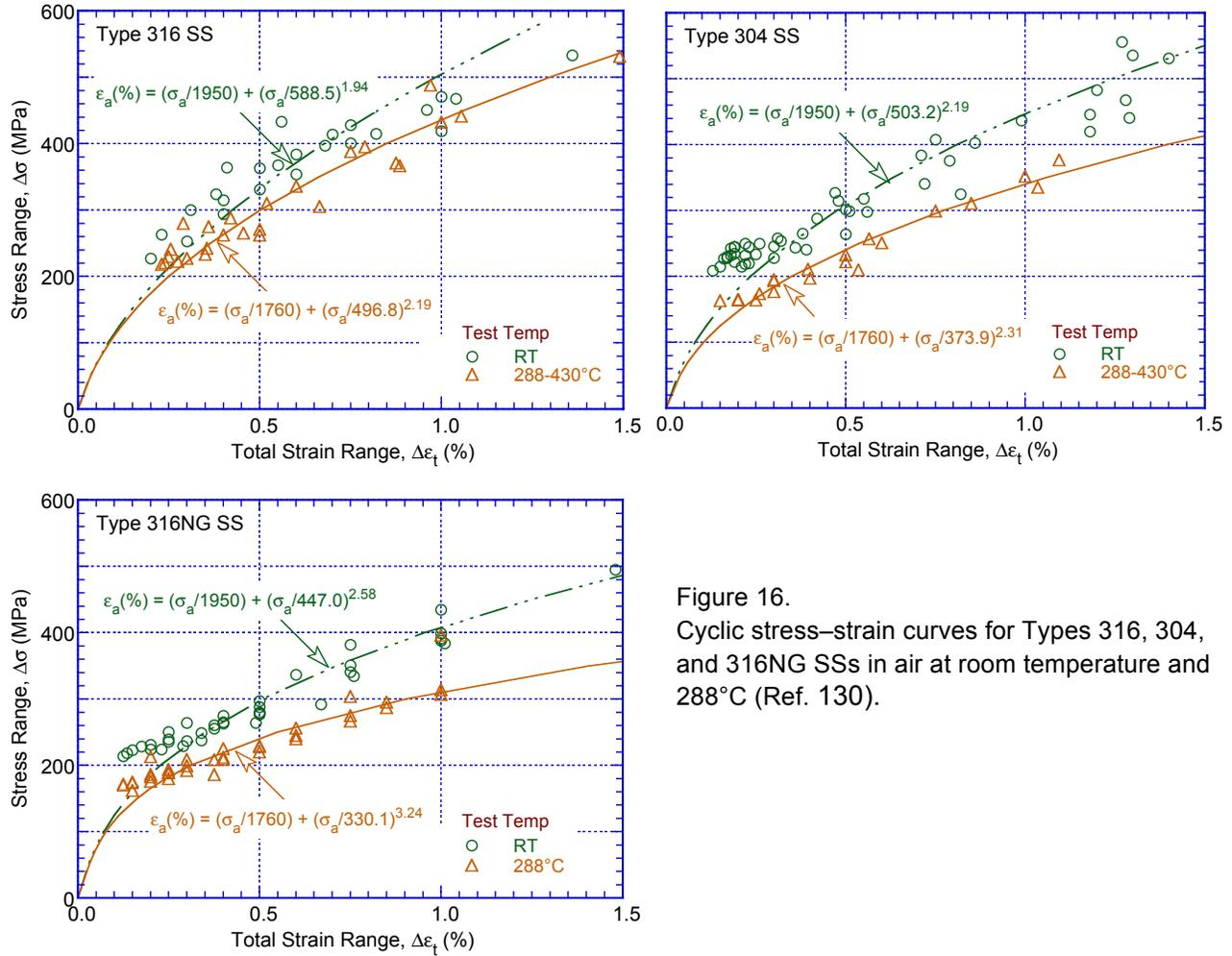
Figure 16. Cyclic stress–strain curves for Types 316, 304, and 316NG SSs in air at room temperature and 288°C (Ref. 130).
