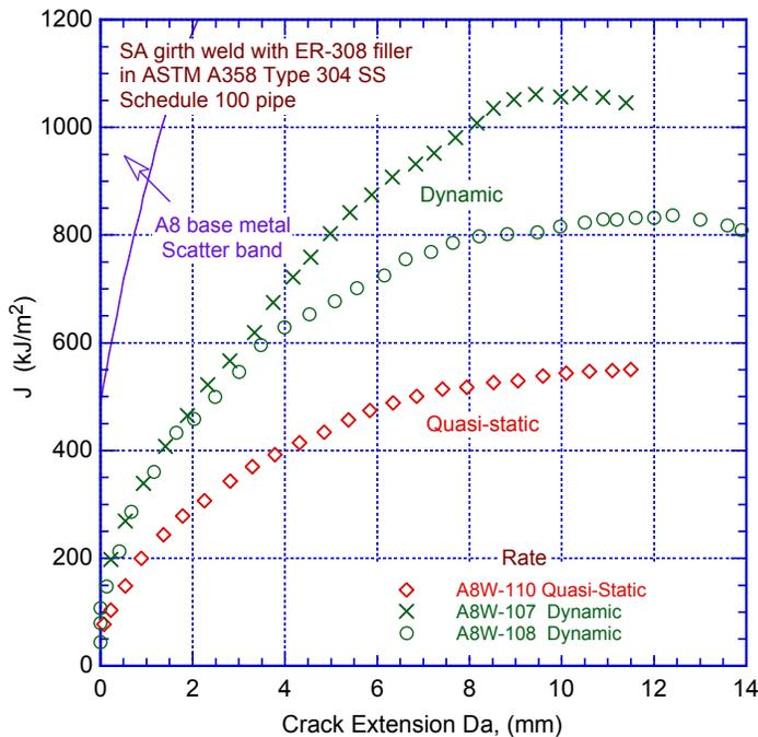
Figure 92. Crack resistance behavior for an SA girth weld specimen from an A358, Type 304 SS 406-mm (16-in.) diameter, Schedule 100 pipe with ER-308 filler metal (Ref. 233).
