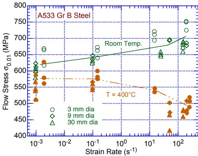
Figure 40. Variation of ultimate tensile strength of A533 Gr B pressure vessel steel with strain rate for three specimen sizes and two temperatures (Ref. 175).
