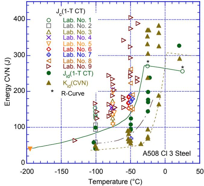
Figure 80. Fracture toughness versus temperature behavior for A508 Cl 3 steel. The three curves, from left to right, represent fits to data generated at strain rates of 1.6 MPa.m<sup>1/2</sup>/s [static 1T-CT tests), 1.4 x 10<sup>4</sup> MPa.m<sup>1/2</sup>/s (dynamic 1T-CT tests), and 6.5 x 10<sup>5</sup> MPa.m<sup>1/2</sup>/s (instrumented Charpy tests), respectively (Ref. 223).
