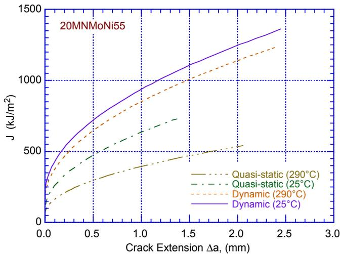
Figure 83. Crack resistance behavior for the German 20MnMoNi55 steel at 25 and 290°C under both quasi-static and dynamic loading conditions (Ref. 176).
