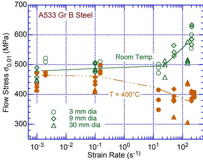
Figure 39. Variation of yield strength (flow stress at a strain of 0.01) for A533 Gr B pressure vessel steel with strain rate for three specimen sizes and two temperatures (Ref. 175).
