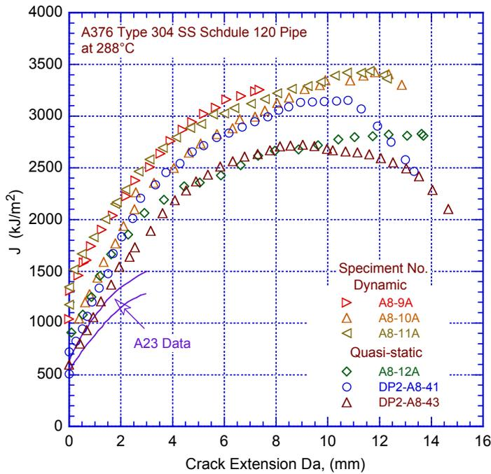
Figure 91. Crack resistance behavior for A376, Type 304 SS Schedule 120 piping material at 288°C under both quasi-static and dynamic loading conditions (Ref. 233).
