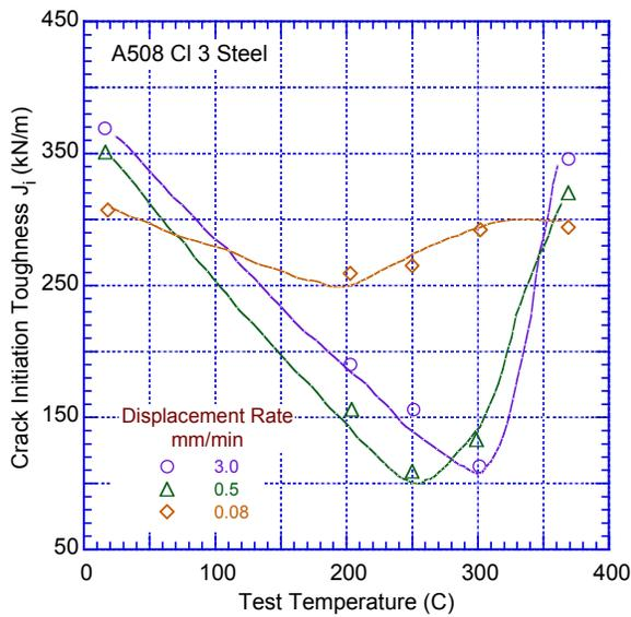
Figure 81. Dependence of crack initiation toughness  $J_{ic}$  on loading displacement rate and temperature for A508 Cl 3 pressure vessel steel (Ref. 165).
