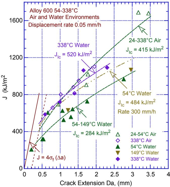
Figure 97. J-R curves for Alloy 600 in air and water at temperatures of 54 to 338°C. All data were obtained under quasi-static loading conditions (displacement rate = 0.05 mm/h) except for the dashed curve, which represents results obtained at 300 mm/h (Ref. 240).
