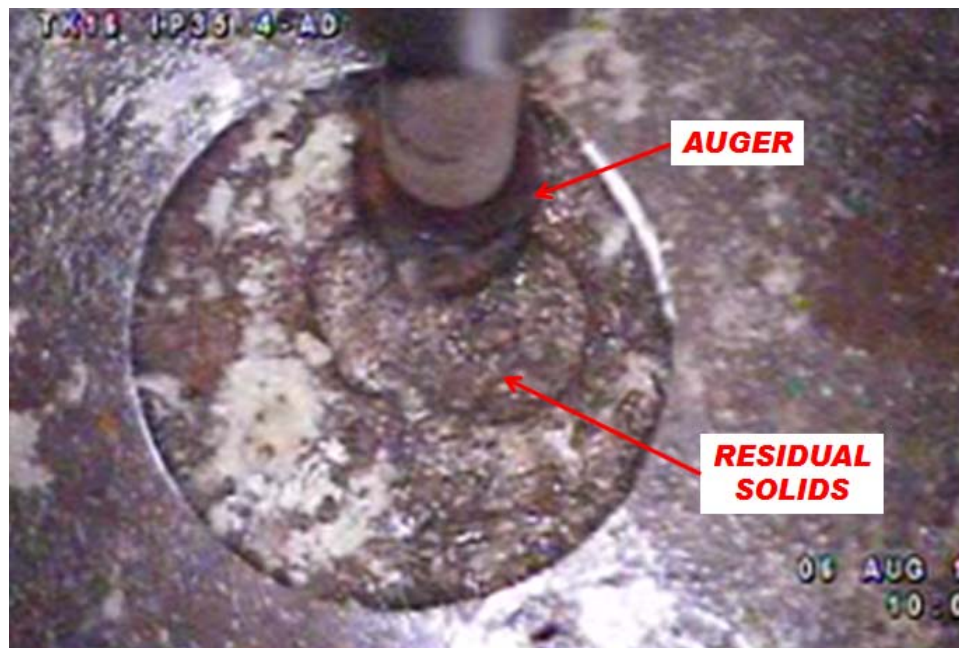
Figure 17: (Sample at IP-35. Sample bore location visible from above. SRR-LWE-2013-0027)
