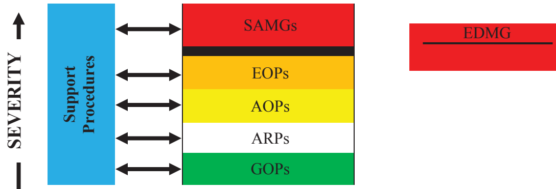
(b) Future View of Typical Operating Procedure Hierarchy
