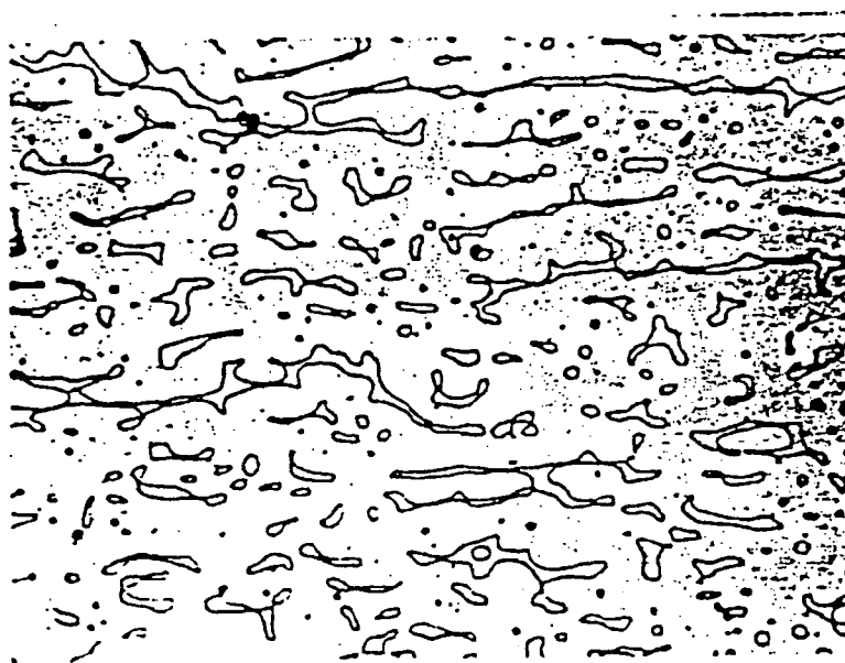
Figure 4-3. Microstructure of Solution Heat Treated Grade CF8 Stainless Steel Casting (Showing Ferrite Phase in Austenitic Matrix)
