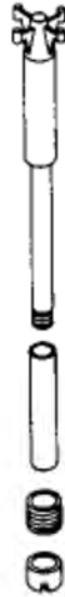
Figure 4-34 Typical Westinghouse core support column. Core support column bolts fasten the top of the support column to the lower core plate
