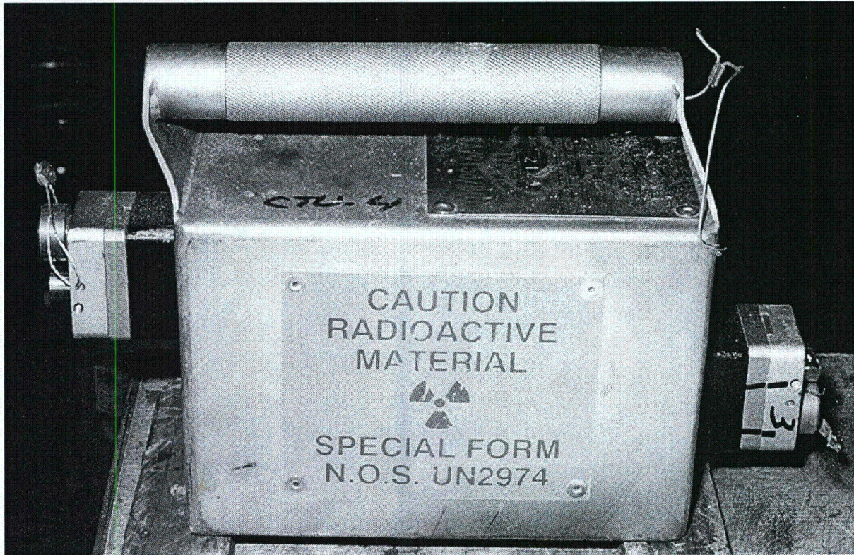
Figure 2.12.1-38 – CTU-4 Post-Test Disassembly: Condition of Handle
