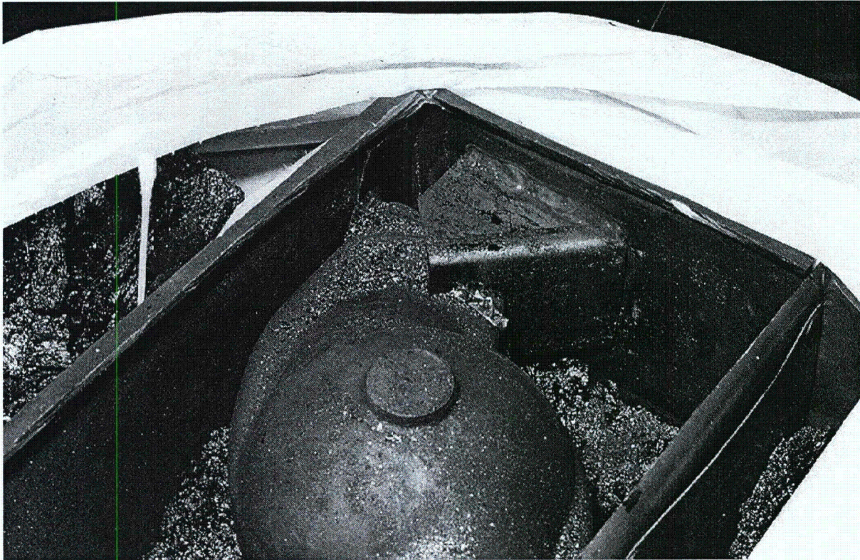
Figure 2.12.1-31 – CTU-3 Post-Test Disassembly: DU Support Bracket Welds and Copper Shims
