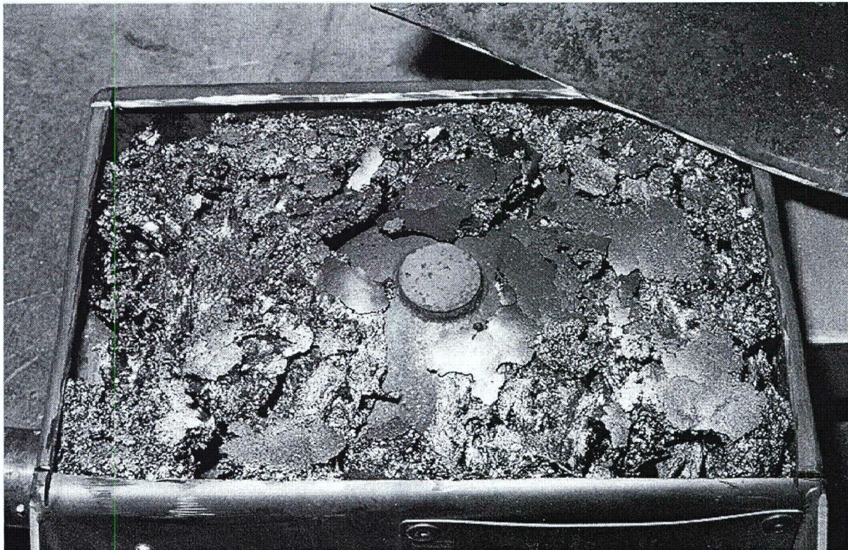
Figure 2.12.1-28 – CTU-3 Post-Test Disassembly: Illustrating Polyurethane Foam Char
