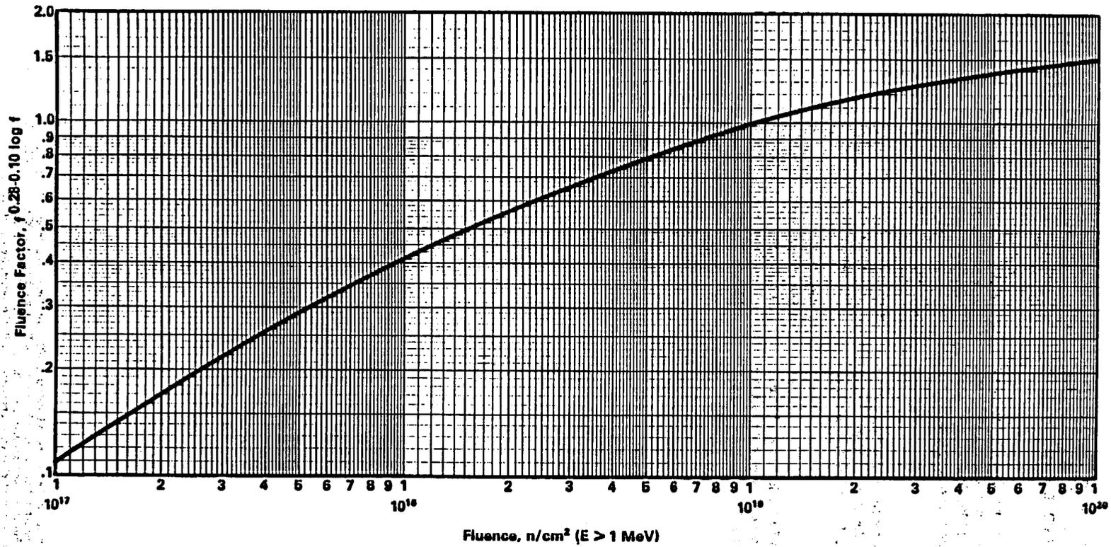
FIGURE 1 Fluence Factor for Use in Equation 2, the Expression for ART<sub>NDT</sub>
