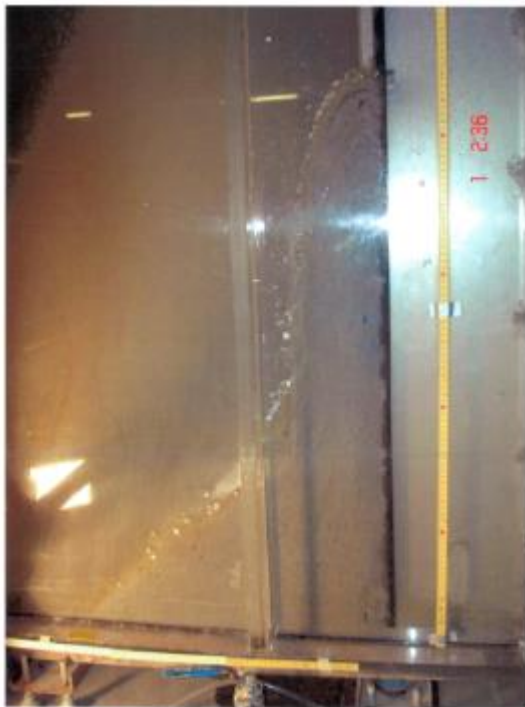
Picture 27: Debris layer without precipitate
