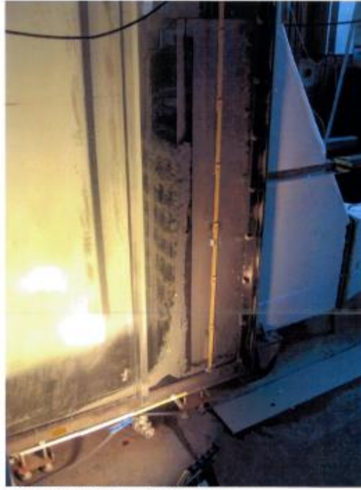
Picture 28: Debris layer at approximate 75 mbar head loss
