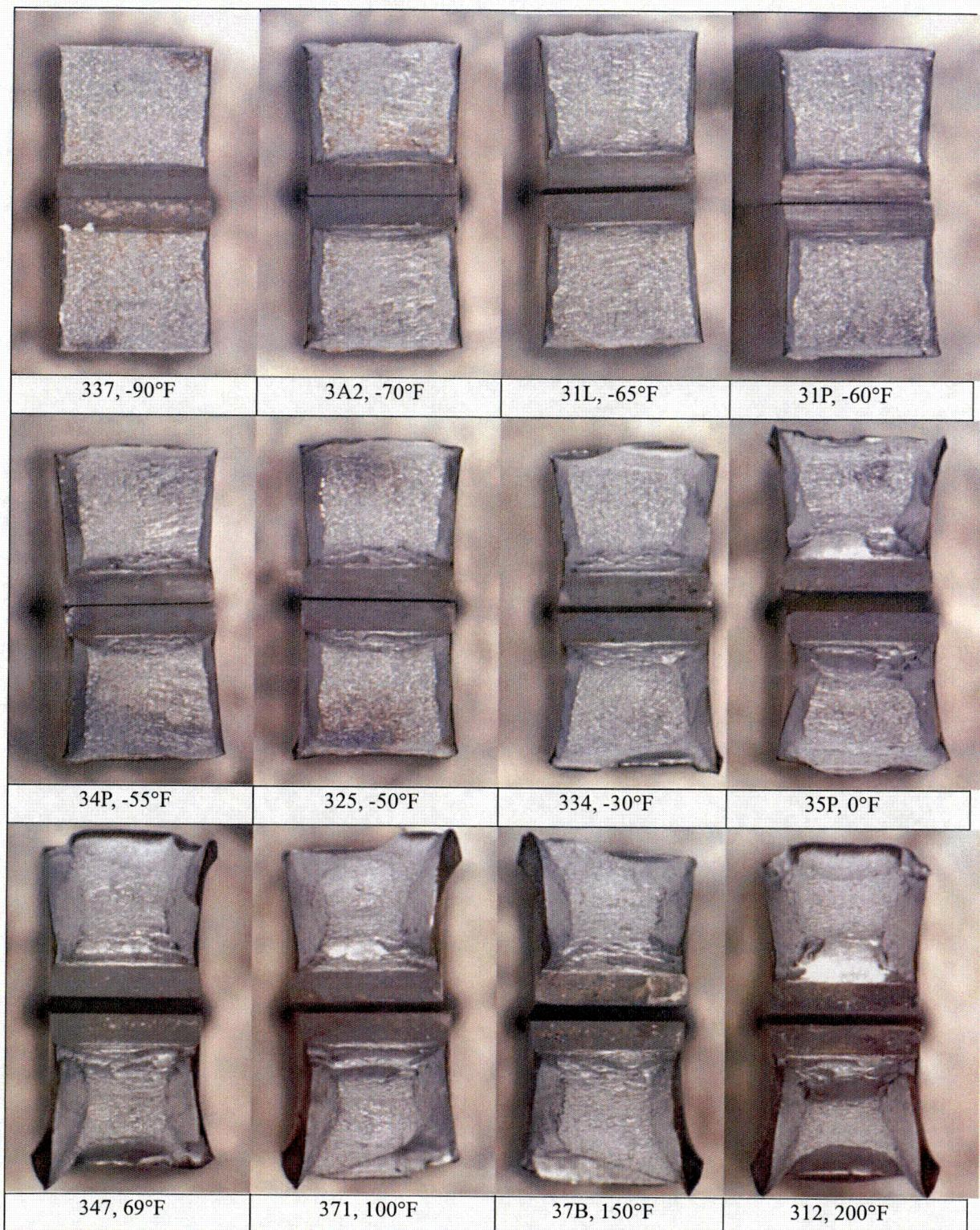
**Figure 5-18 Charpy Impact Specimen Fracture Surfaces for the Waterford Unit 3 Reactor Vessel Surveillance Program Weld Material (Heat # 88114)**
