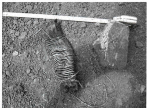
Photo #: PGE Decommission IF-5 View: Close-up Description: Sampling of other debris included a burnt length of fire hose and several fire brick fragments
