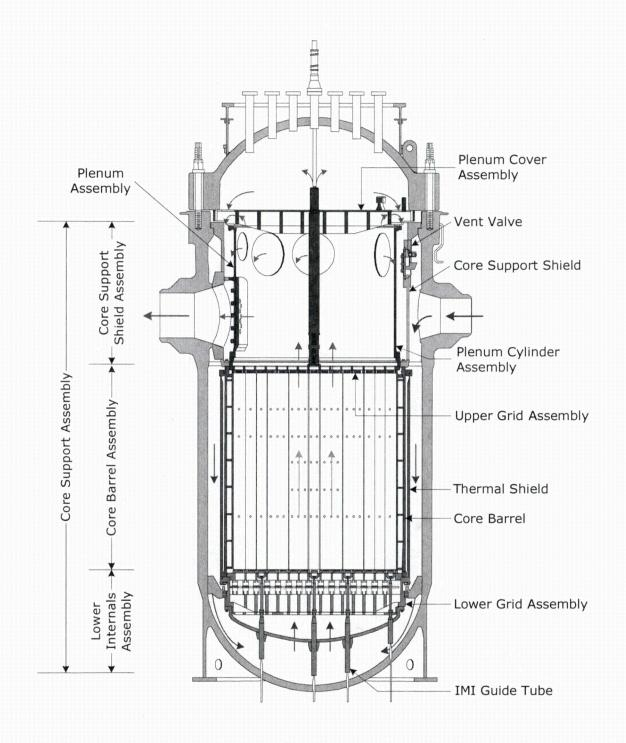
Figure 3-6 Typical B&W Reactor Vessel and Internals Arrangement
