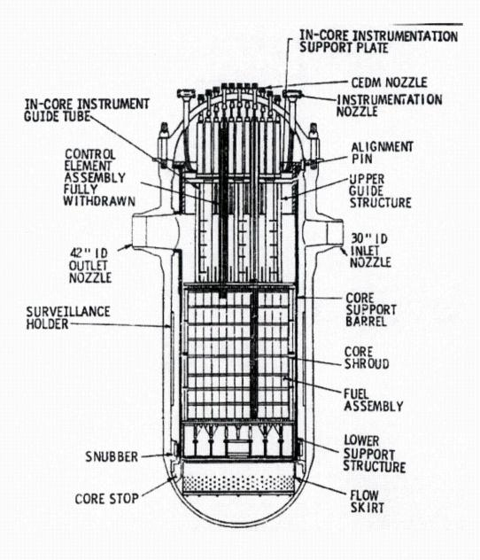
Figure 3-5 Typical CE Reactor Vessel and Internals Arrangement
