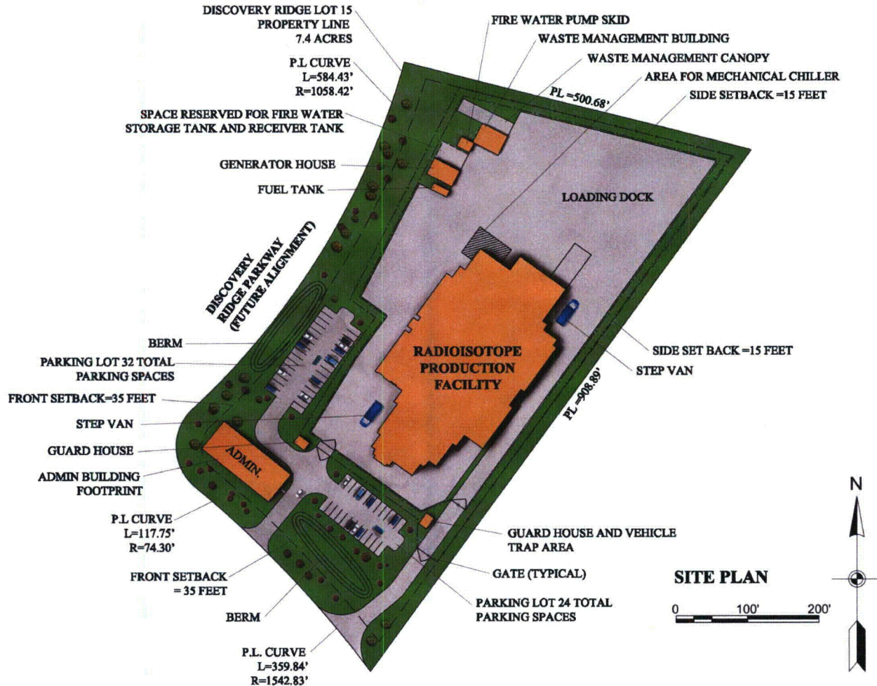
Figure 19-7. Radioisotope Production Facility Site Layout
