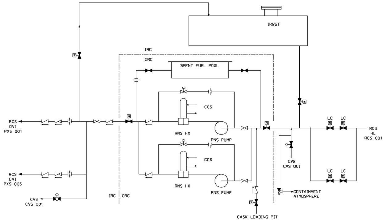
Figure 5.4-6 Normal Residual Heat Removal System
