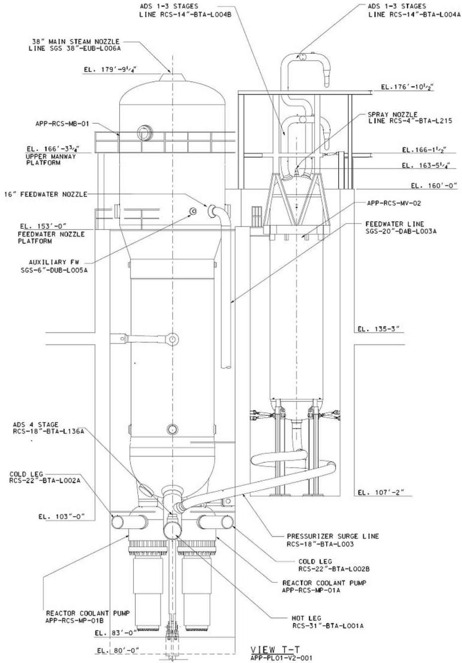
**Figure 5.1-4 Reactor Coolant System – Elevation**
