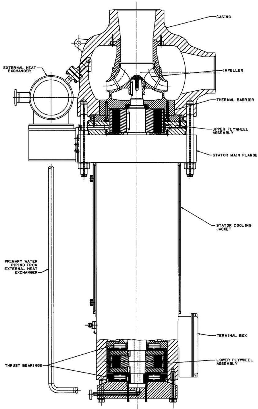
Figure 5.4-1 Reactor Coolant Pump
