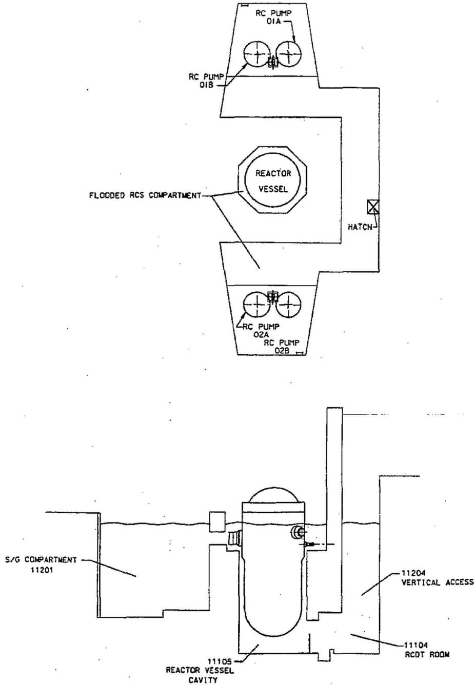
Figure 5.3-8 RCS Flooded Compartments During Ex-Vessel Cooling
