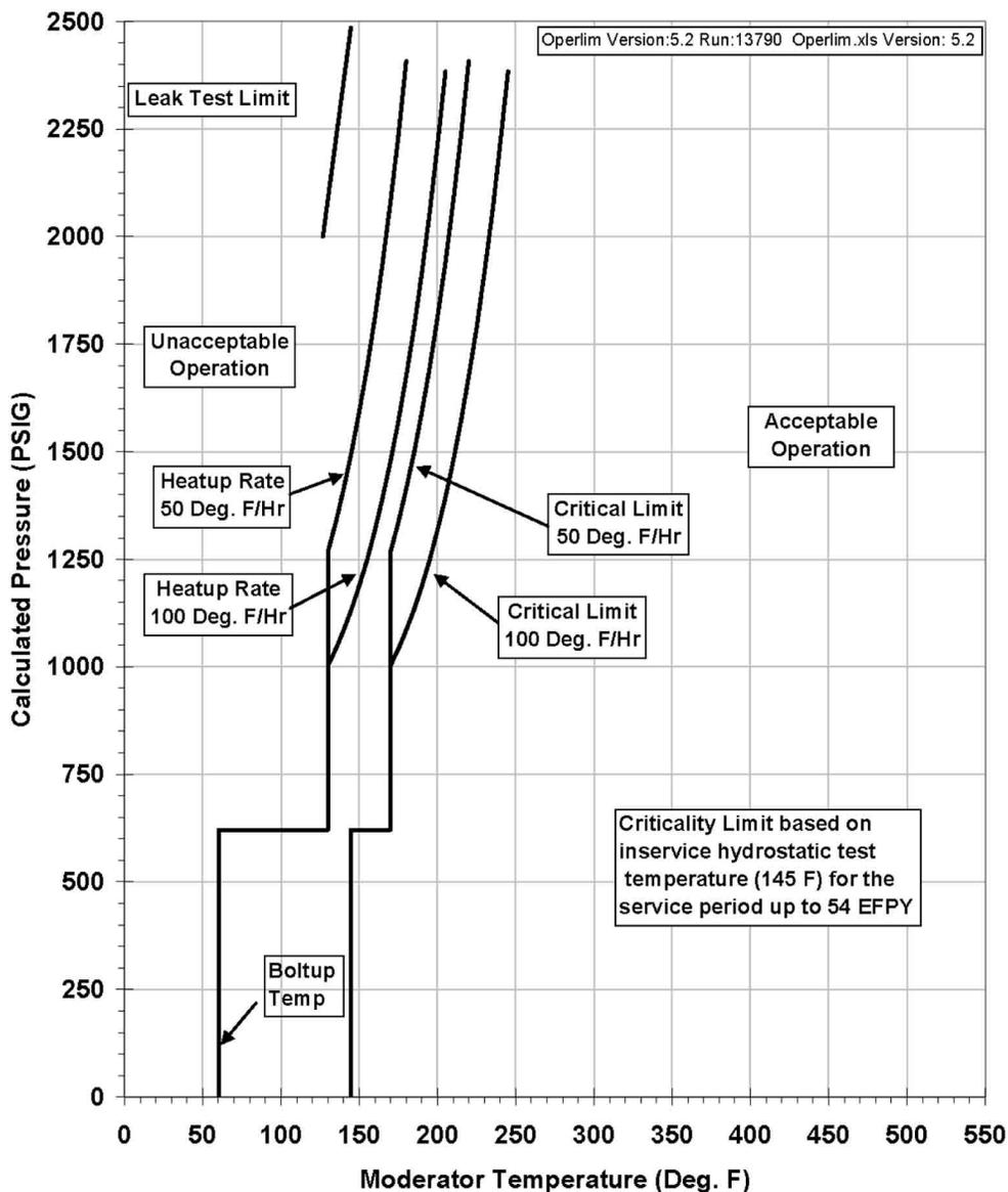
Figure 5.3-2 AP1000 Reactor Coolant System Heatup Limitations (Heatup Rate Up to 50° and 100°F/hour) Representative for the First 54 EFPY (Without Margins for Instrumentation Errors)
