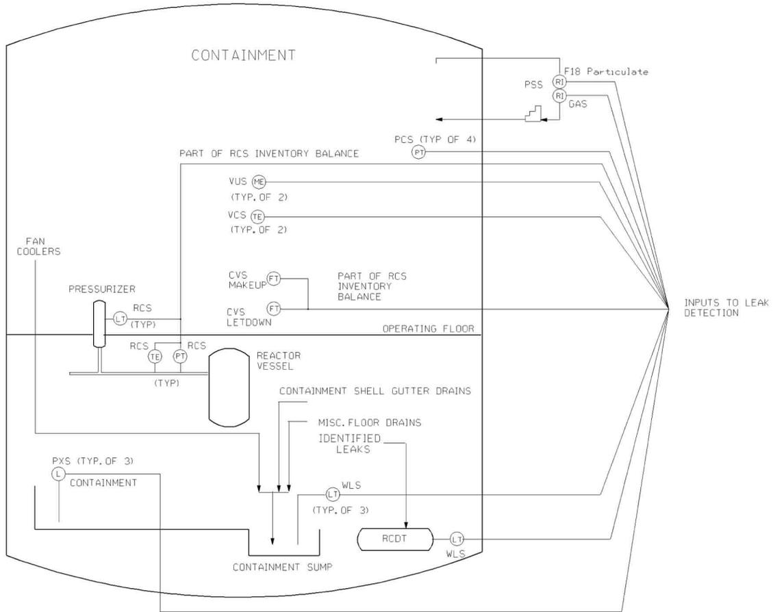
Figure 5.2-1 Leak Detection Approach
