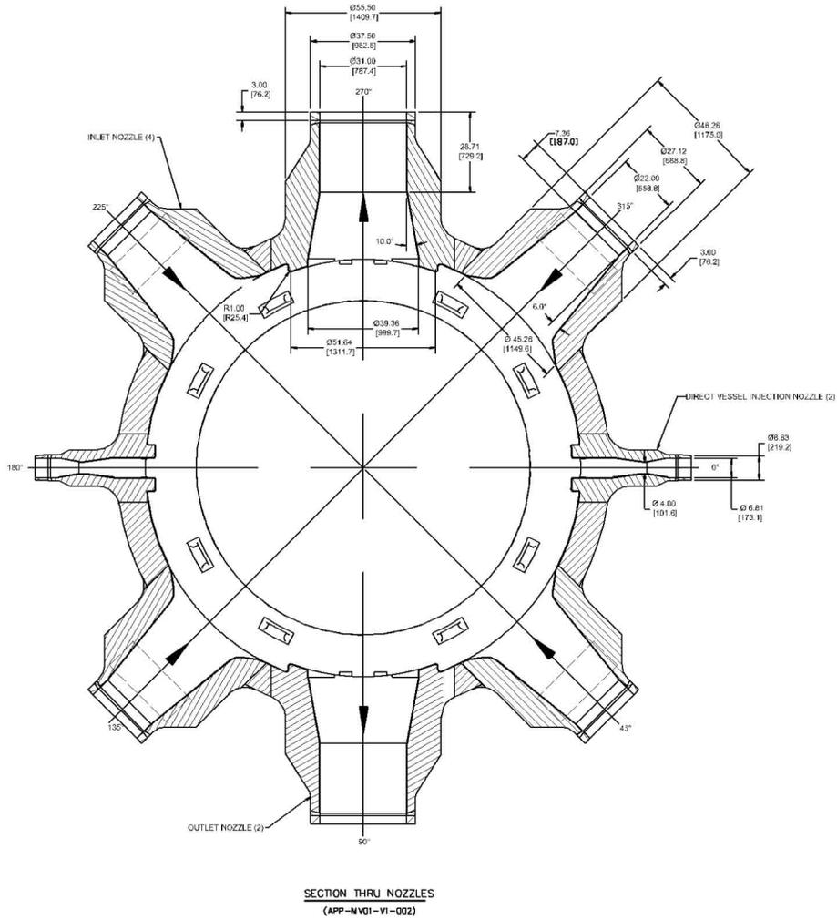
Figure 5.3-5 Reactor Vessel Key Dimensions Plan View
