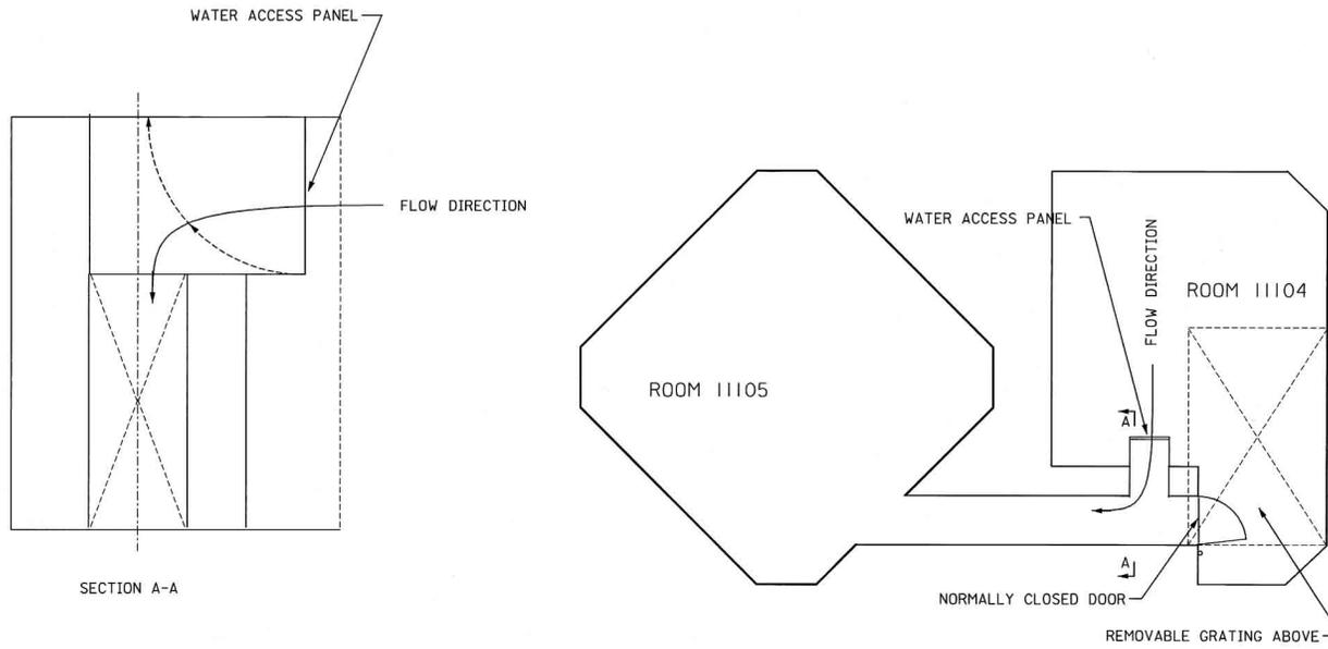
Figure 5.3-9 Door Between RCDT Room and Reactor Cavity Compartment
