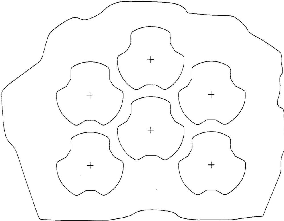
**Figure 5.4-3 Support Plate Geometry (Trifoil Holes)**
