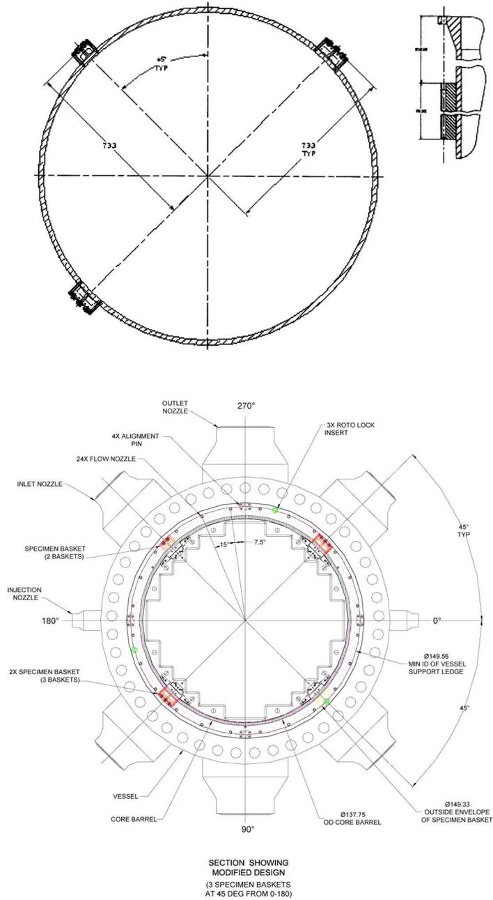
Figure 5.3-4 AP1000 Reactor Vessel Surveillance Capsules Locations
