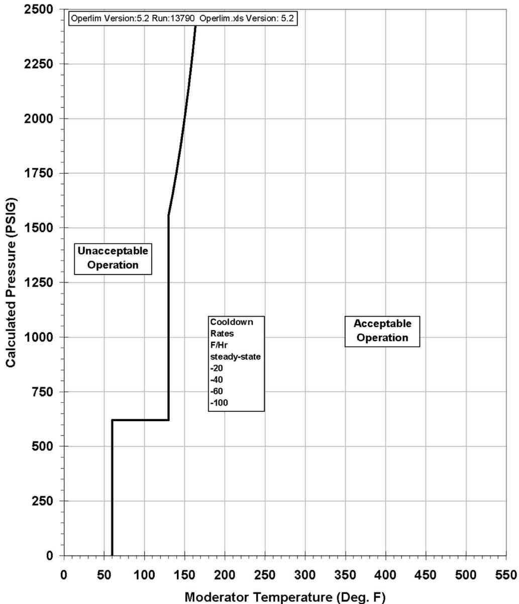
Figure 5.3-3 AP1000 Reactor Coolant System Cooldown Limitations
