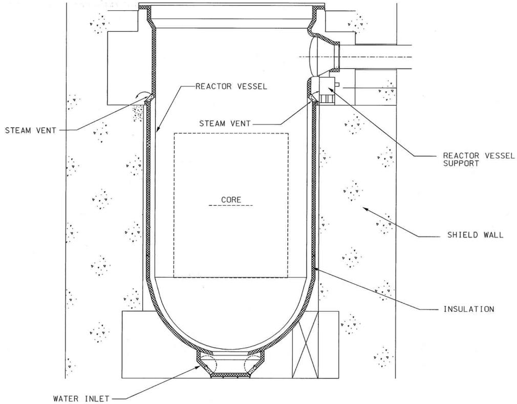
Figure 5.3-7 Schematic of Reactor Vessel Insulation
