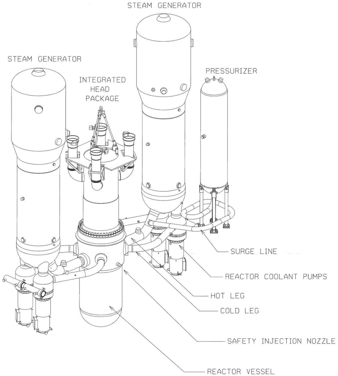
Figure 5.1-2 Reactor Coolant Loops – Isometric View
