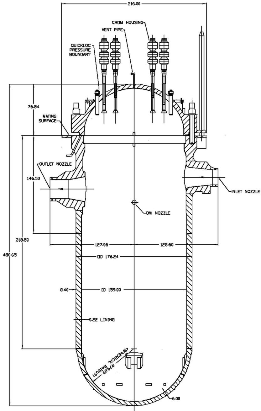
Figure 5.3-6 Reactor Vessel Key Dimensions, Side View
