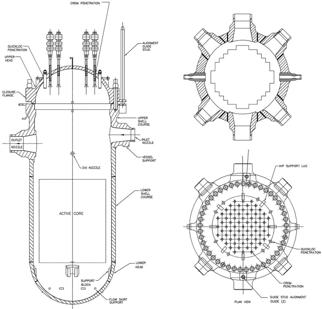
Figure 5.3-1 Reactor Vessel
