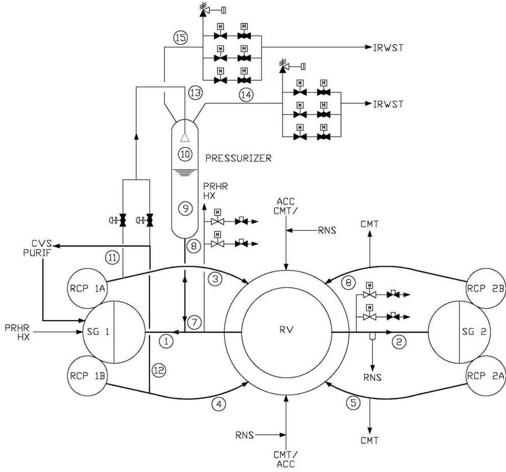
Figure 5.1-1 Reactor Coolant System Schematic Flow Diagram
