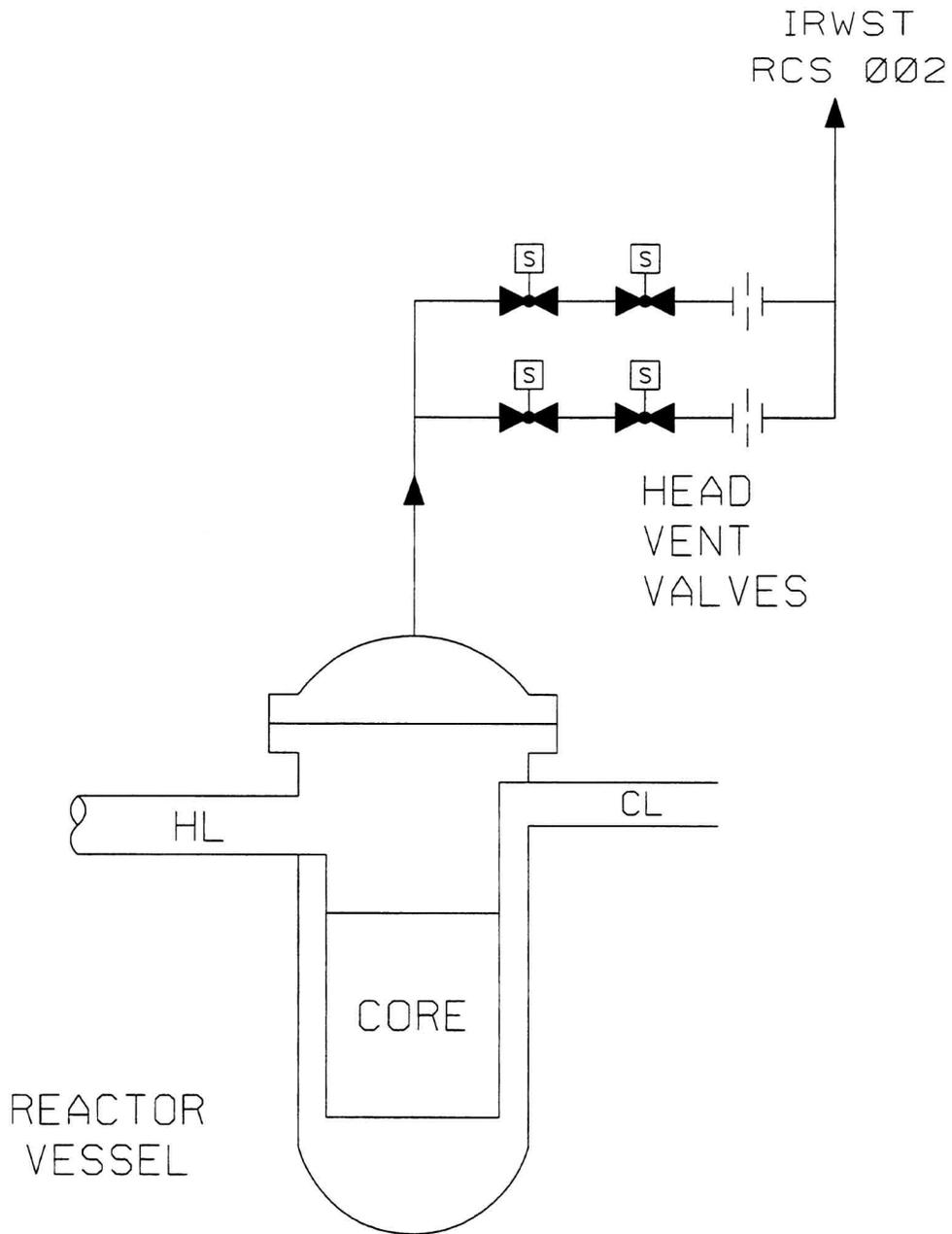
Figure 5.4-8 Reactor Vessel Head Vent System
