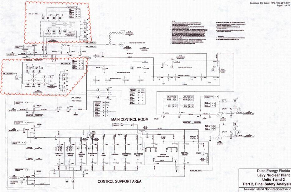
Units 1 and 2 Part 2, Final Safety Analysis Report Nuclear Island Non-Radioactive Ventilation System Piping and Instrumentation Diagram FIGURE 9.4-201
