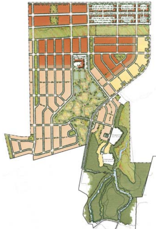
impervious areas reduced by lessening road length through clustering of development (Plano, IL) (Conservation Design Forum)
