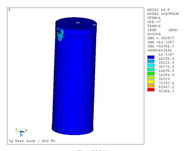
Figure 3.9.5-11 Stress Intensity (psi) Plot for Load Case 3g
