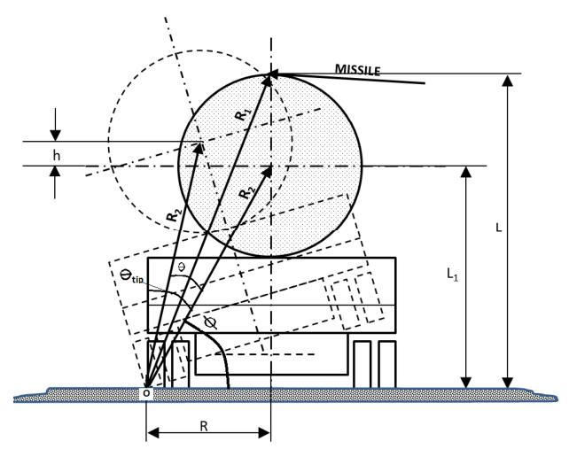
Figure 3.9.7-10 Stability Geometry of TC on Transfer Trailer
