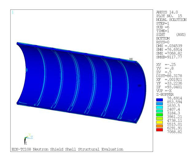
$\label{eq:Figure 3.9.5-15} EOS\text{-}TC108 \ Neutron \ Shield \ Panel \ Stress \ Intensity \ (P_m+P_b) \ Plot \ Load \ Case \\ E1$
