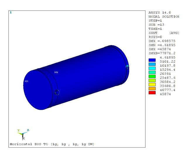
Figure 3.9.5-12 Stress Intensity (psi) Plot for Load Case Horizontal Transfer on Skid
