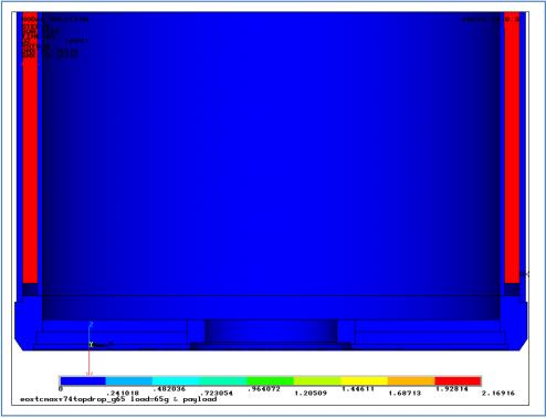
Figure 3.9.5-21 Bottom and Top, respectively, End Drops - Load 65g - Lead Slump Displacements
