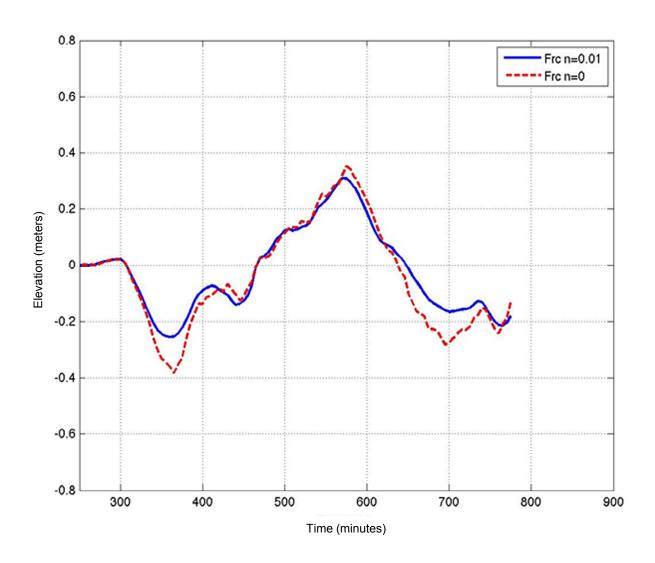
Frc = Friction n = Manning's Roughness Coefficient
