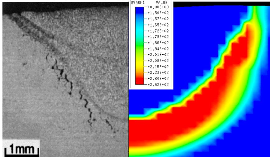
High Tensile Residual Stresses Modeled
