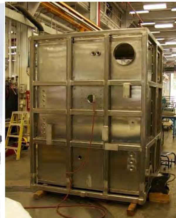
Welding Hot Cell fabrication at ORNL
