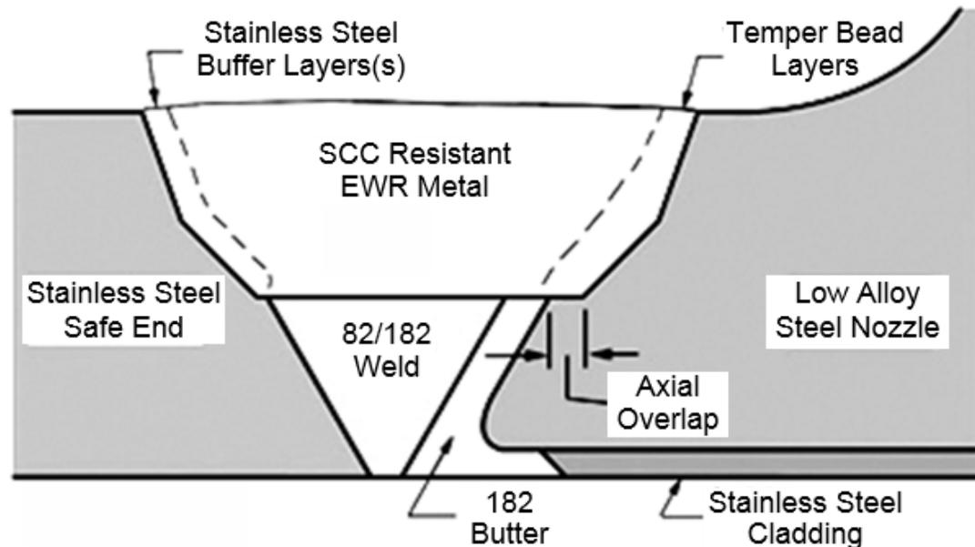
Schematic of EWR for 82/182 PWSCC Mitigation
