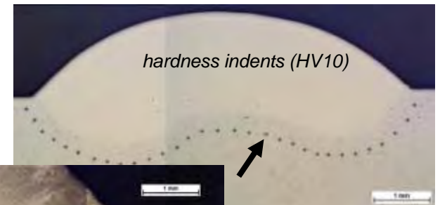
Hydrogen Testing SMAW TB – Code Case N-839
