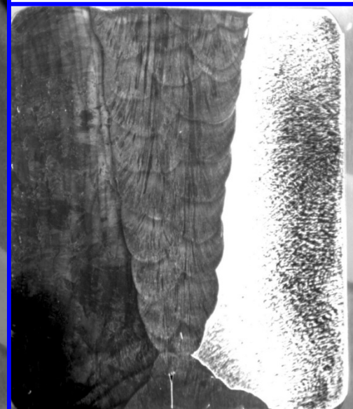
Phase 2B alloy 182 dissimilar metal nozzle weld
