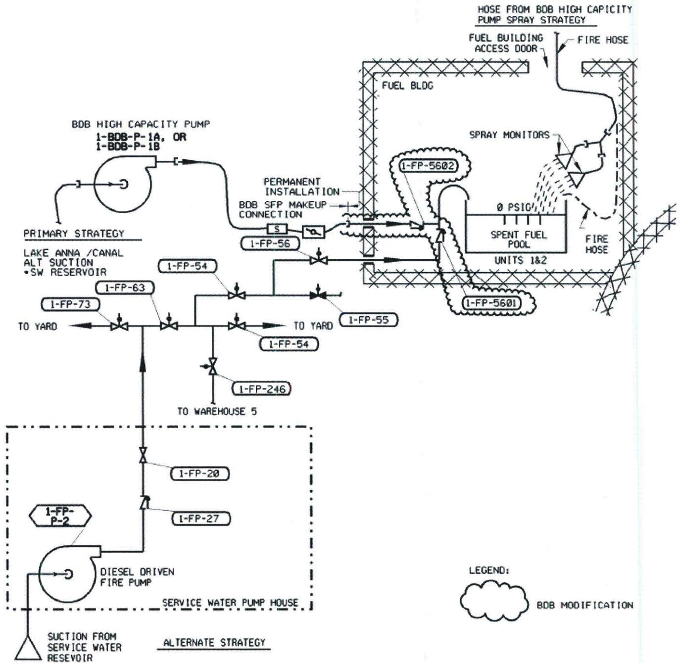
Figure 18: Spent Fuel Pool Cooling Primary and Alternate Mechanical Connections
