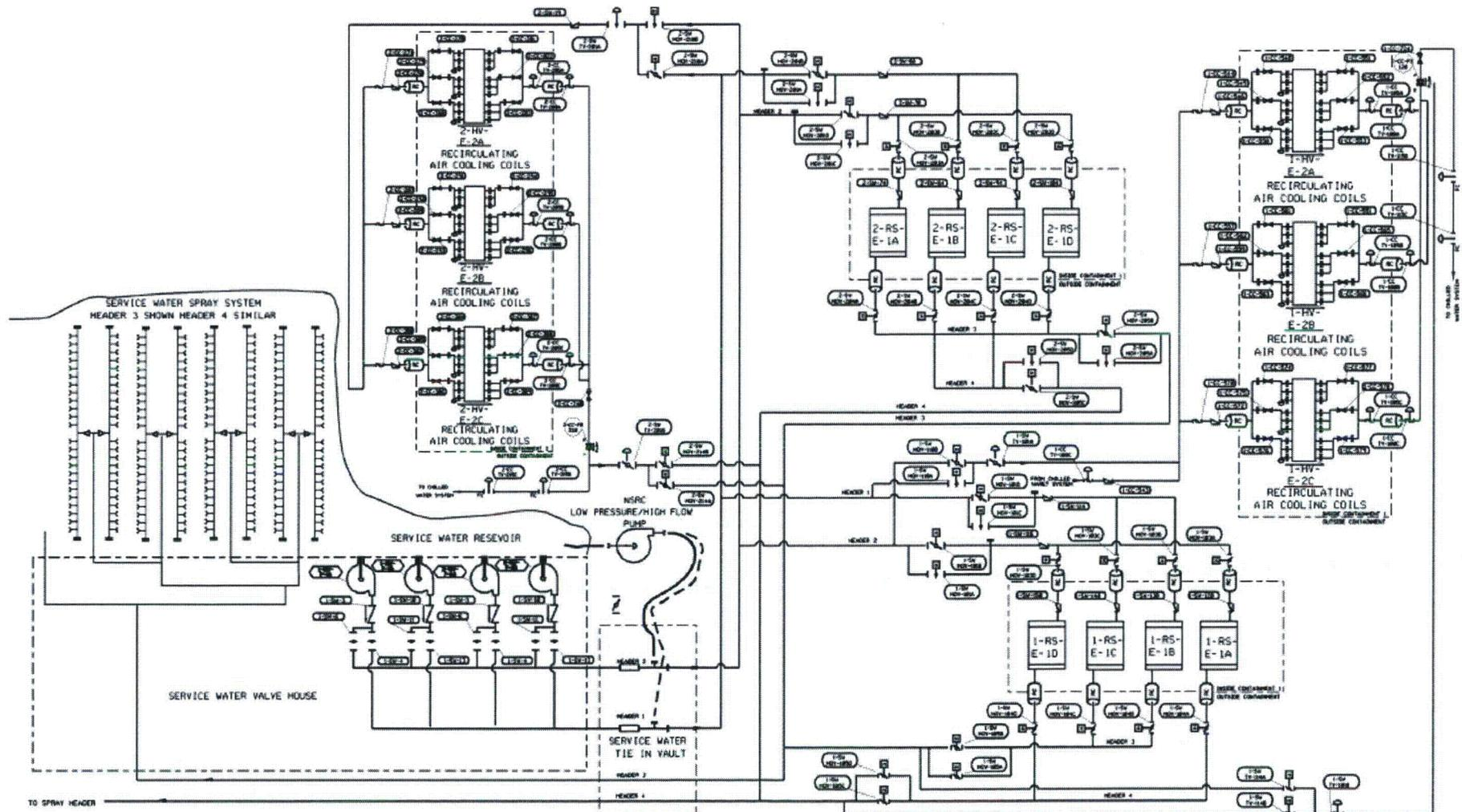
Figure 19: Phase 3 Containment Cooling Connections
