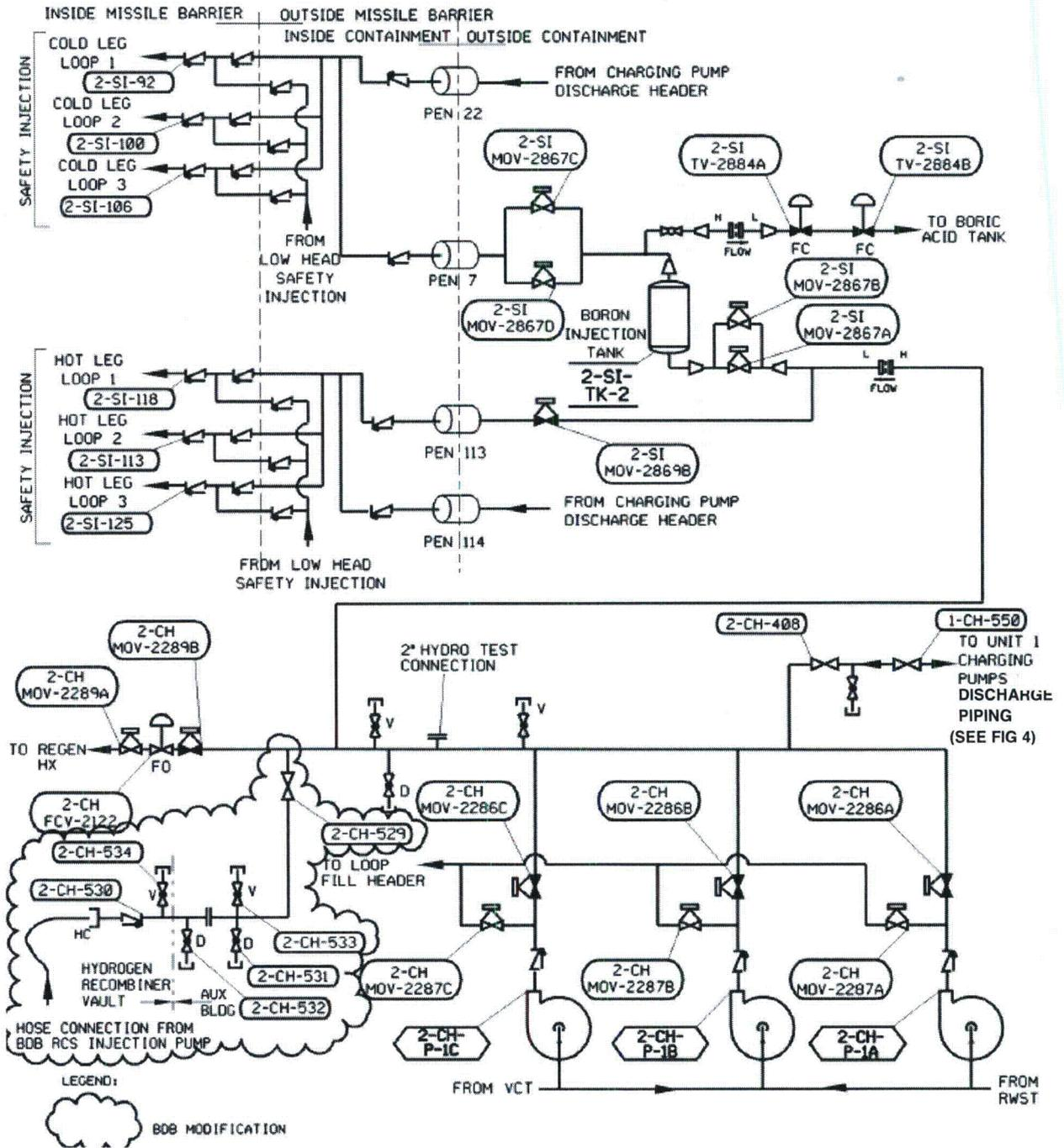
Figure 5: RCS Makeup Alternate Mechanical Connection
