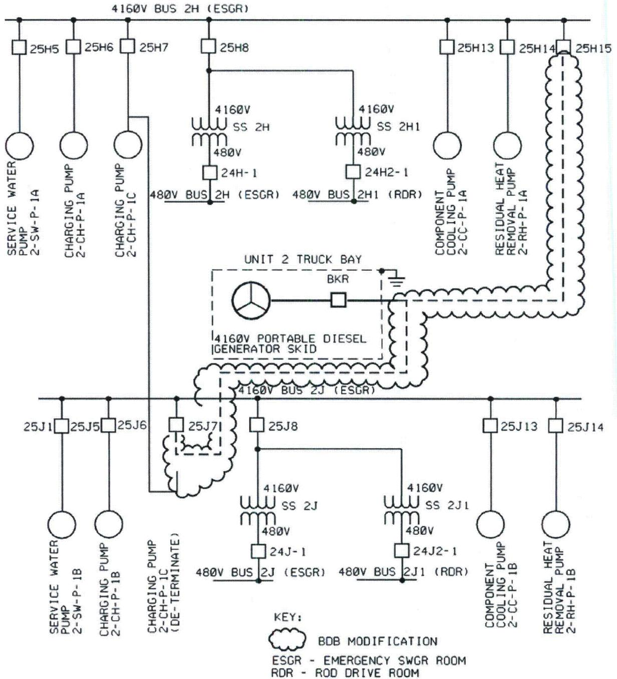
Figure 17: 4160 VAC Generator (NSRC) Electrical Connections to 4160 VAC MCC 2H and 2J – North Anna Unit 2
