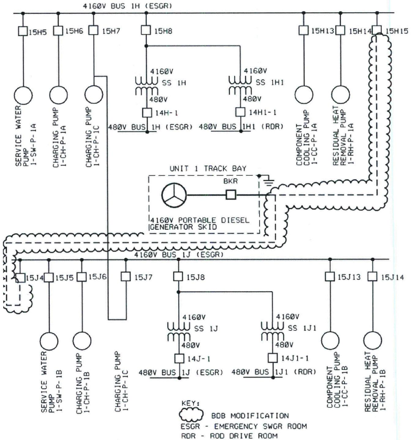
Figure 16: 4160 VAC Generator (NSRC) Electrical Connections to 4160 VAC MCC 1H and 1J – North Anna Unit 1
