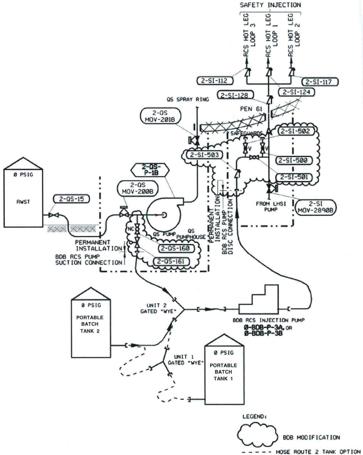
Figure 3: RCS Makeup Primary Mechanical Connection
