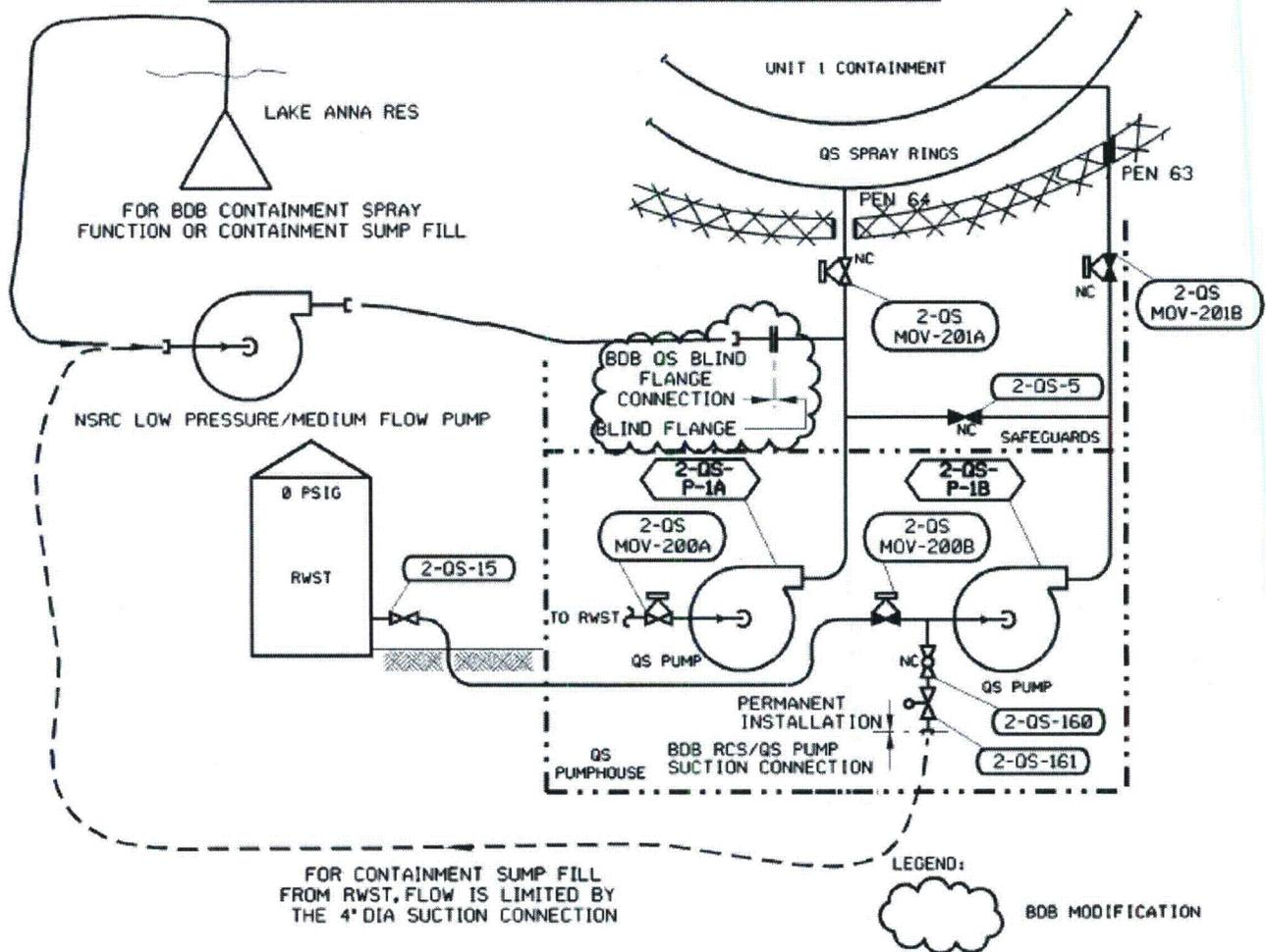
Figure 21: Containment Cooling Phase 3 Containment Spray Mechanical Connections North Anna Unit 2
