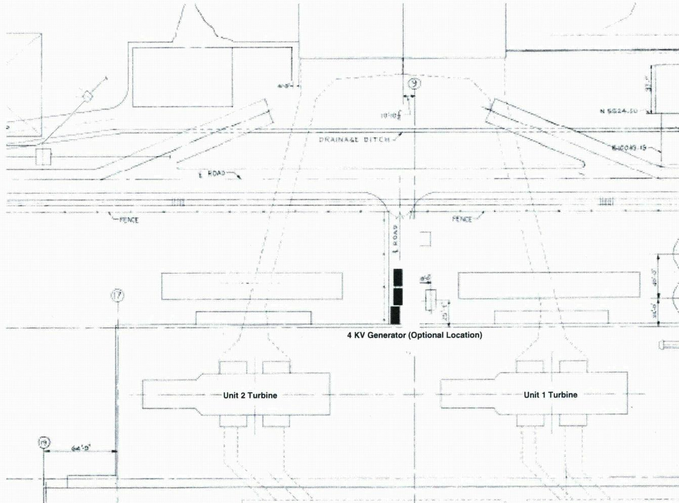
Figure 11: 4160 VAC Generator (NSRC) Electrical Connection General Layout
