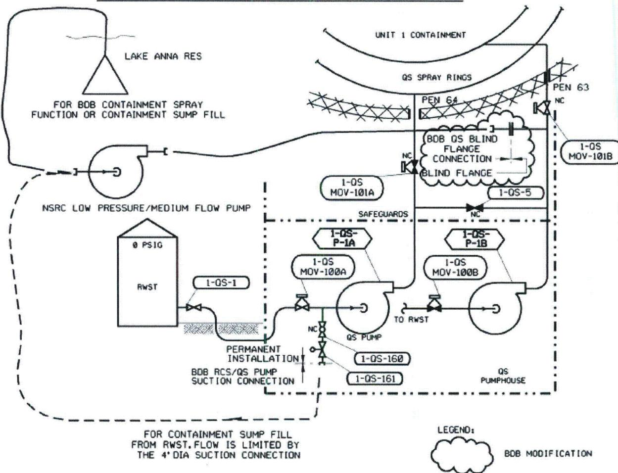
FOR CONTAINMENT SUMP FILL FROM RWST, FLOW IS LIMITED BY THE 4" DIA SUCTION CONNECTION
