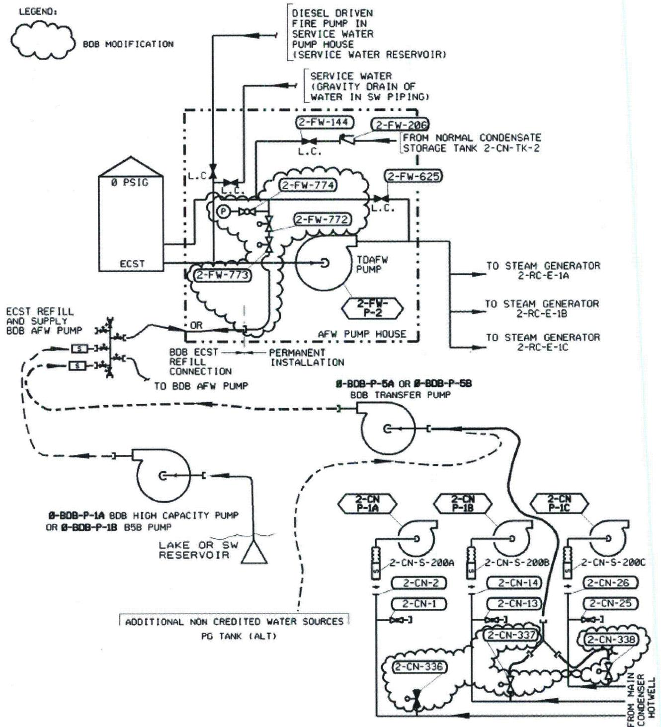
Figure 15: ECST Refill Mechanical Connections, Paths, and Sources
