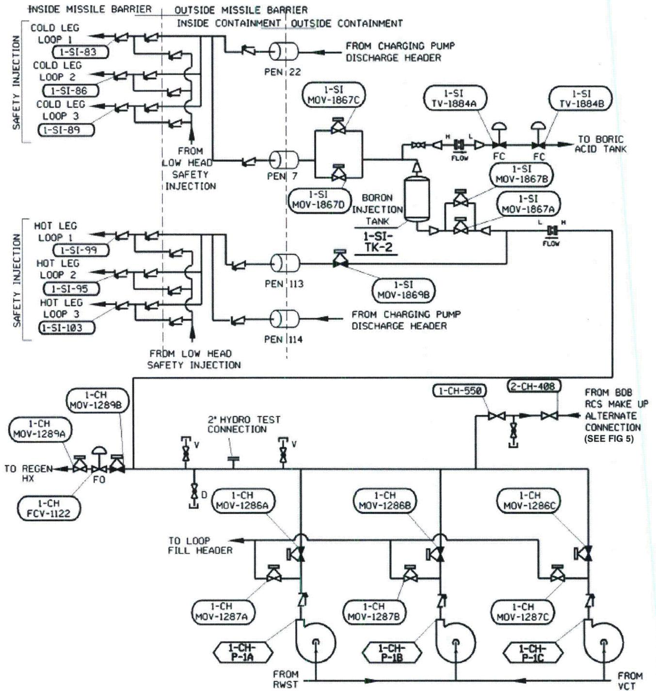
Figure 4: RCS Makeup Alternate Mechanical Connection
