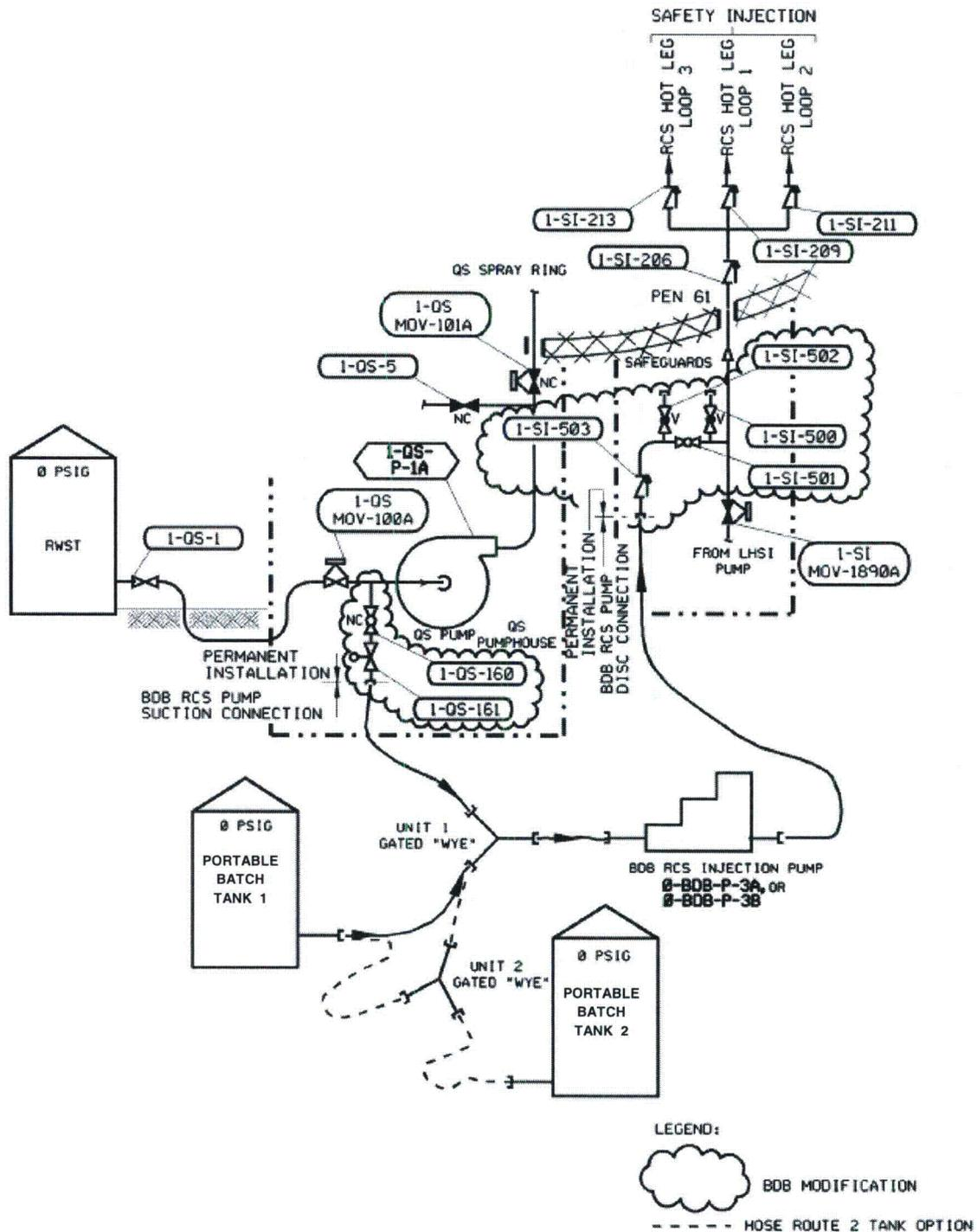
Figure 2: RCS Makeup Primary Mechanical Connection
