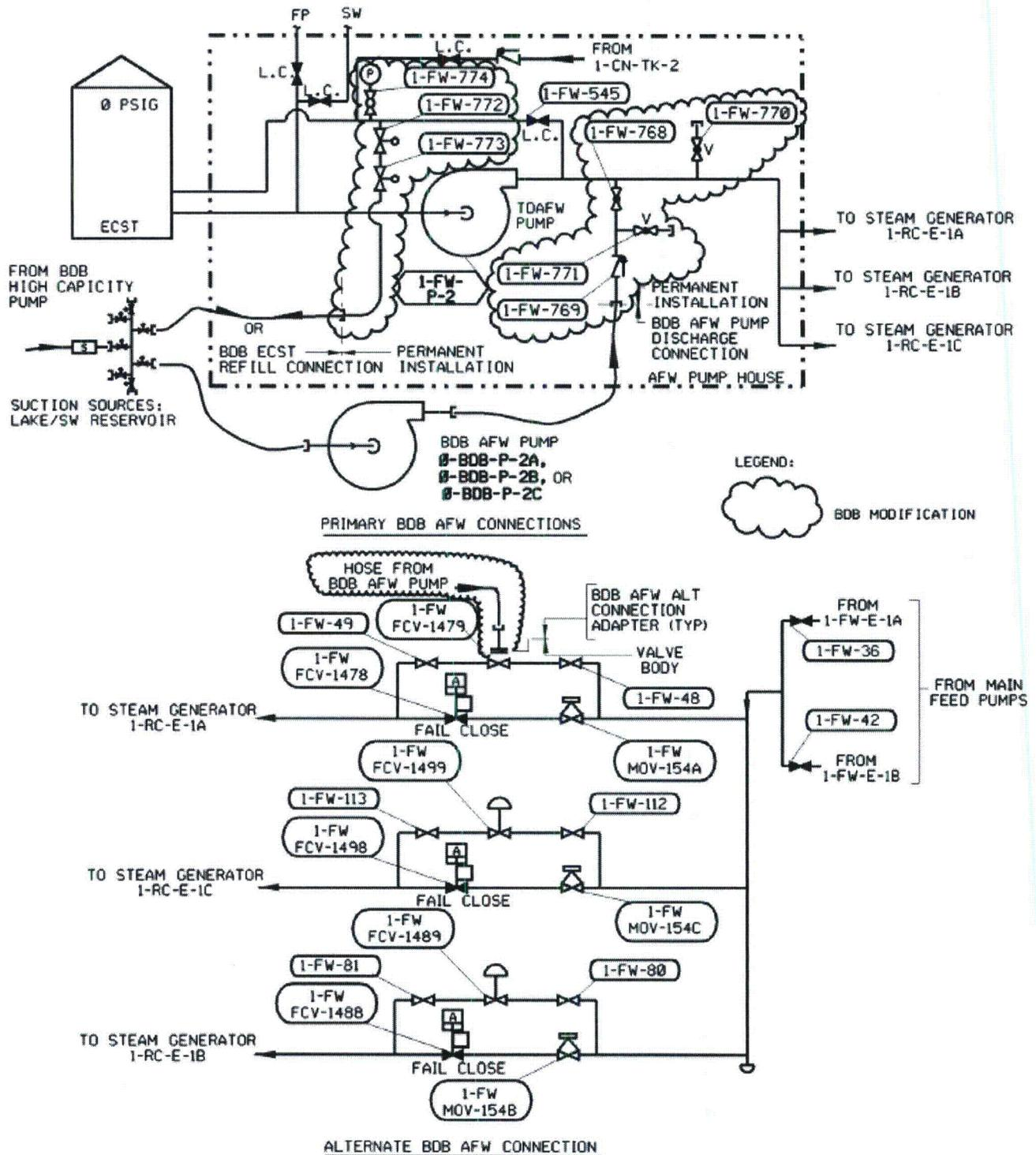
Figure 12: Core Cooling and Decay Heat Removal AFW Primary and Alternate Mechanical Connections – North Anna Unit 1
