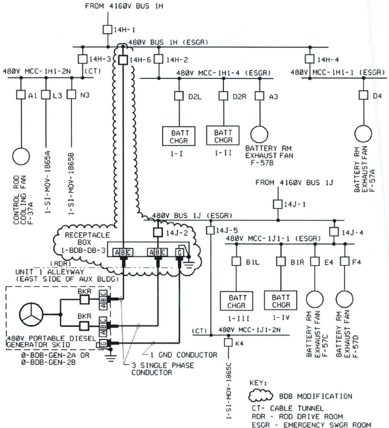
Figure 9: 480 VAC Portable Generator (BDB) Electrical Connections to 480 VAC MCC 1H and 1J – North Anna Unit 1
