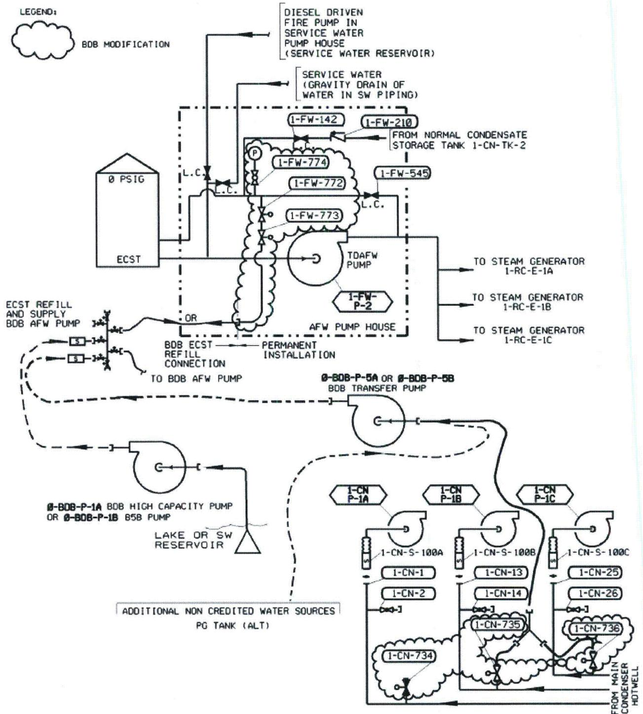
Figure 14: ECST Refill Mechanical Connections, Paths, and Sources
