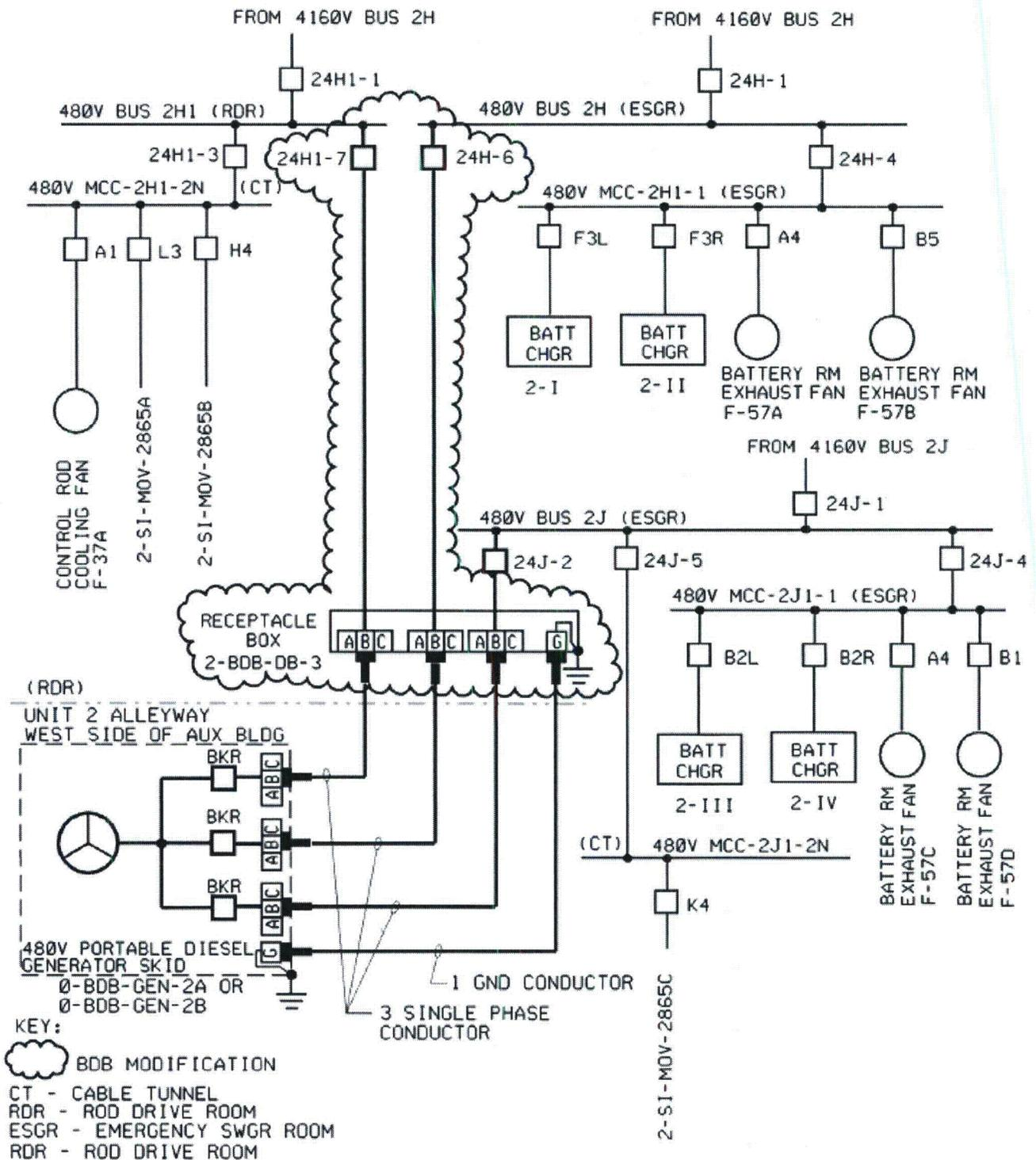
Figure 10: 480 VAC Portable Generator (BDB) Electrical Connections to 480 VAC MCC 2H and 2J – North Anna Unit 2
