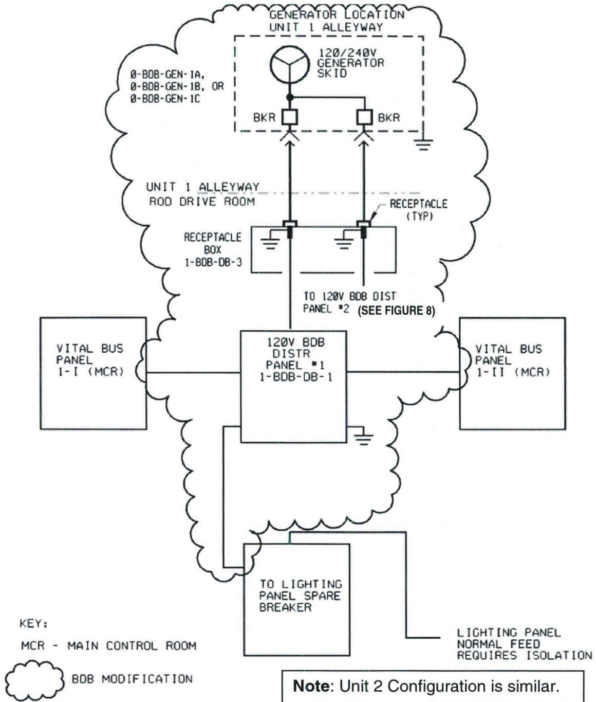
Figure 7: 120/240 VAC Portable Generator (BDB) Electrical Connection
