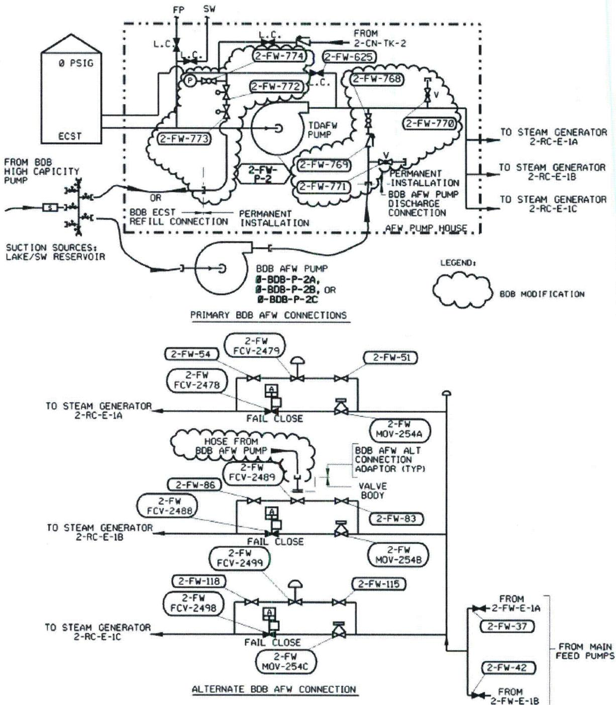
Figure 13: Core Cooling and Decay Heat Removal AFW Primary and Alternate Mechanical Connections – North Anna Unit 2
