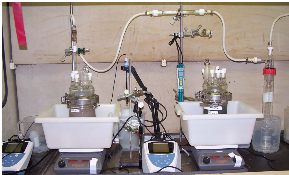
Figure 2-2. Photograph of Experimental Equipment to Prepare Larger Bench-Scale Quantities of Pore Waters
