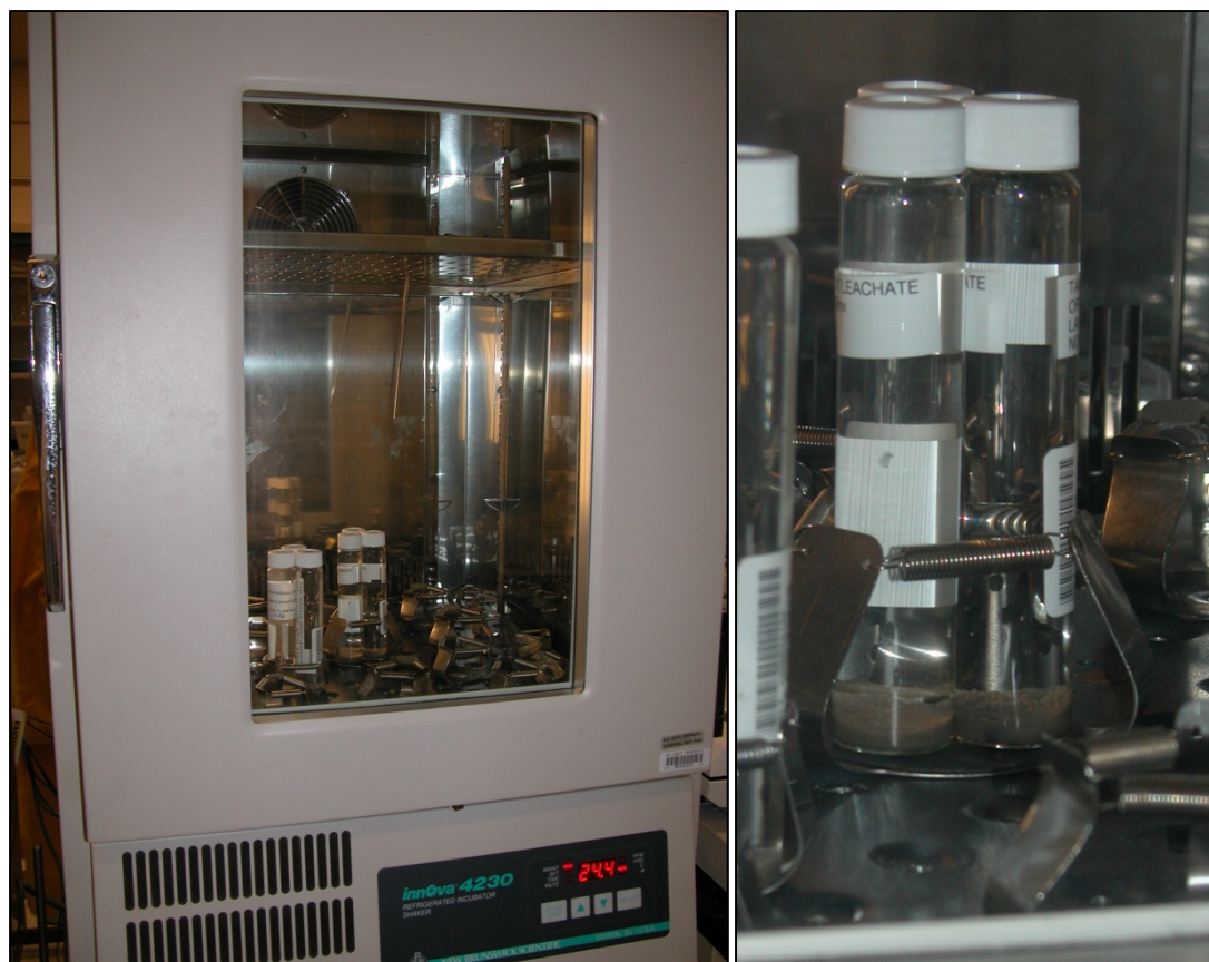
Figure 2-3. Photographs of Incubator Shaker Oven and Nested Glass Vials Inside Oven Used in Zero Head Space Tests
