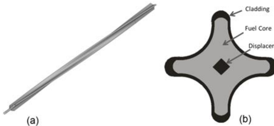
Figure 1. Schematic of Lightbridge's metallic fuel rod for PWRs. (a) Segment of rod showing helical twist; (b) cross-section showing the fuel core, central displacer and cladding. [Not to scale].
