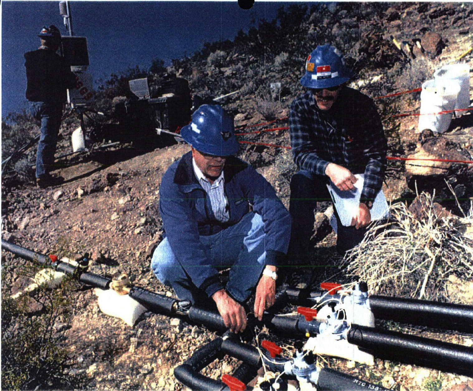
Infiltration and percolation studies being conducted by the USGS in Alcove 1. This slide shows water being infiltrated on top of Exile Hill.
