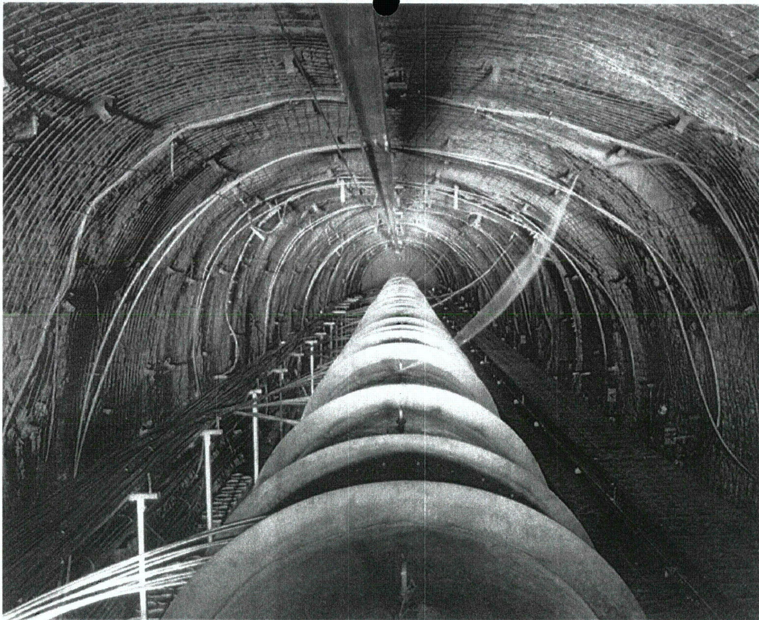
View of Canister #1 in the Heated Drift. The Drift Scale Test was initiated on December 2, 1997 and is planned to run for up to eight years.
