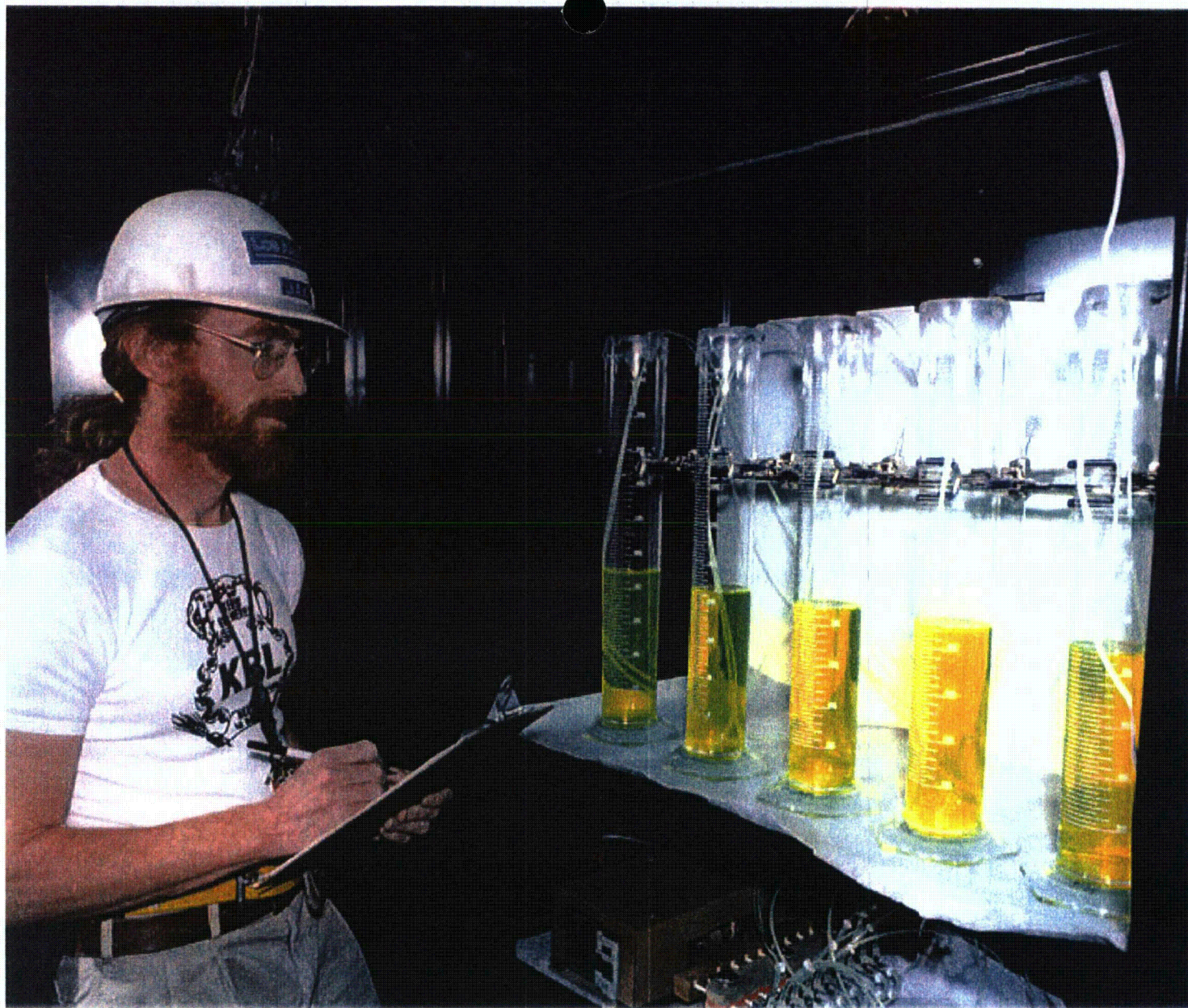
The collection of traced solution used during injection in the Unsaturated Zone Transport Test at Busted Butte. The tracer is a Flourescein Disodium Salt.
