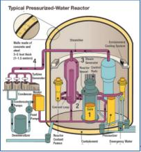
The control rods are composed of chemical elements that absorb neutrons created by the fission
