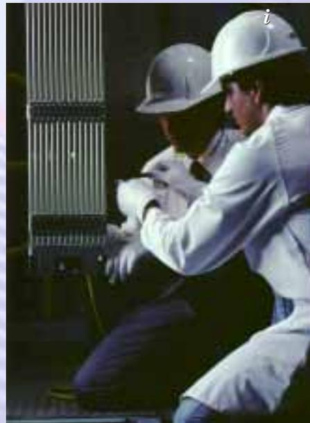
*Finished assemblies are inspected both before shipment (h) and upon arrival at the reactor site (i)*
