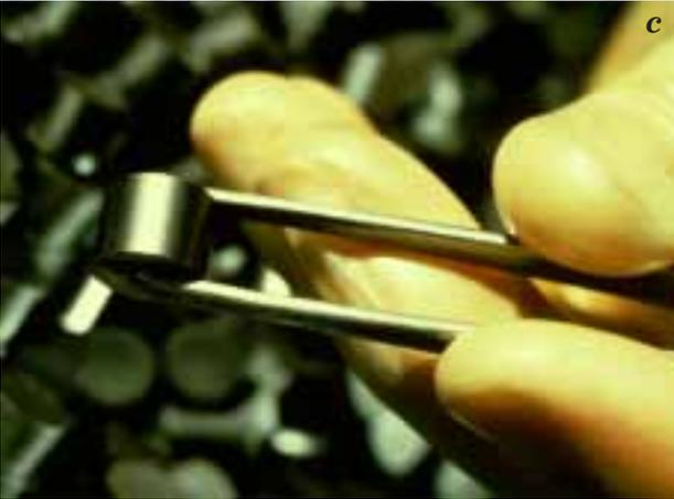
*UF<sub>6</sub> is received in cylinders (a), converted to UO<sub>2</sub> powder (b), and pressed into fuel pellets, which must pass strict quality inspections (c) before columns of pellets are loaded into fuel rods (d)*
