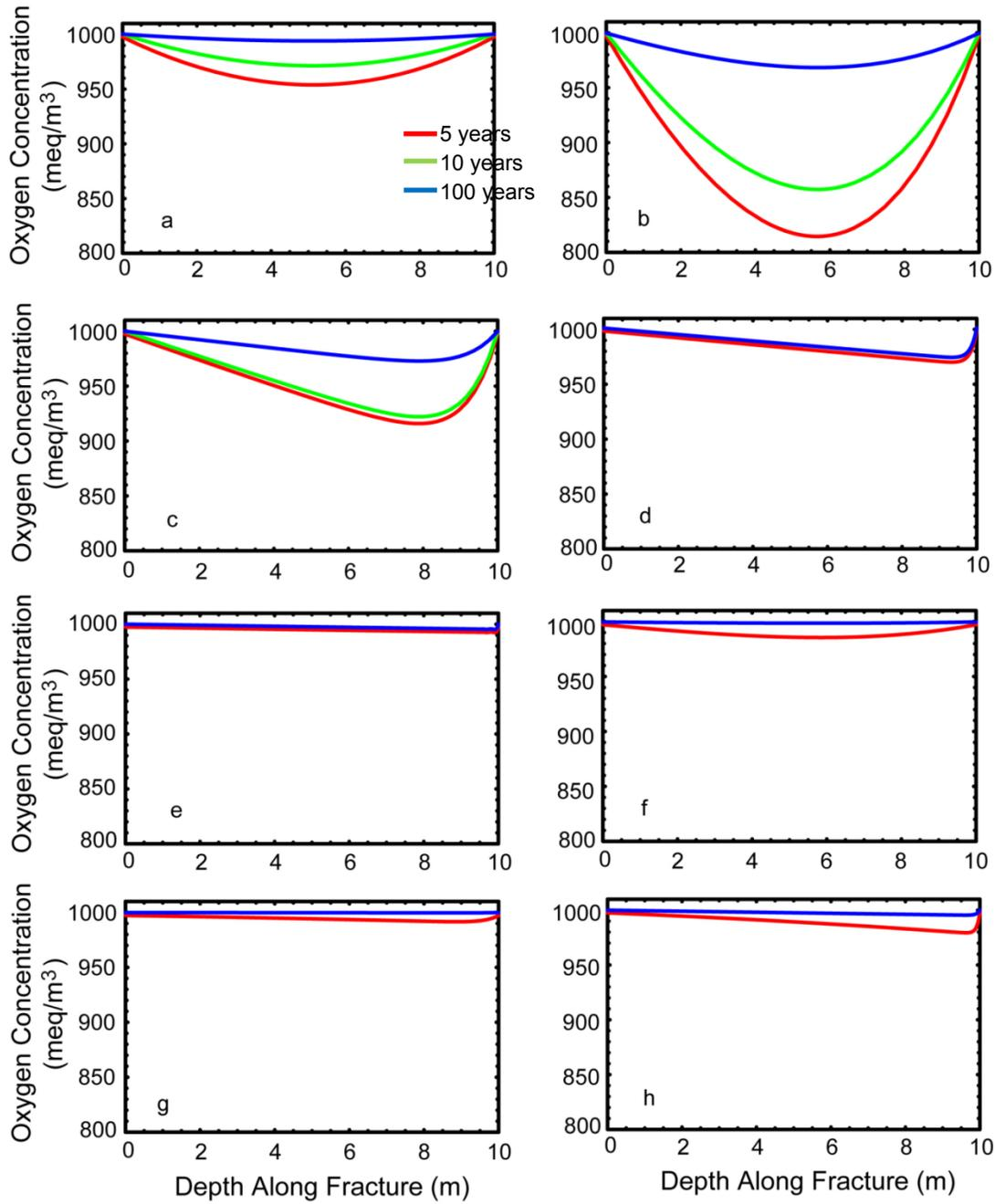
**Figure 3** Adapted from Painter and Pabalan (2009). Fracture aperture, saturation, and porosity are as follows for each case: (a) 0.3 mm, 1.0, 0.15; (b) 0.1 mm, 1.0, 0.28; (c) 0.1 mm, 1.0, 0.43; (d) 0.1 mm, 1.0, 0.57; (e) 0.1 mm, 1.0, 0.87; (f) 10 mm, 0.25, 0.31; (g) 10 mm, 0.25, 0.58, (h) 10 mm, 0.25, 0.80.
