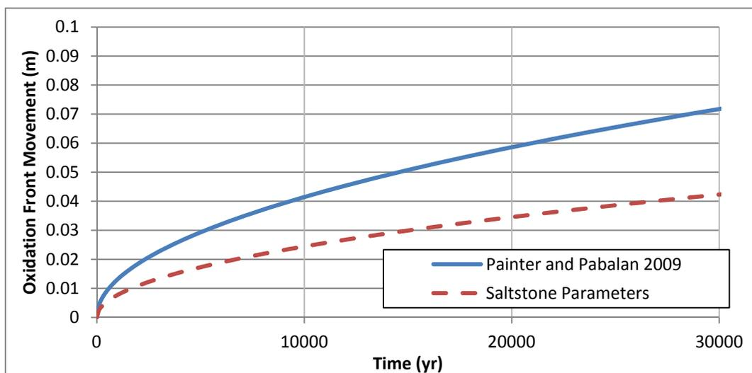
**Figure 4.** Oxidation projections based on the model of Painter and Pabalan (2009) and predictions modified for saltstone parameters, including a reducing capacity of  $0.607 \text{ meq e}^- / \text{g}$  saltstone, porosity of 0.58, density of  $1010 \text{ kg per m}^3$ , and effective diffusion coefficient of  $3.15 \times 10^{-5} \text{ m}^2 / \text{year}$ .
