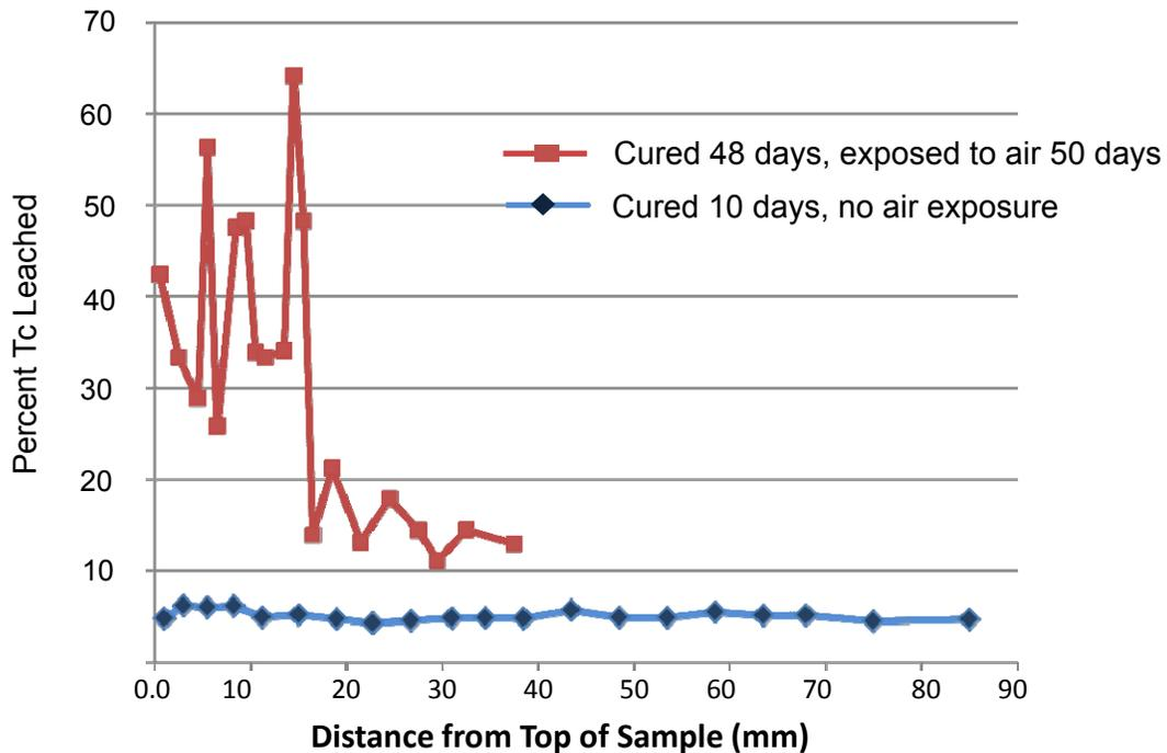
**Figure 2.** Adapted from Langton and Almond (2013) (SRNL-STI-2013-00541). Comparison of Tc-99 fraction leached as a function of distance from the top surface for a 10 day old and a 98 day old (exposed to air) Cast Stone sample.
