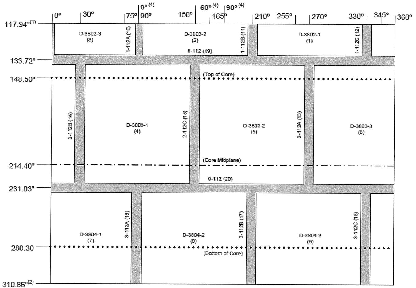
**Figure 4-1 Identification and Location of Beltline Region Materials for the Palisades Reactor Vessel <sup>(3)</sup>**
