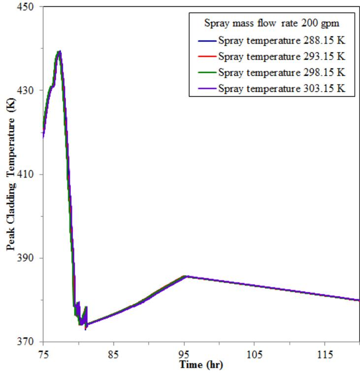
**Figure 15 The peak cladding temperature for sensitivity study of spray flow temperature (beginning to spray while pool level reached 2/3 fuel height)**
