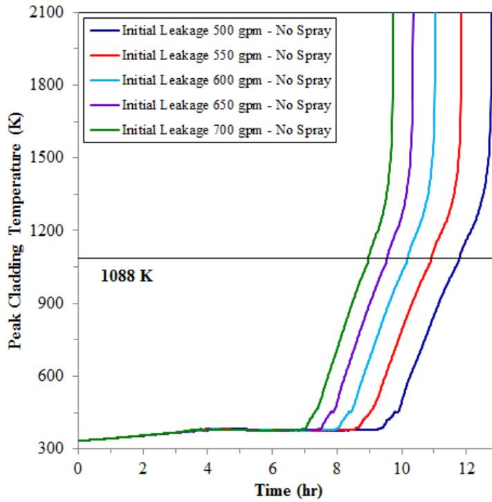
Figure 17 The peak cladding temperature for different leakage rates without spray
