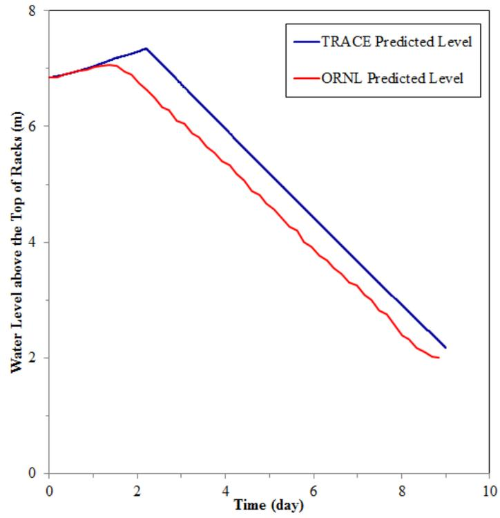
**Figure 4 The water level of SFP4**
