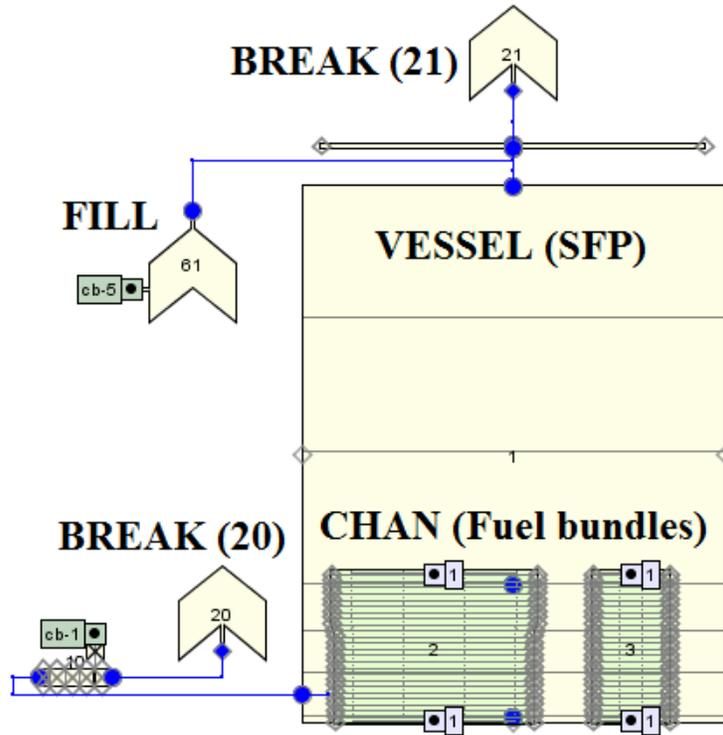
Figure 2 Chinshan NPP spent fuel pool two-channel TRACE model
