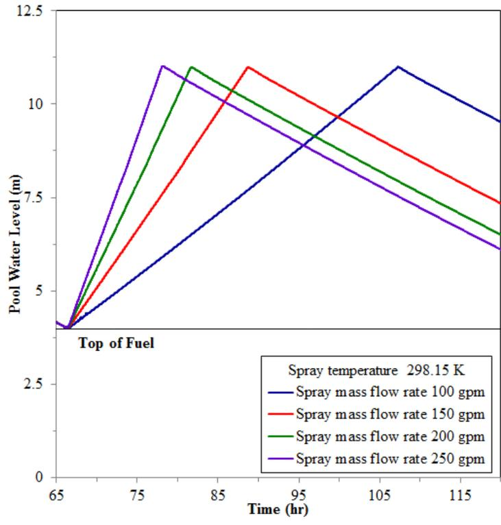
**Figure 8 The water level of the SFP for sensitivity study of spray flow rate (beginning to spray while pool level reached top of fuel)**
