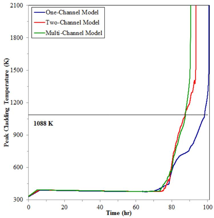
Figure 24 The peak cladding temperature for three models
