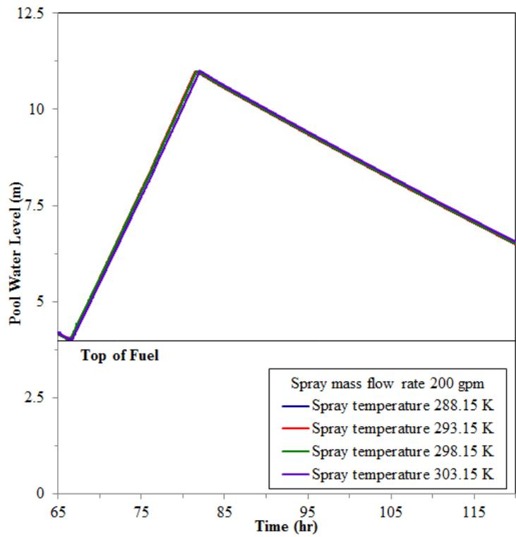
**Figure 12 The water level of the SFP for sensitivity study of spray flow temperature (beginning to spray while pool level reached top of fuel)**
