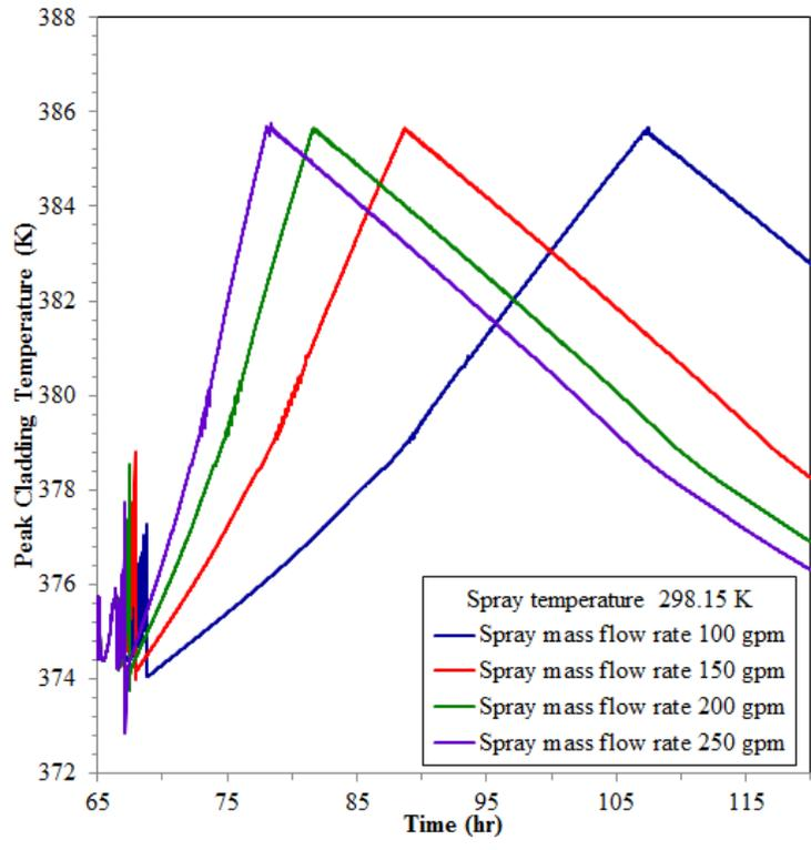
**Figure 9 The peak cladding temperature for sensitivity study of spray flow rate (beginning to spray while pool level reached top of fuel)**
