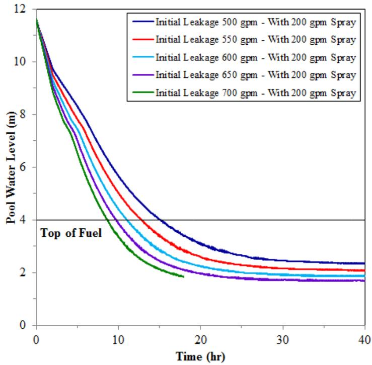
Figure 18 The water level for different leakage rates with spray
