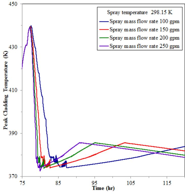
**Figure 11** The peak cladding temperature for sensitivity study of spray flow rate (beginning to spray while pool level reached 2/3 fuel height)
