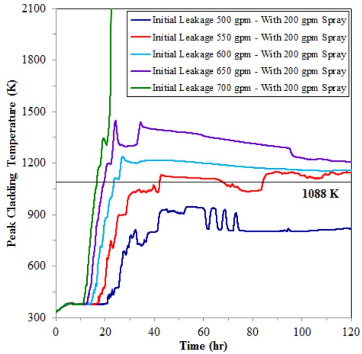
Figure 20 The peak cladding temperature for different leakage rates with spray
