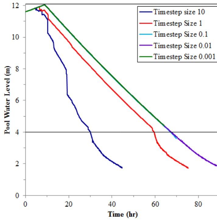
Figure 21 The pool water level for different timestep sizes
