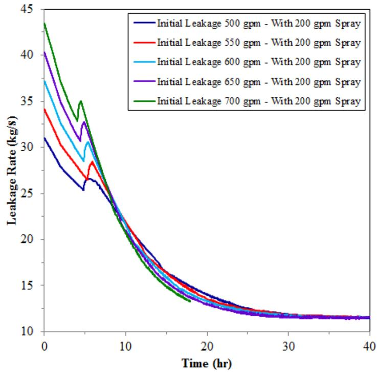
Figure 19 The changes of different leakage flow rates with spray
