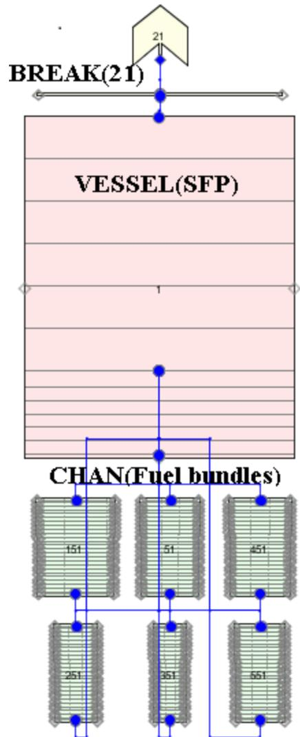
Figure 3 Chinshan NPP spent fuel pool multi-channel TRACE model
