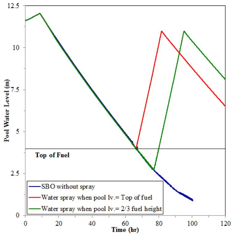
**Figure 6** The water level of the SFP for sensitivity study of spray system initiation time
