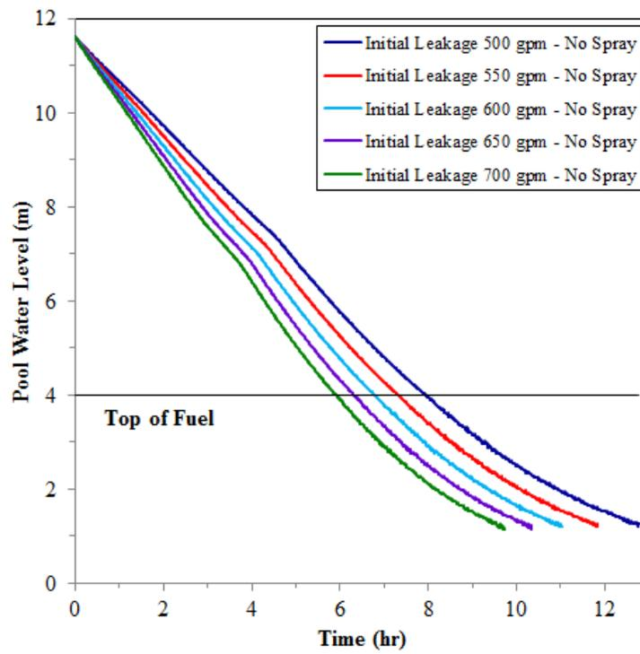
Figure 16 The water level for different leakage rates without spray
