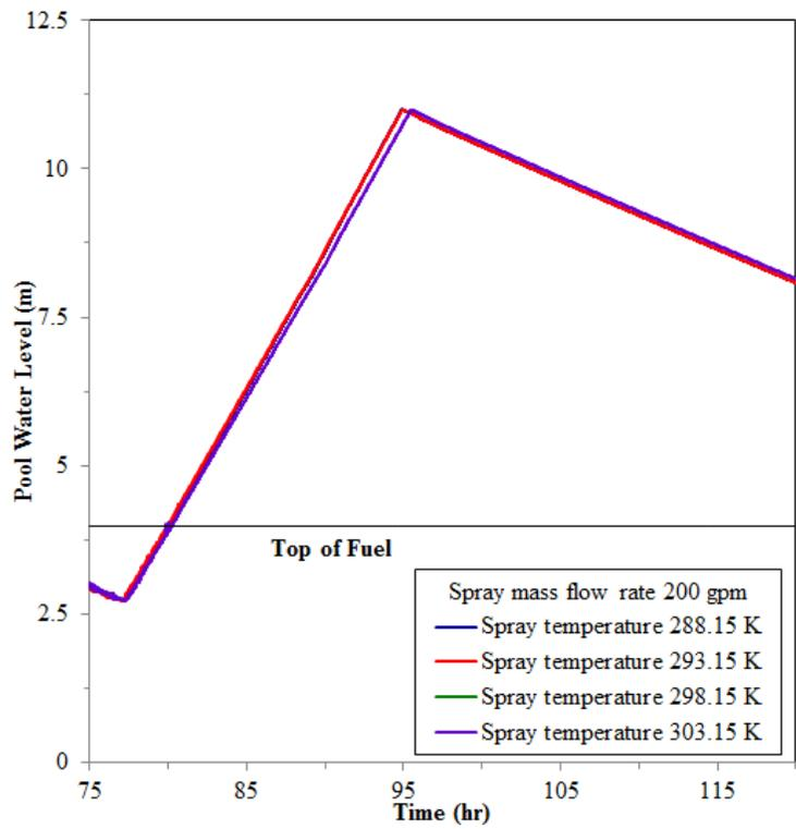
**Figure 14 The water level of the SFP for sensitivity study of spray flow temperature (beginning to spray while pool level reached 2/3 fuel height)**
