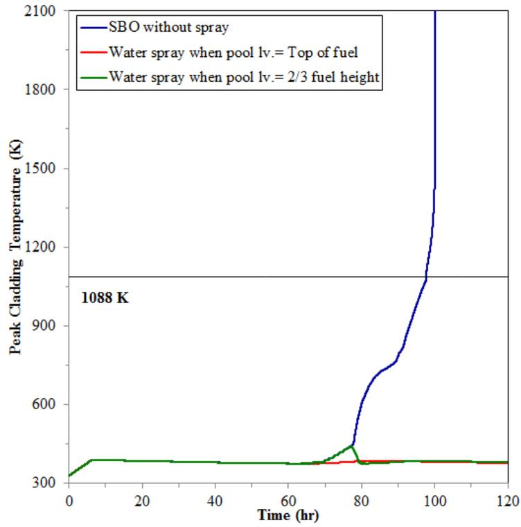
**Figure 7 The peak cladding temperature for sensitivity study of spray system initiation time**
