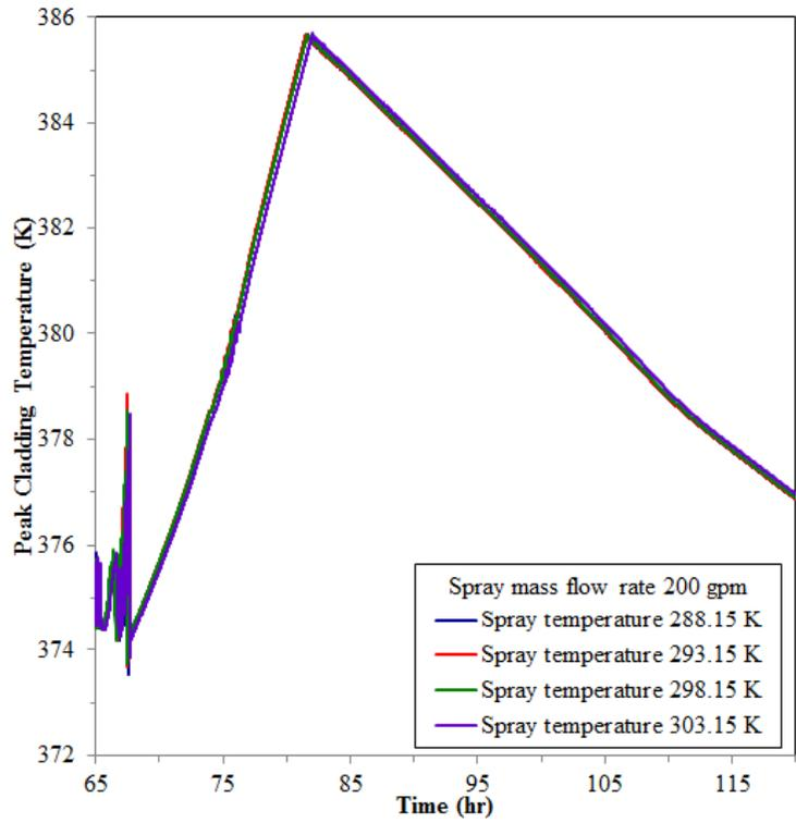
**Figure 13 The peak cladding temperature for sensitivity study of spray flow temperature (beginning to spray while pool level reached top of fuel)**
