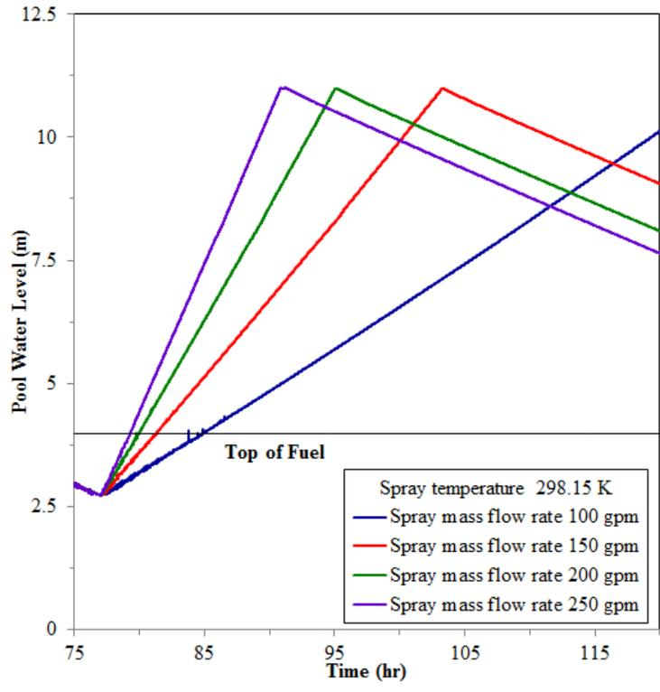
**Figure 10** The water level of the SFP for sensitivity study of spray flow rate (beginning to spray while pool level reached 2/3 fuel height)
