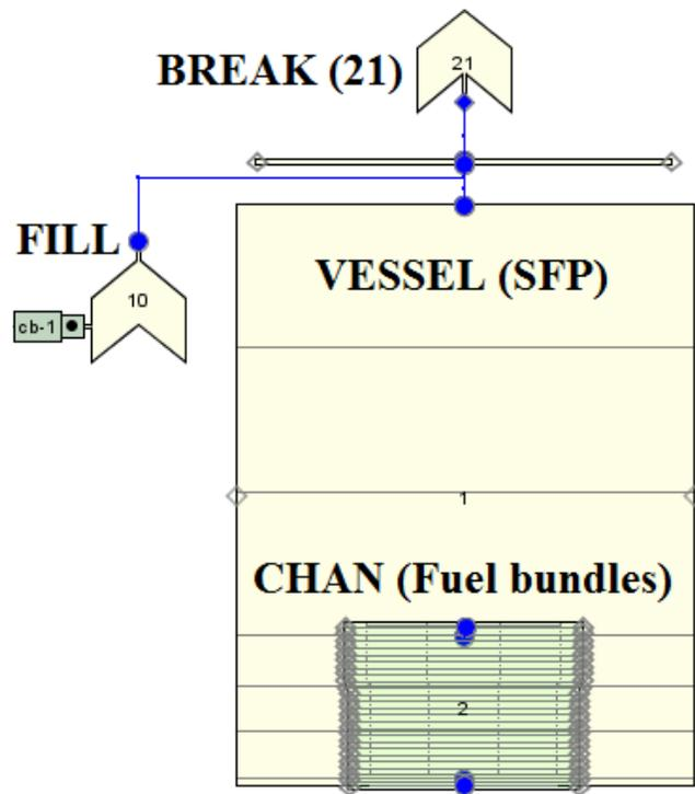
Figure 1 Chinshan NPP spent fuel pool one-channel TRACE model
