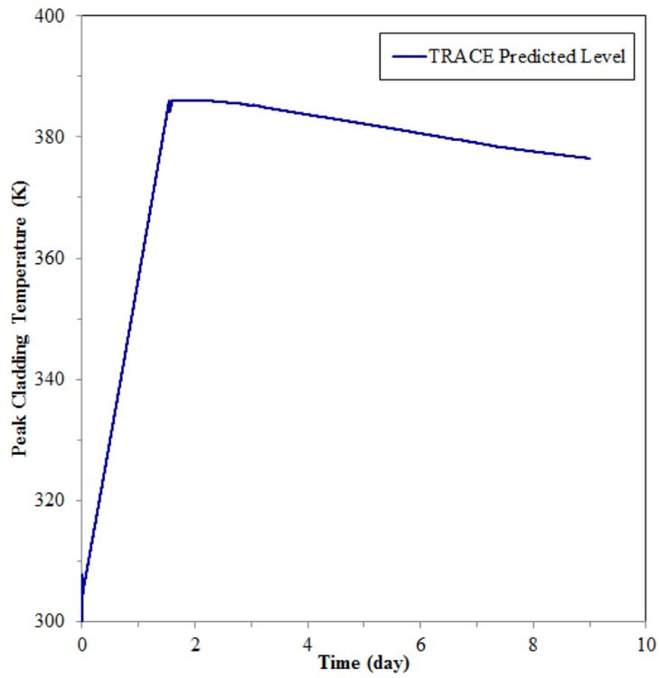
**Figure 5 The peak cladding temperature of SFP4**
