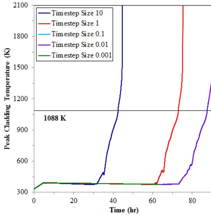
Figure 22 The peak cladding temperature for different timestep sizes
