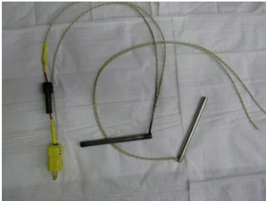
Figure 4-3. Two 300 W cartridge heaters. One has an in-line circuit breaker.
