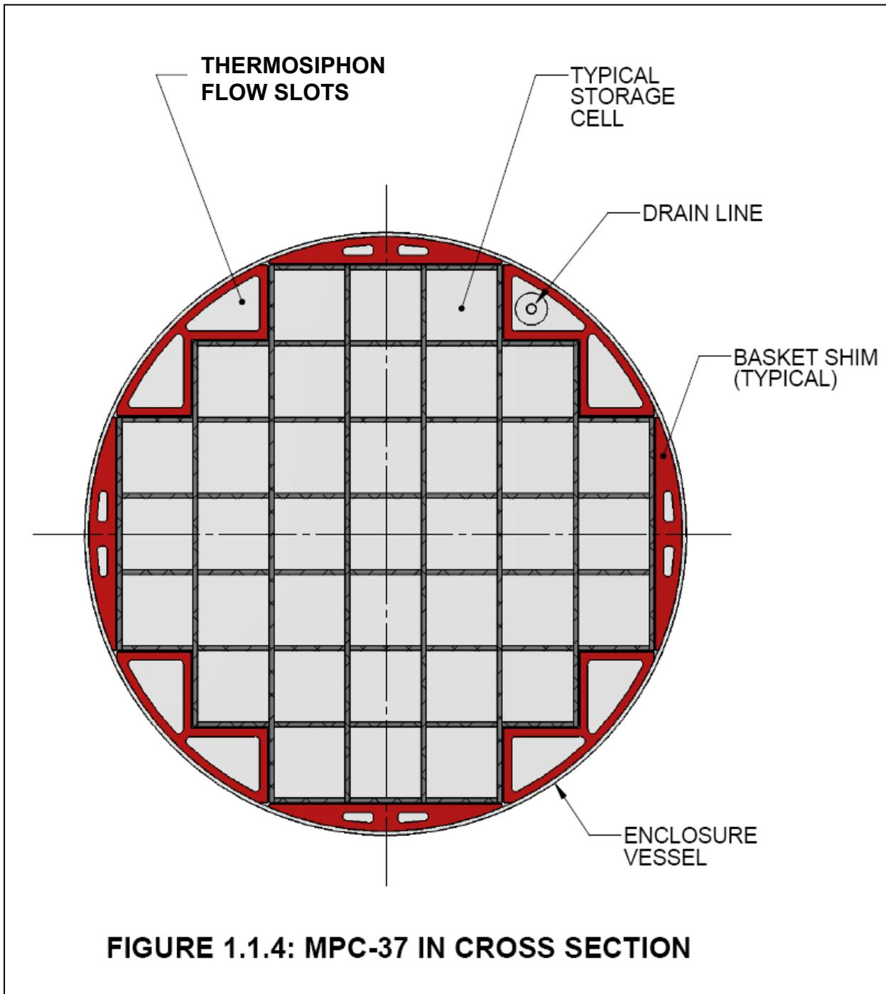
**FIGURE 1.1.4: MPC-37 IN CROSS SECTION**
