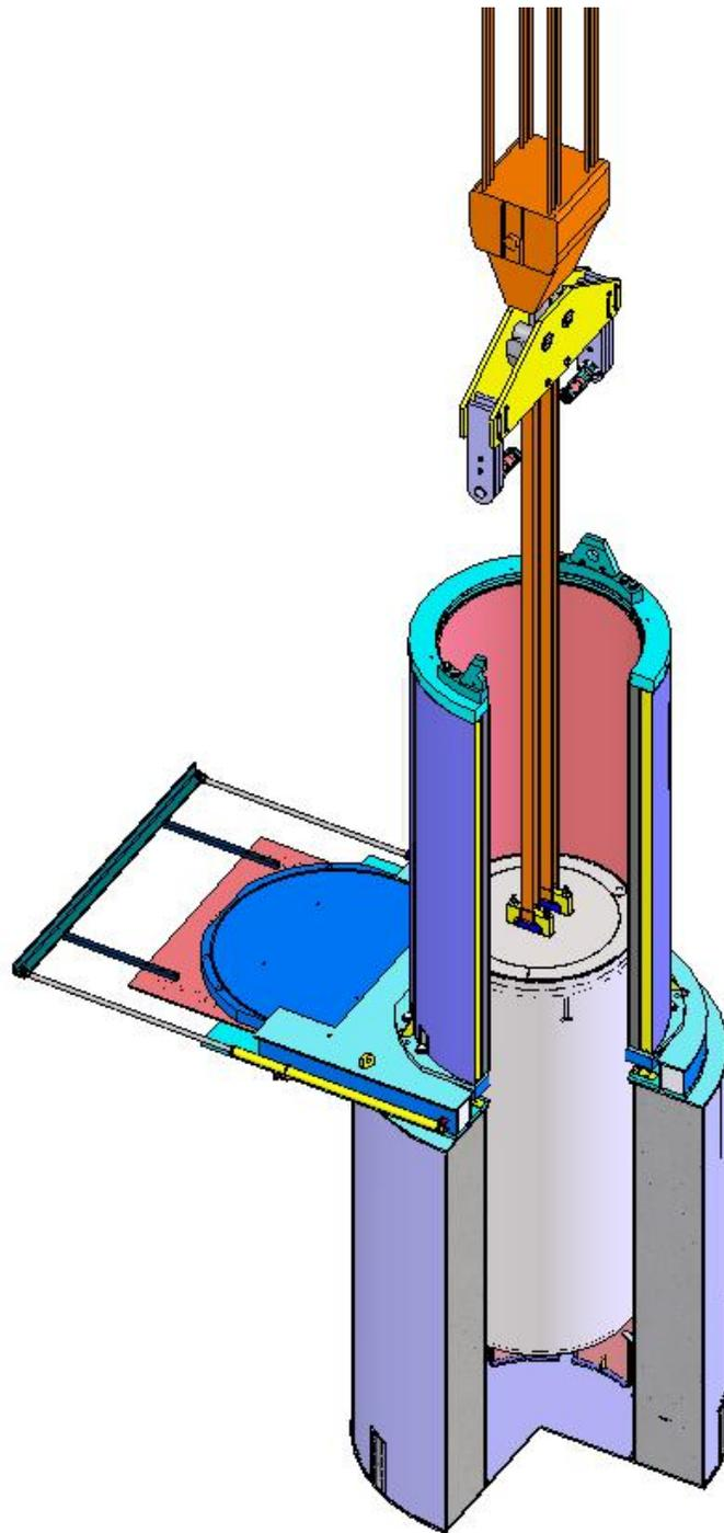
**FIGURE 1.1.3: MPC TRANSFER IN THE PLANT'S EGRESS BAY**
