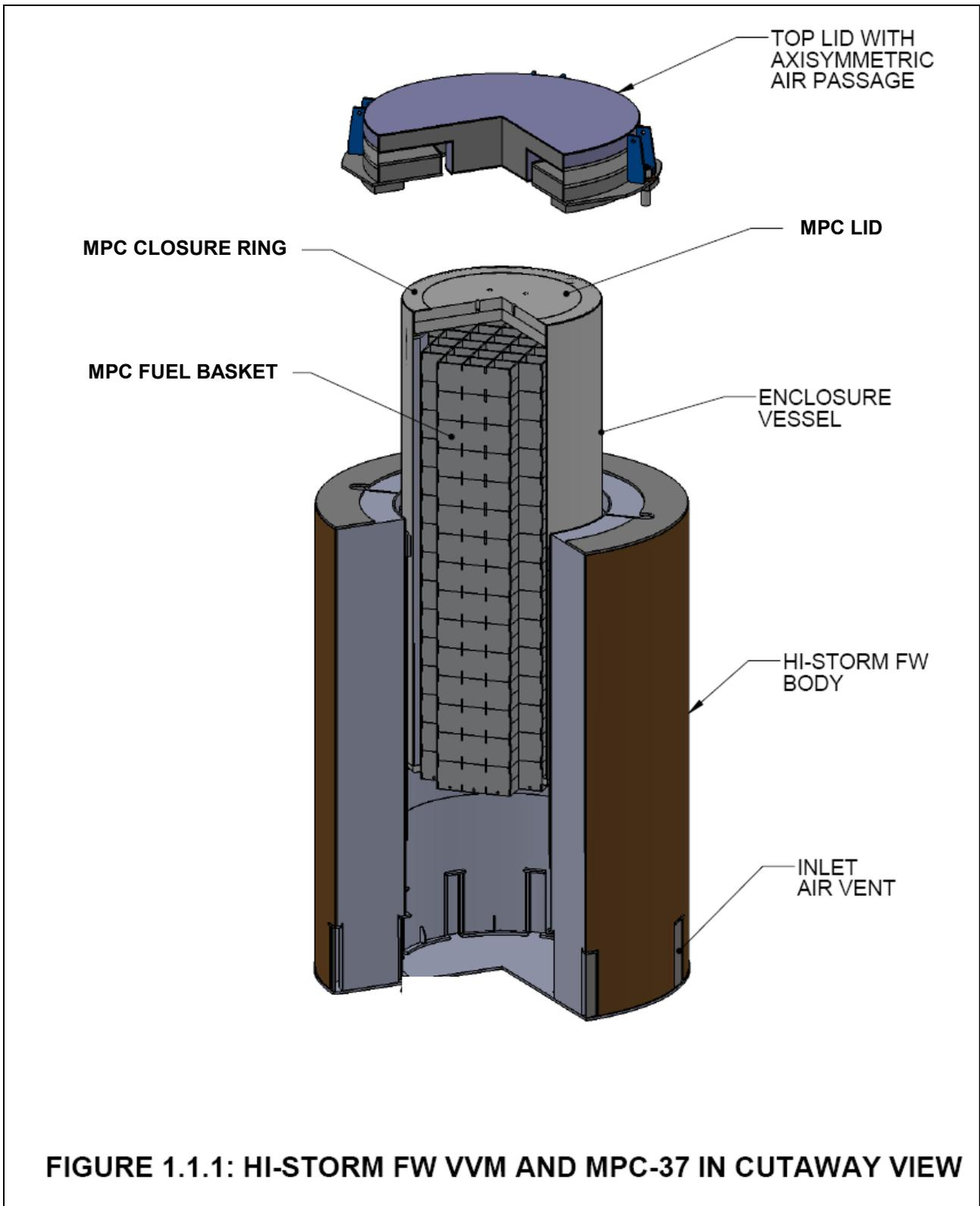
**FIGURE 1.1.1: HI-STORM FW VVM AND MPC-37 IN CUTAWAY VIEW**
