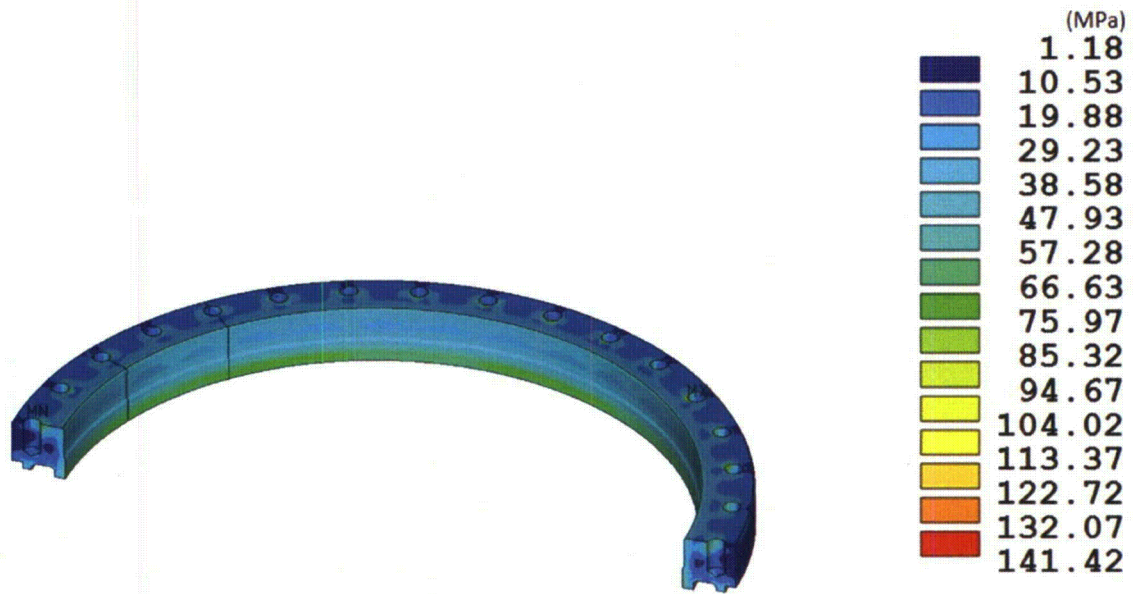
Figure 2.7.1-4 RT-100 Flange HAC End Drop Stress Intensity Results
