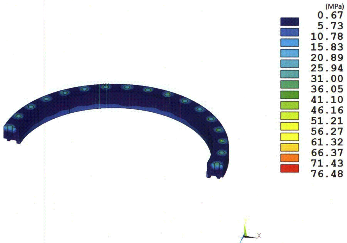
Figure 2.6.7-15 RT-100 Flange NCT End Drop Stress Intensity Results
