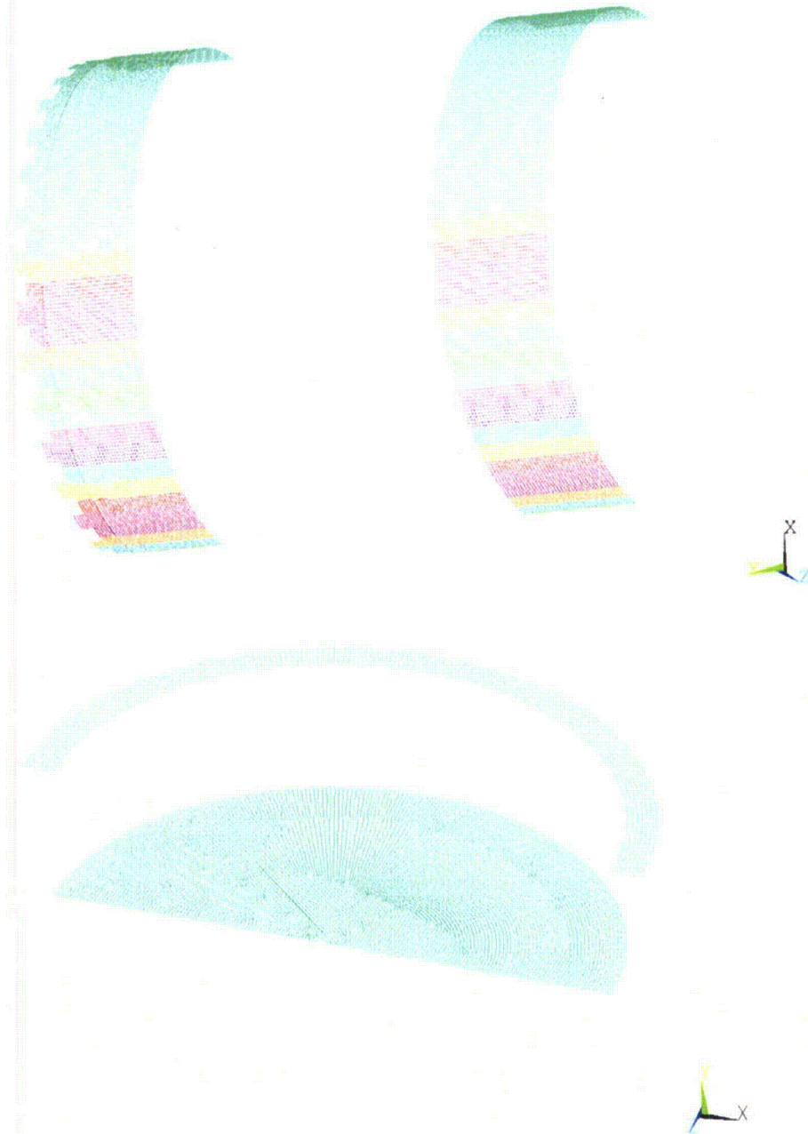
Figure 2.6.7-3 Gap Elements Used to Represent the Impact Limiters for Side and End Drop Configurations
