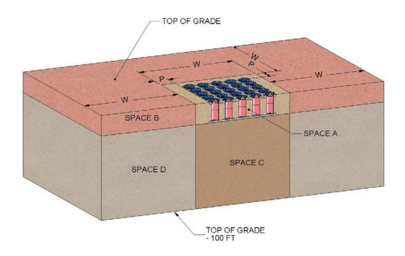
Figure 3-1 - SUBGRADE AND UNDERGRADE SPACE NOMENCLATURE
